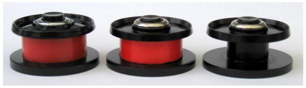
On both pictures above, to the left: an original plastic Cardinal 44/4 spool with red arbor ring; middle and right: two aluminium replacement spools, one with an original arbor ring slightly cut to size.
