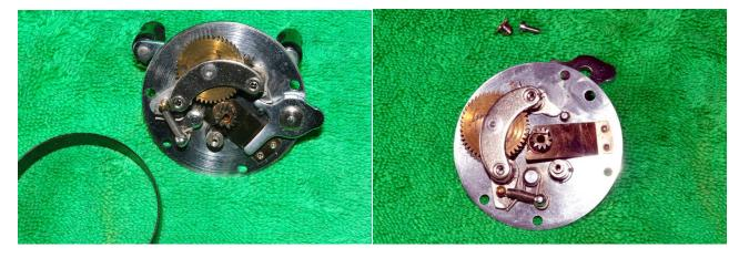
The free spool button/lever is held in place with a screw and nut. Hold the nut whilst loosening the screw from the other side of the side plate.
