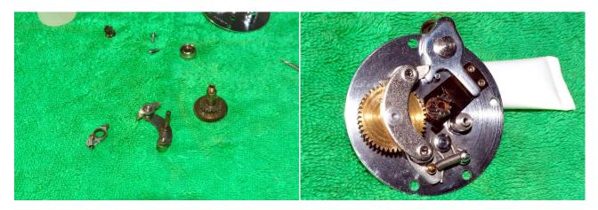
Give everything a thorough clean and then reassemble. Use light oil on the gear shaft and a light coat of grease on all other metal to metal friction surfaces. Ensure that the teeth on the main and pinion gear have a coating of grease. Remember to use a light coat of grease on all screw threads.
