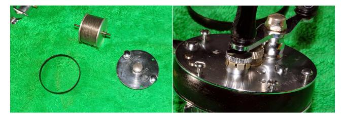
Loosen the two thumb screws holding on the left side plate-the left side plate, plate spacer and the spool can then be removed. Remove the spool cap-there's a felt washer in it that needs to be cleaned (use lighter fuel or Shellite). When it's clean add a drop of oil to the felt and a light coat of grease to the threads and replace.
