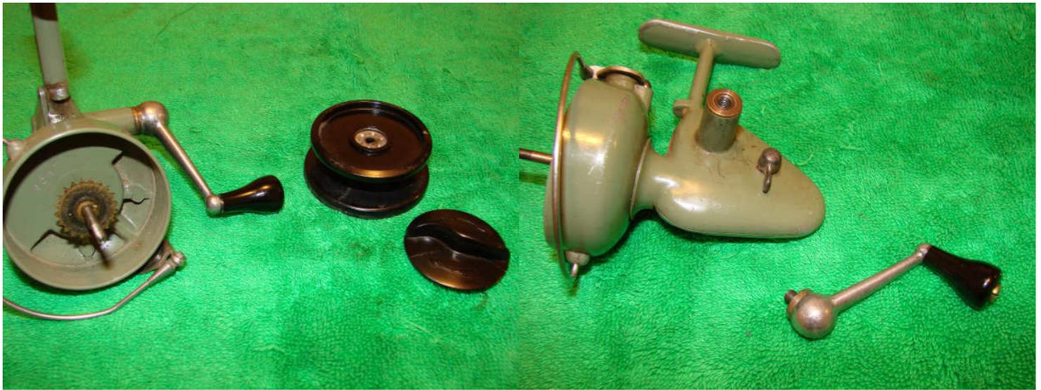
Remove the spool and unscrew the handle by turning backwards.
