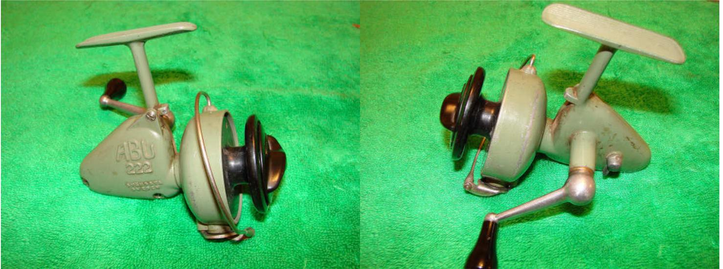
This reel seems to be working fine and just needs a quick service. The drag knob was broken but this can be easily repaired with some glue.
