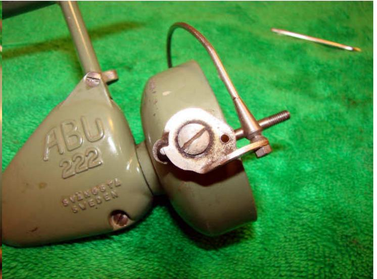
Replace the main shaft and arm. Note the screw in the housing for the pinion gear-remove this and add a couple of drops of oil. Replace the side cover and the three screws holding it in place. Remove the screw holding on the bail arm and apply a light coat of grease to the bail spring. Add a drop of oil to the bail trip mechanism (it sits below the bail spring).
