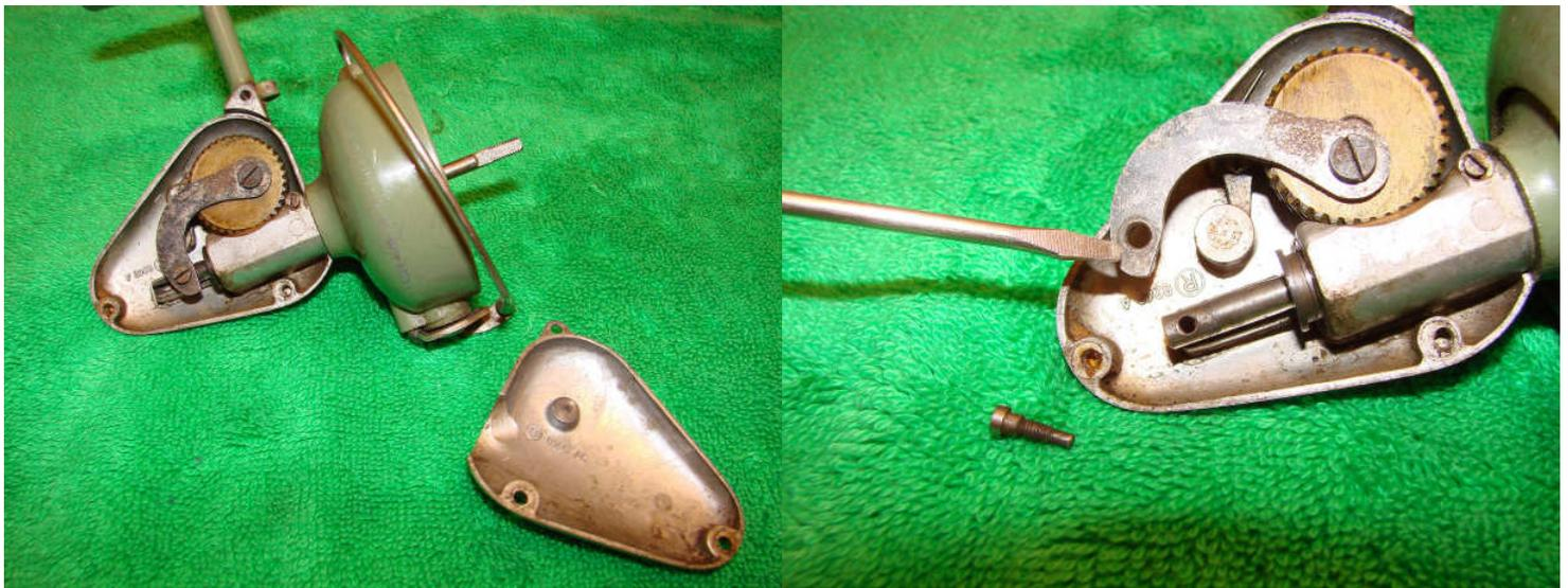
Remove the three screws holding on the side cover and remove the side cover. Remove the screw attaching the arm to the end of the main shaft.
