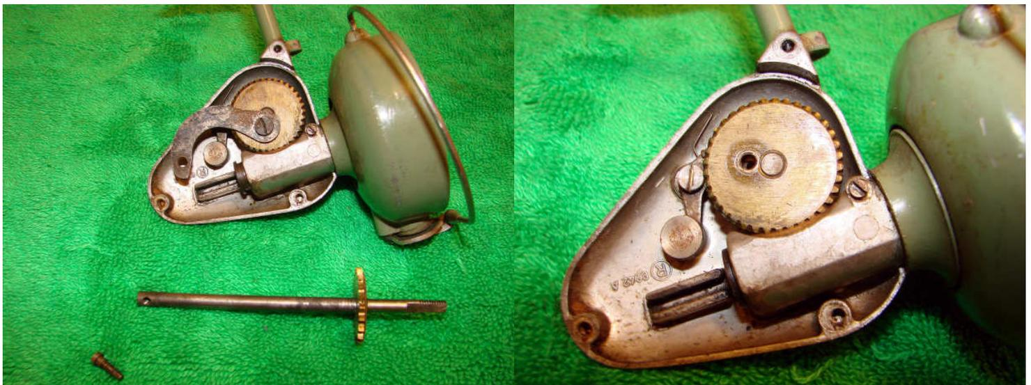
Remove the shaft and then remove the screw attaching the arm to the main gear. Remove the arm.
