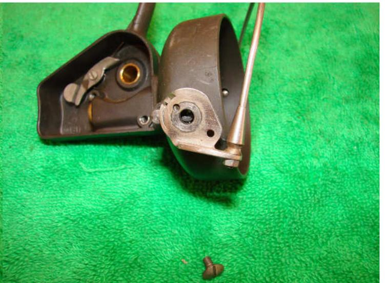
The main gear lifts out of the body. Remove the screw holding on the bail arm.
