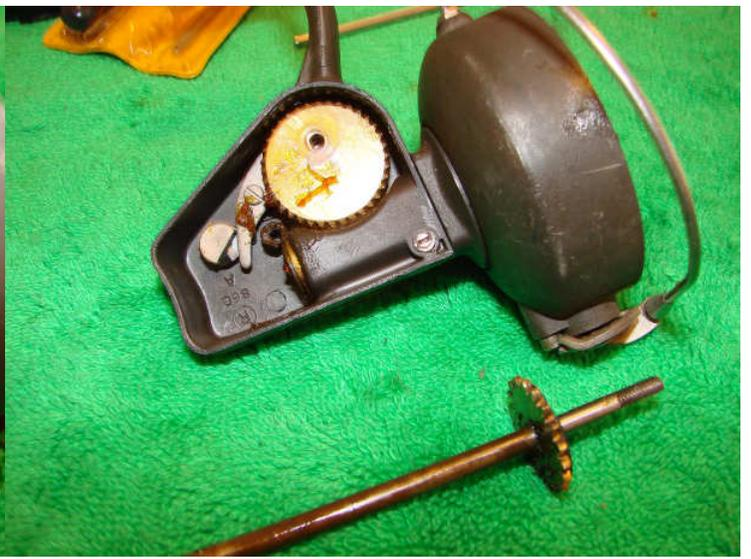
Remove the screws that connect the arm to the main gear and the end of the main shaft. Remove the main shaft and the arm.
