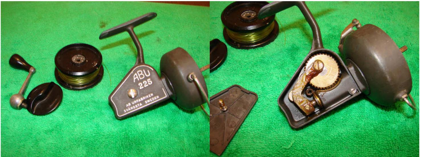
Remove the drag knob and spool, and then remove the handle by winding it backwards. The side cover is held in place by just one screw.
