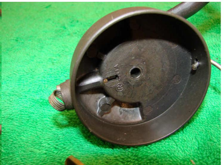
Fortunately the bail spring is not broken-it just needs a clean. Remove the bail spring and clean it and then give a light coat of grease. Lubricate the bail trip lever with a drop of oil where it
