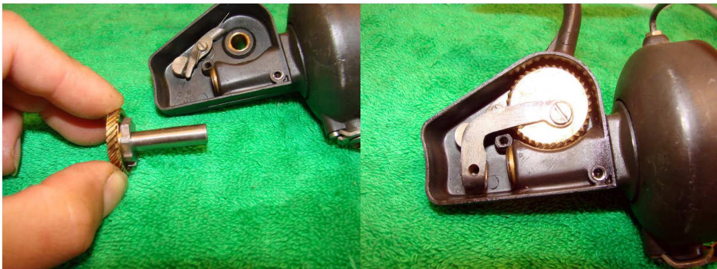
Clean the shaft of the main gear and give it a light coating of oil. Grease the teeth on the main gear with a coating of light grease and replace the gear in the reel body. Add a light coating of grease to the surface of the main gear and then replace the arm.
