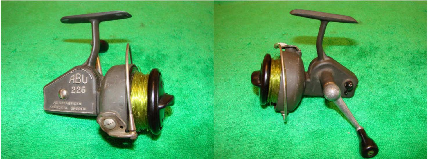
This reel is simple to service and shouldn't take long to do. Overall this reel is in very nice condition though the bail arm felt a bit loose and wasn't closing properly-probably due to a dirty or worn bail spring. When cranking the reel felt a bit 'gummed up'-this was probably due to the original oil and grease drying out-nothing a quick service won't fix.
