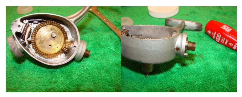
Coat the teeth and the upper surface of the gear with a light grease. Place a few drop of oil in the pinion bushing and then replace the pinion gear in the housing. Note the screw in the reel body that holds the pinion gear in place.
