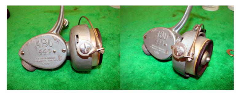
This reel seemed to working fine with the exception of the line lay. The spool did not move in and out fully when cranking the handle-at certain points the spool would 'hang up' and stick in one position. It is a display reel but it is still nice to have display reels that are fully functioning and can be fished.
