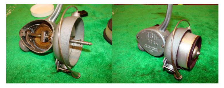
Replace the rotor cup and the rotor cup locking nut. Replace the body cover and fix in place with the two screws. Replace the spool and handle. The spool oscillation works fine now-note the perfect line lay-a lot better than many modern spinning reels!
