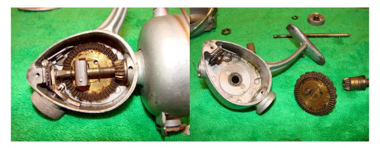
The problem with the line lay is apparent-the oscillating slider is held in place on the main shaft with two c-clips. One of the c-clips is loose and needs to be replaced.
