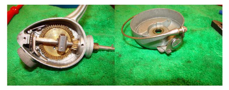
Apply a few drops of oil to the main shaft and then replace-you will need to place the oscillating slider on the stud on the main gear (note that the 'dimple' on the oscillating slider faces towards the base of the reel). When everything is in position replace the two c-clips ensuring that they are seated fully in the grooves on the main shaft.
