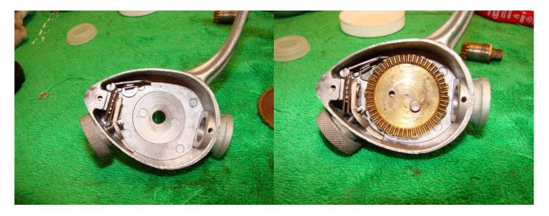
Reassemble the drag stack giving the fibre washers a light coat of drag grease. Oil the shaft on the main gear and replace it in the housing.
