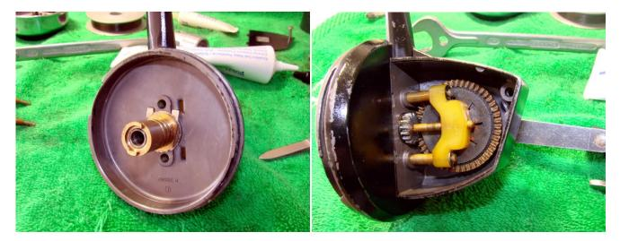
Replace the locking washer and pinion gear housing, not forgetting to oil the shaft of the pinion gear where it contacts the housing. Replace part #9675 and lubricate the pins and fix in place with the two e-clips.
