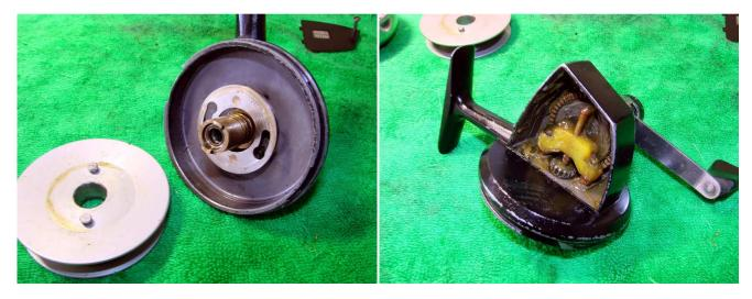
Remove the spool-it has a bayonet mount and you can see the two pins on base of the spool. It's hard to see due to all of the grease but there are two e-clips (#3909) holding on part #9675. Remove these.
