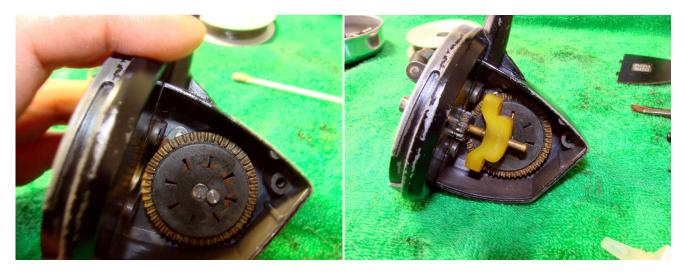
Make sure the anti reverse pawl is correctly seated on its' pin. Replace the pinion gear and plastic oscillating slider.
