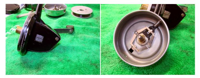
Replace the side plate and the handle assembly not forgetting to grease the thrust bearing. Replace the spool. You will probably need to tighten the drag when you replace the bell housing #9664.
