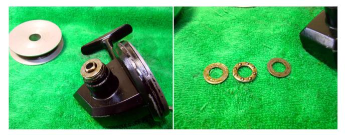
Note there is an open thrust bearing under the handle (# 9011 and #9015).
