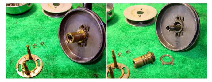
Part #9675 can be removed from the front of the reel body. Unscrew the housing for the pinion gear #9743. Note the locking washer underneath #9742-in this instance it is incorrectly fitted.
