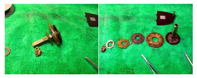
Remove the main gear assembly from the reel body. The anti reverse pawl (#5579) is still present but the copper 'ears' have been bent out of shape-simply bend them back into shape so they grip either side of part #9010-the third part from the left in the second photo.
