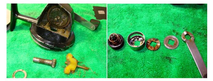
The pinion gear #9671 and the plastic part #5680 can then be removed from the reel body. Note the metal pin in the photo is housed in the plastic part #5680. It should actually be attached to the pinion gear-this is no problem as it can be fixed. Unscrew the drag knob and then remove the handle assembly.
