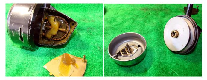
Remove the side plate-just one screw to loosen and no shortage of grease here! Remove the spool cover #9674 (it simply twists off) and unscrew the bell housing #9664. You may need to tighten the drag fully to accomplish this. There is only one pickup pin #9301 although the housing has space for two.
