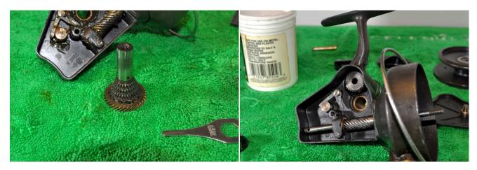
Before reassembly give everything a thorough clean. Apply a light coat of oil to the main shaft and replace in the reel body. Add oil to the friction surfaces on the pinion gear where it contacts the bushings. Add a drop of oil to the friction surfaces on the anti reverse switch. Apply a light coat of grease to the teeth of the pinion gear and the ratio selector gear.
