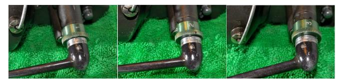
To change the gear ratio, simply pull out the green collar and turn. Each gear ratio will click and lock in place. There are three different speeds available as shown in the above photos. To oil the shaft for the selector gear put in position three-note there is a slight gap under the green collar where you can place a drop or two of oil.
