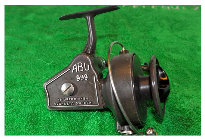
Replace the left hand side plate and tighten the side plate screw. Add a drop of oil to the bail spring screw and you're done.
