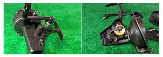
Remove the handle by winding backwards. Then remove the right side plate-it is held in place with one screw. Remove the screws that hold the oscillating arm to the main shaft and the main gear.
