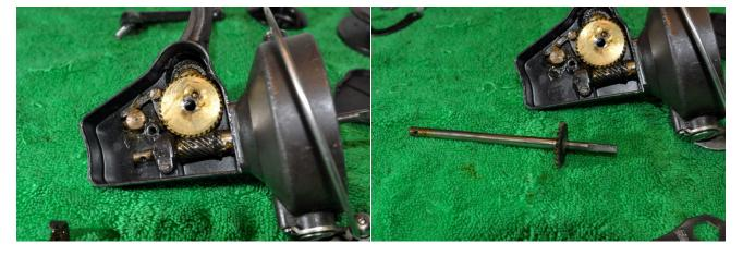
Remove the oscillating arm and the main shaft. The drag washer on the main shaft (above the click wheel) will need to be cleaned.
