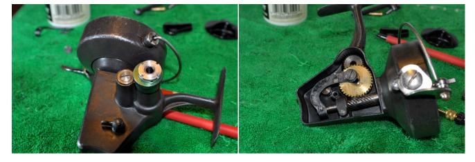
Apply grease to the teeth of the main gear and the three stainless gears behind it. Oil the shaft of the main gear and replace in the body. Fix in place with the washer and screw. Replace the oscillating arm and fix in place with the two screws (one on the main shaft and one on the main gear). Apply a light coat of grease where the oscillating arm contacts the main gear.
