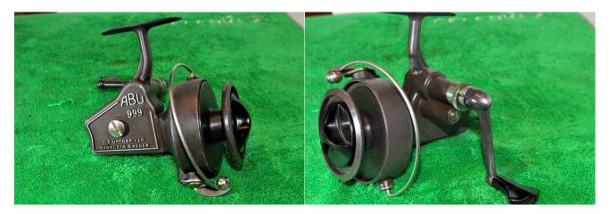
There are numerous two speed multipliers and lever drag reels around, but this is the first three speed spinning reel that I am aware of. It is a very solid old reel and even now it is quite unique in that it is a three speed-the ABU 999 must have been cutting edge technology when it first came out.
