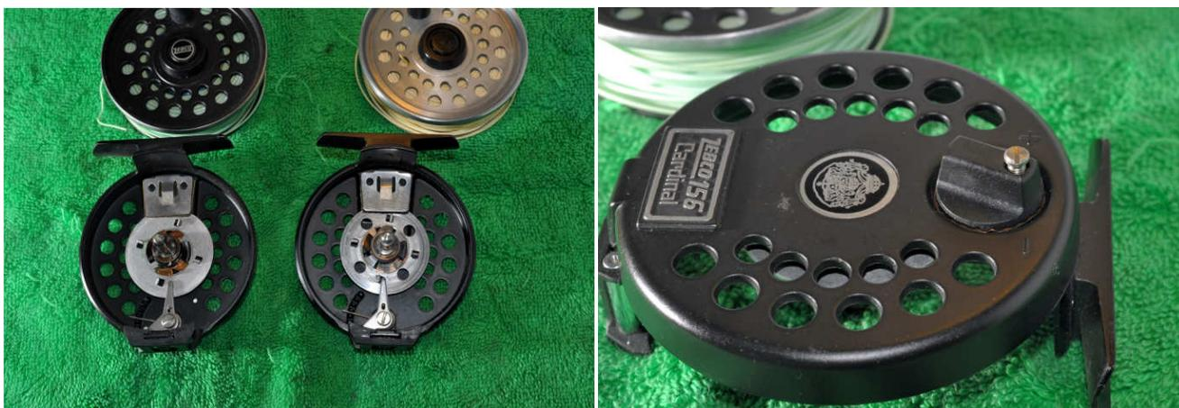
The spool is removed by simply pressing the push button in the middle and lifting it off. Internally there are no differences apart from the fact that the Zebco does not have the holes in the drag plate. In addition in the Zebco you can see the studs used to fix on the name plate. Servicing is the same for both reels. Undo the screw for the drag knob and remove it.
