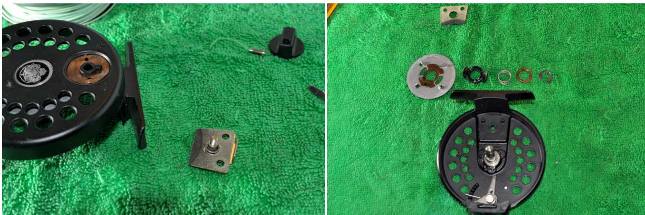
Note the copper washer under the drag knob. The outer cork drag plate will fall out from the other side-note the spring. Remove the c-clip on the spool shaft and remove the components. They are laid out left to right=top to bottom; drag disc, plastic cam, spring, copper washer and c-clip. The other cork drag plate at the top of the photo sits under the metal drag disc-it is the last part to be removed from the reel body.
