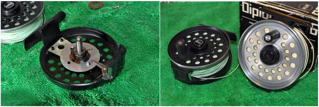
Give everything a thorough clean before reassembly. The cork drag plates can be lightly greased with drag grease. Use light oil on the other friction surfaces including the spool clicker. The spool clicker will need to be pushed out of the way before the metal drag disc can be replaced.
