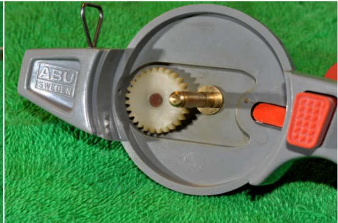
The anti reverse mechanism simply lifts out. Check that the spring is in good order-give a light coating of grease and then replace. Give everything a thorough clean and then reassemble. Add some oil to the shaft of the main gear and then replace in the body. Fix in place with the c-clip and then replace the handle and handle nut.
