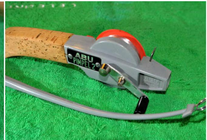
Add some grease to the teeth on the main gear and some oil to the spool shaft. Replace the spool on the body and you're finished-very quick and simple!
