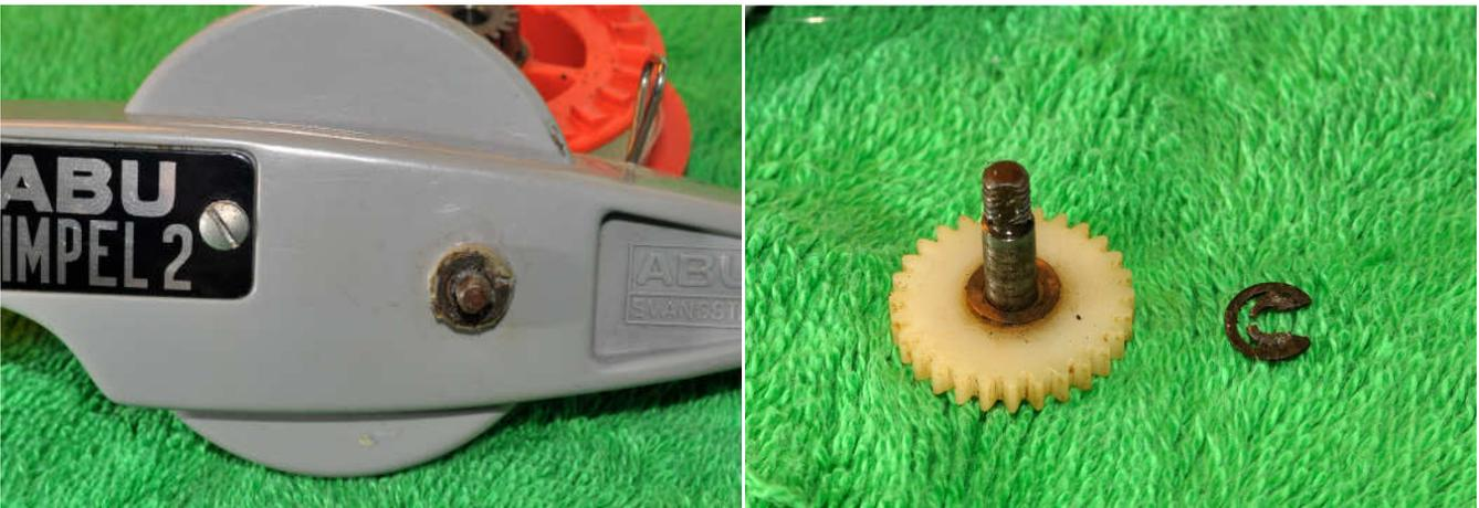
Remove the handle nut and handle. There is a c-clip on the shaft for the main gear holding it in the body. Remove this and the main gear can be removed from the other side. Note the copper washer on top of the main gear.
