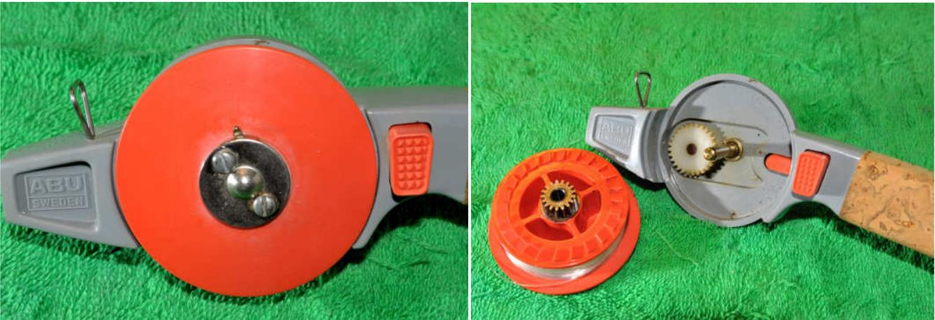
A lever on the spool allows it to be removed—simply push the lever to one side and the spool lifts off. The pinion gear is fixed to the bottom of the spool and is brass, note that the main gear is plastic.
