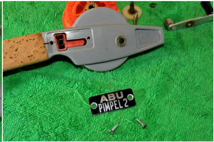
To access the anti reverse mechanism remove the two screws on the metal plate and then remove the plate.
