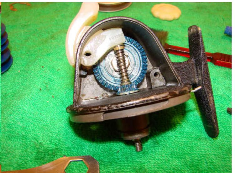
When everything is spotless apply grease to the gears. A toothbrush is good for ensuring coverage to the base of the teeth. Apply some light grease to the friction surfaces on the thumb button. Add a light coating of oil on the throw out pin and spring.
