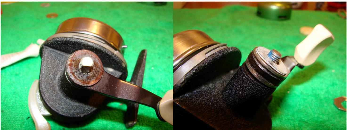
Then add a fibre washer/handle/fibre washer, flat metal washer, curved metal washer.
