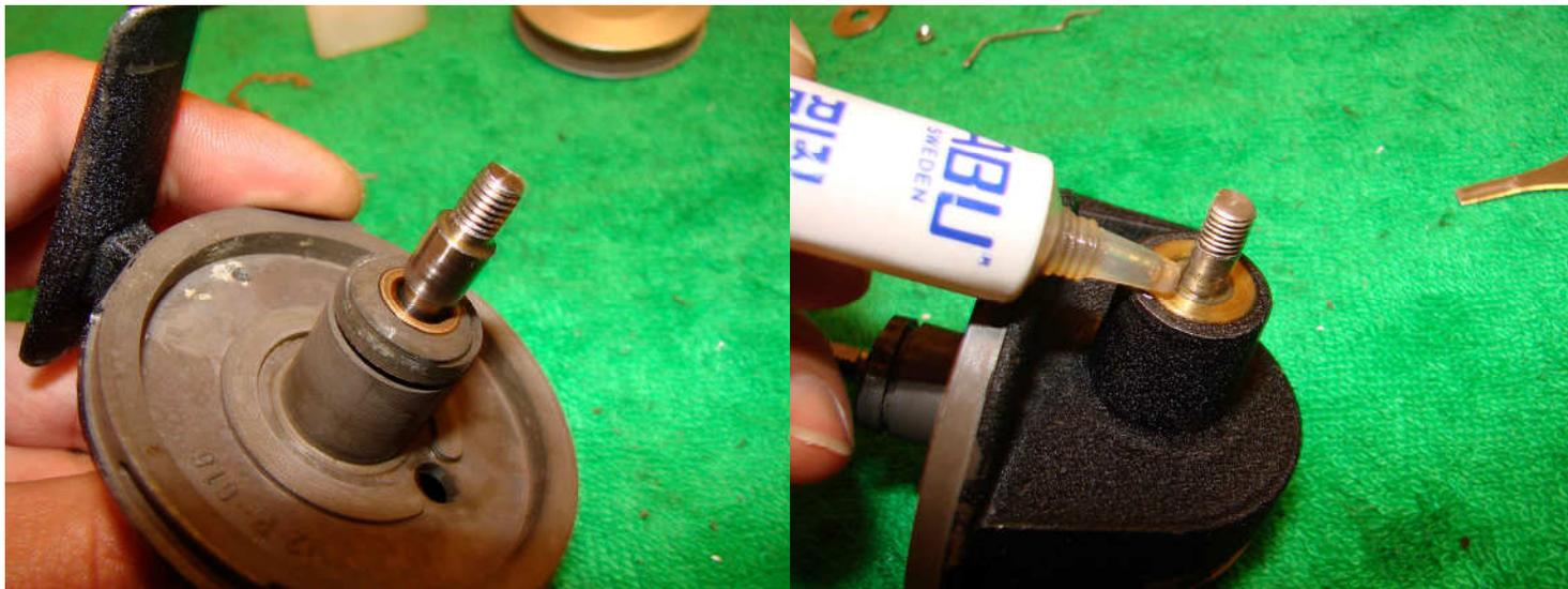
Push in the throw out spring with your finger and then turn the reel over. Apply oil to the gap between the winding cup shaft and the reel body. Wipe off any excess. Apply oil to the drive shaft/drive shaft bushing and let it penetrate. Wipe off excess.
