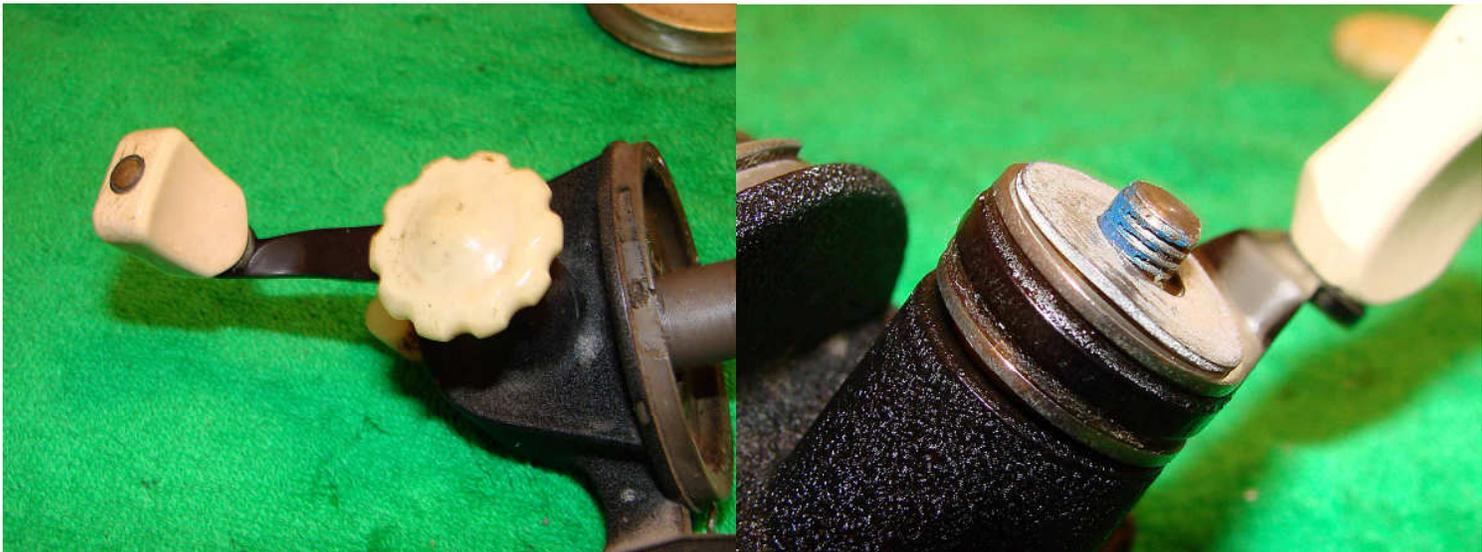
Unscrew the drag knob and remove the handle. Note the orientation of the washers. From the top, drag knob, curved metal washer, flat metal washer, fiber washer, handle, fiber washer, flat metal washer.
