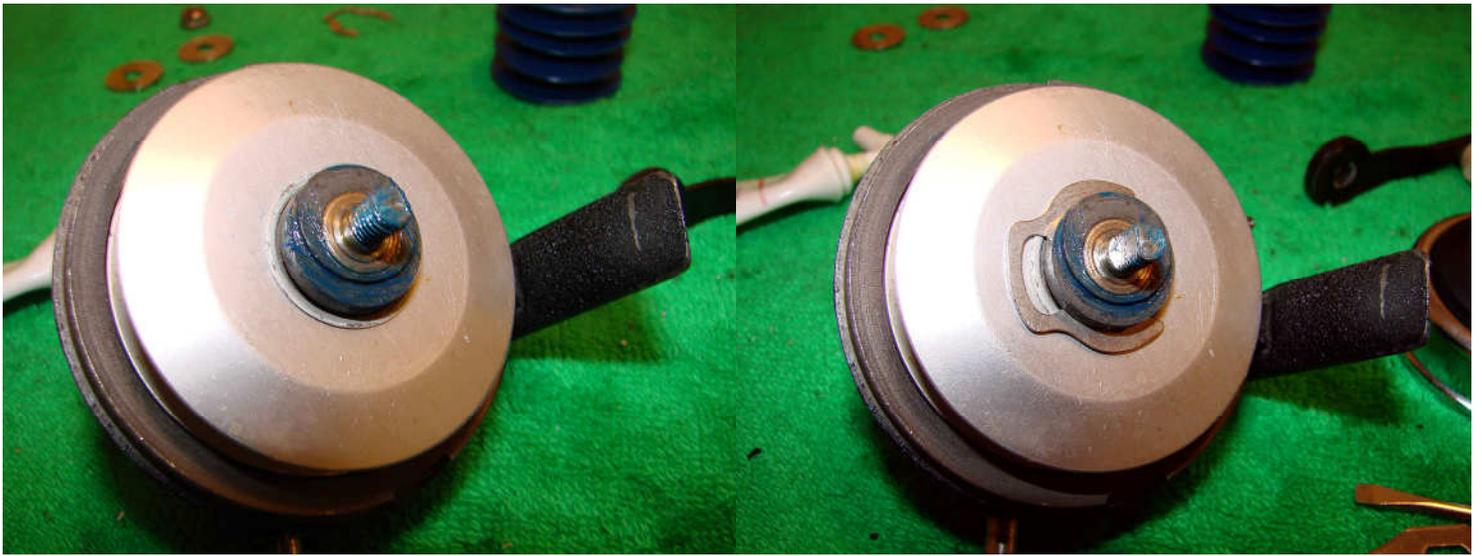
Reattach the spool and add a light coating of grease where the line pick up ejector contacts the body (don't forget to add a light coating of oil/grease to the friction surfaces on the ejector on the underside of the winding cup). Replace the circlip.
