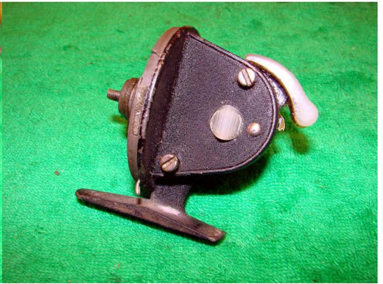
Remove the two screws holding on the side plate.
