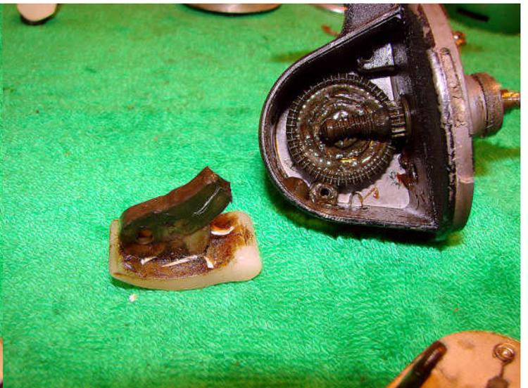
Oh dear-looks like the reel is filled with tar. No wonder it felt sluggish. The thumb button simply pulls out; it pivots on one of the side plate screws. Give everything a thorough clean. I prefer not to use solvents on plastic but this means *a lot* of scrubbing with washing up liquid and warm water.
