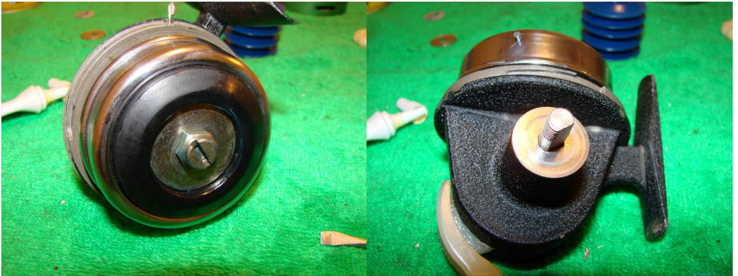
Reattach the winding cup and nut. Attach the flat metal washer to the drive/handle shaft.
