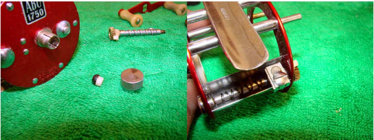
And remove the spool bearing. Remove the level wind assembly from the frame by undoing the line carriage screw and removing the pawl. The worm gear can then be removed from the line carriage.
