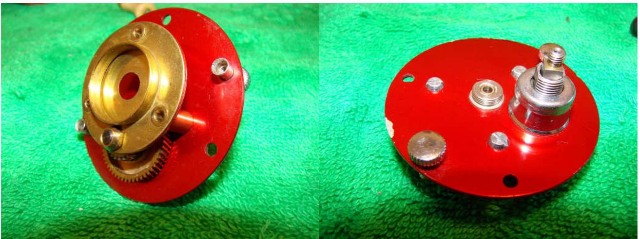
Replace the bridge gear unit on the side plate and fix in place with the three bridge screws. Replace the dust shield.
