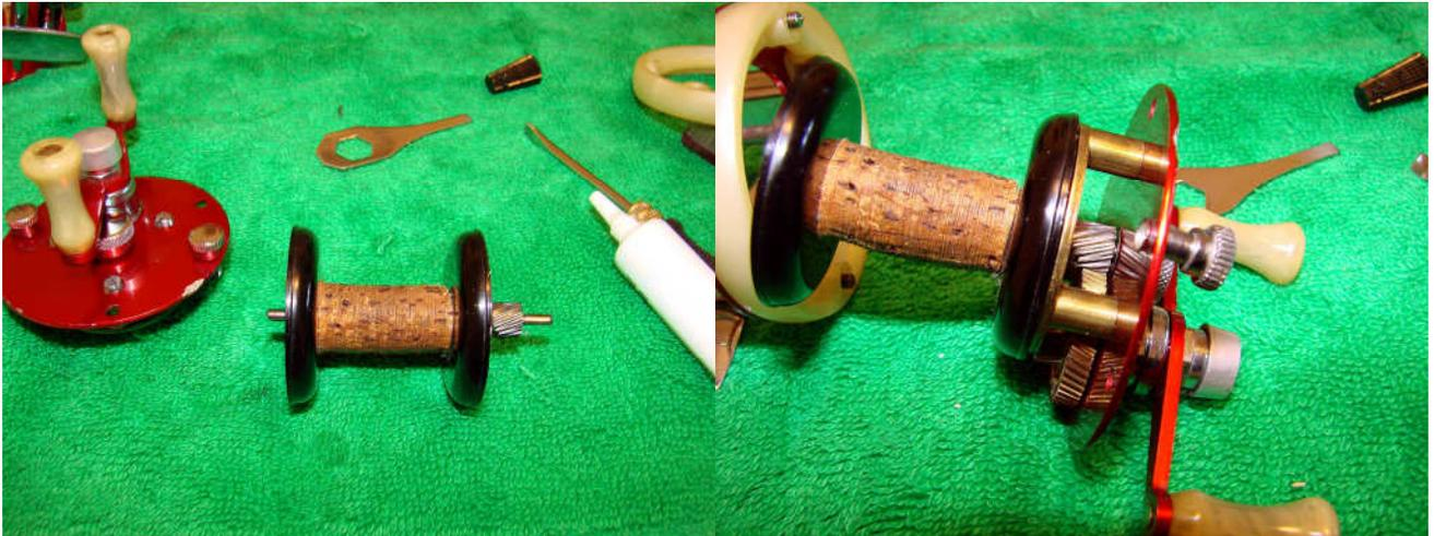
Add a drop of oil to both ends of the spool shaft and then replace the spool in the right side plate. The spool and side plate can then be replaced in the frame. Tighten the two thumb nuts.
