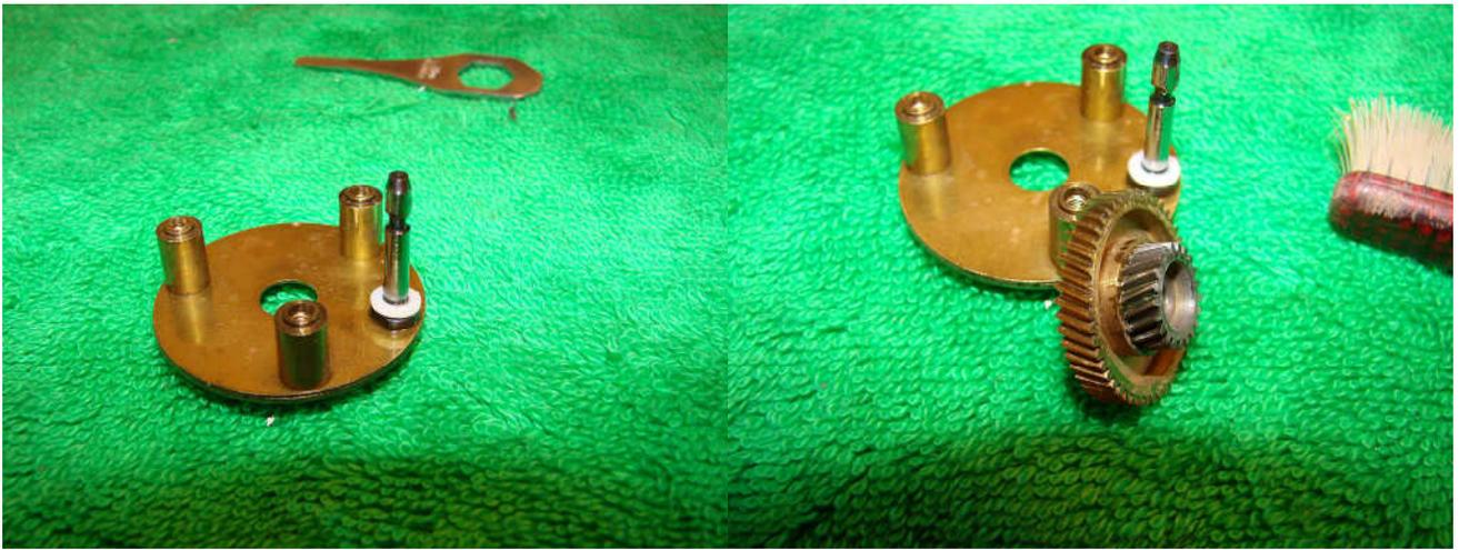
Add a drop of oil to the drive shaft and replace the drive shaft bearing (plastic washer). At this stage it is easier to add grease to the teeth on the main gear. I have used a light liquid grease.
