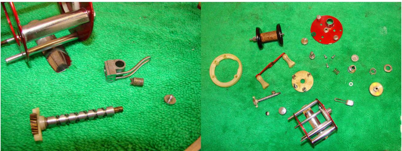
Worm gear (foreground), line carriage next to pawl and line carriage screw to the right of the photo. Everything is now ready for a thorough clean before reassembly. I prefer not to use harsh cleaners on older reels. A clean using warm water and washing up liquid followed by a thorough rinse should be sufficient.
