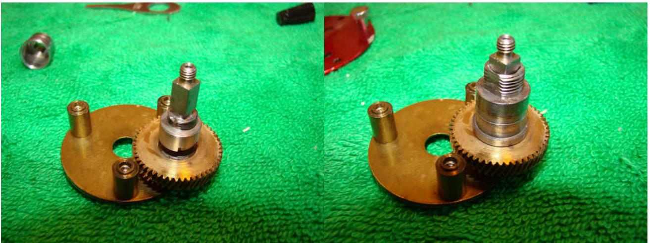
Replace the main gear on the drive shaft followed by the lock pin retainer and the handle bearing. Lubricate the handle bearing with liquid grease or heavy oil.
