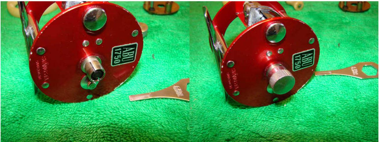
Add a drop of oil to the spool bearing and replace in the left side plate. Replace the left spool cap.
