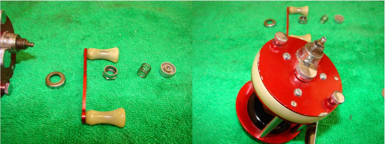
Remove the dust shield. Everything is laid out in sequence. Unscrew the two thumbnuts on the right plate.
