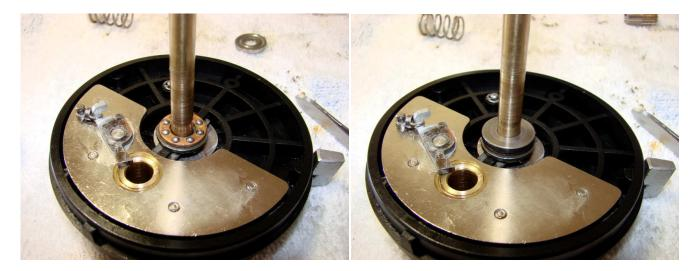
Replace the thrust bearing and pack it with grease-make sure the parts are replaced in the correct sequence.
