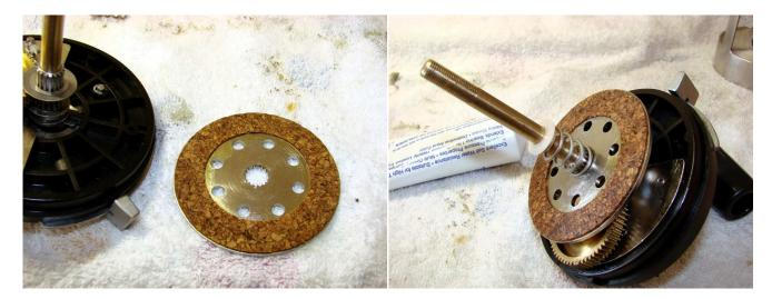
Clean the cork drag thoroughly (and the disc brake on the spool) and then apply a light coating of drag grease to the cork. Replace it on the main shaft and then replace the spring #10054 and plastic washer #10055. Reattach the handle assembly.
