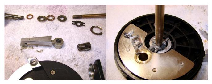
Remove the drag lever and give all parts a thorough clean before reassembly. Lubricate the anti reverse dog and spring with grease. Replace the drag lever, the main shaft, the washer, and part #10048. Use a light coating of grease.
