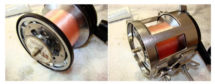
Replace the spool on the main shaft and fix in place with the gear wheel #10065. Follow the instructions on the gear wheel for setting the drag. Slide this whole assembly back into the frame. In this instance I cleaned the spool bearings and repacked them with grease
