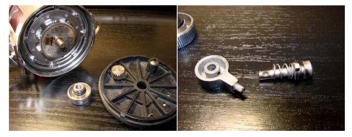
The left side plate can be removed from the frame. Undo screw #10067-the clicker knob (#10084) simply lifts off and parts #10078, #10079, #10074 can be removed from the inside of the side plate. Clean off all salt deposits before lightly greasing the assembly and replacing in the side plate.
