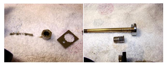
Spring, grease nipple, handle nut and lock plate laid out. Remove the shaft (#10013) from the right side of the right side plate. The pinion gear #10052 slides off the shaft.
