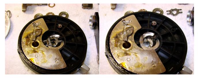
Remove part #10048 and the washer underneath-note that the washer has been slightly mangled-at some stage the reel must have been disassembled and the washer replaced incorrectly-nothing serious as the washer can be straightened out.
