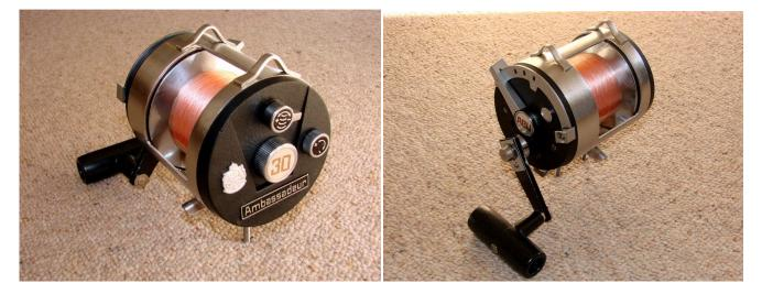
Reattach the left side plate and fix in place with knob #10089. All done and simple enough to be done by anyone!
