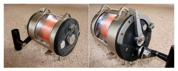
This must be one of the easiest reels to service-a brilliant design enables you to strip it down to grease the gears/service the bearings and drag without needing any tools at all. I was surprised with how few parts there were on this reel-an uncomplicated design means less things that can go wrong.
