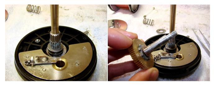
Grease the pinion gear teeth (and the bore) and replace on the main shaft. Replace the copper shim on the main gear and grease the gear shaft, gear teeth, and where the anti reverse dog contacts.
