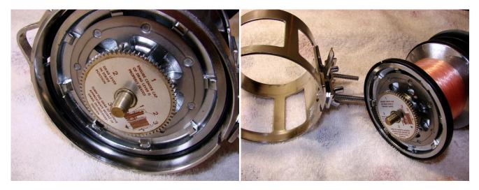
Remove the entire right side plate assembly and spool from the frame.
