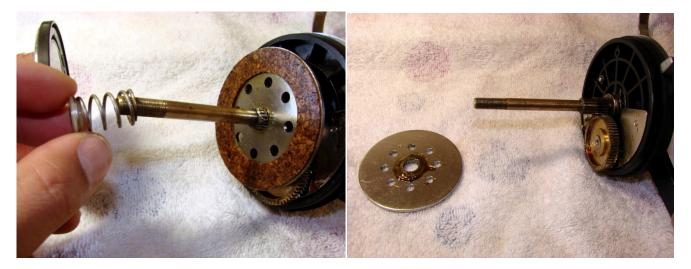
Remove the spring and plastic washer (#10054 and #10055) and the drag plate #10060. Note the washers (#10133 and #10062) and their orientation on the other side of the drag plate.
