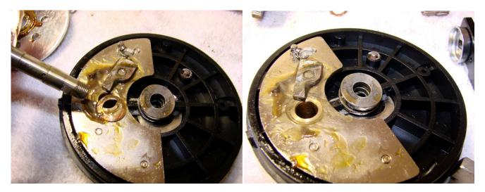
Remove the main gear (#10046) from the right side plate. Note the copper washer #10047.
