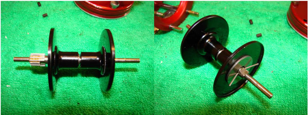
It must have been a huge amount of force to cause the spool to separate and bend the brake pins (judging by the force required to get them back together). I have no idea what could have caused it.
