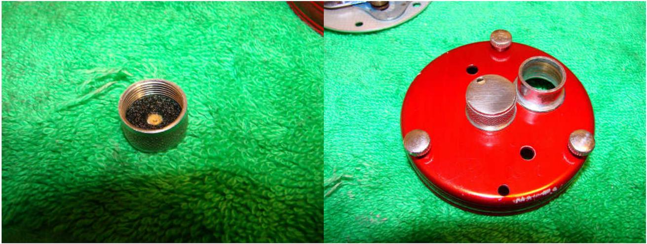
Replace the circlip in the right side plate followed by the bushing (soak in oil first and remove any excess). Replace the copper shims in the spool cap with a drop of oil. Replace the felt washer and saturate it with oil. Grease the threads for the spool cap and replace the spool cap ensuring that it is screwed in fully.
