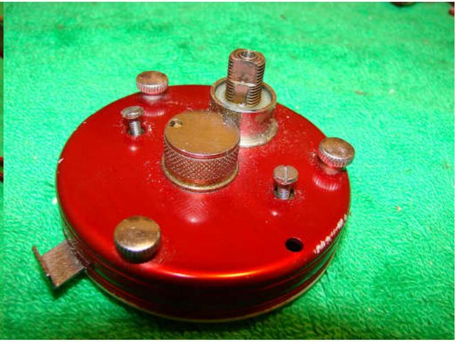
Remove the handle and star drag and then undo the three thumb nuts and remove the side plate from the frame. Undo the two bridge screws and remove the side plate from the brake plate.
