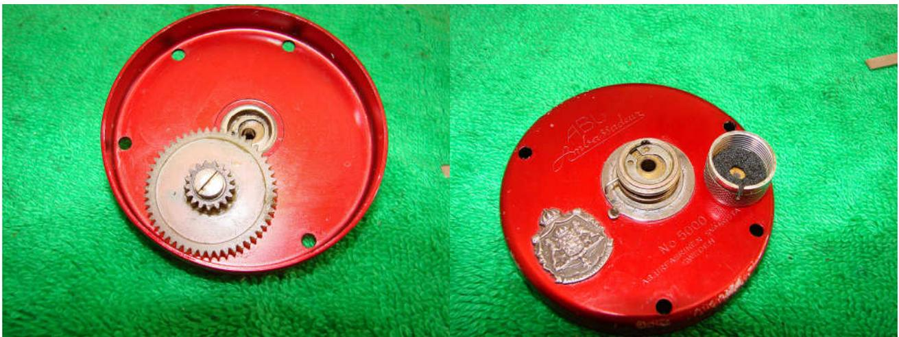
Remove the four pillar screws holding on the left side plate. Remove the idler gear screw and remove the idler gear. Turn the plate over and remove the spool cap.
