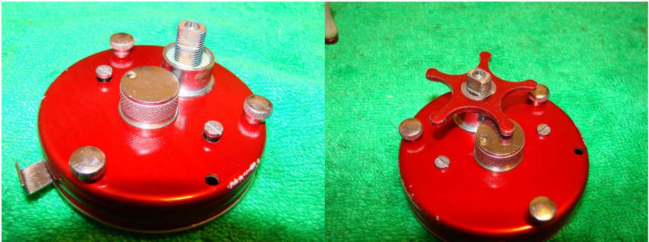
Replace the side plate on the brake plate. Grease the threads on the bridge screws and snug them down. Replace the star drag.
