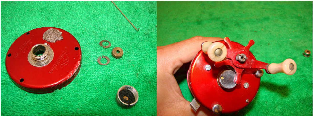
Remove the circlips and the bushing. The felt can be pried out of the spool cap with a tooth pick and the copper shims can be removed. Clean the felt washer by soaking in lighter fuel. Undo the handle nut and remove the screw.
