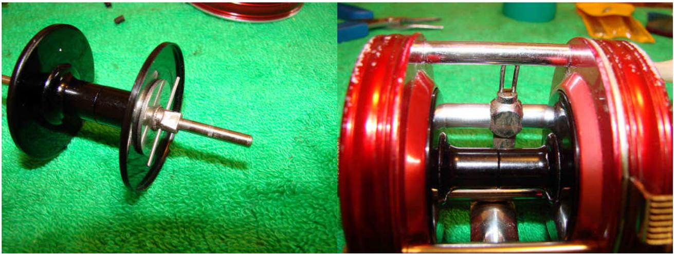
Pins all straightened. The spool is now a perfect fit in the frame and the centrifugal brakes work as they should. On with the rest of the service now that the spool has been fixed.
