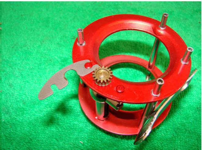
The carriage screw lock is on upside down here! Remove by sliding off.
