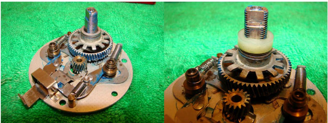
Replace the click wheel and then the curved washer followed by the flat washer and the drive shaft bearing. Smear liquid grease to the outside of the drive shaft bearing.
