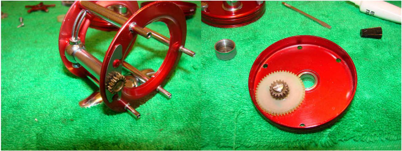
Replace the carriage screw lock, the pawl and the line carriage nut. Add a drop of oil either side of the carriage screw (in the threads). Add a drop of oil to the idler gear post and then replace the idler gear and the retaining screw. Spread liquid grease on the teeth of the idler gear.
