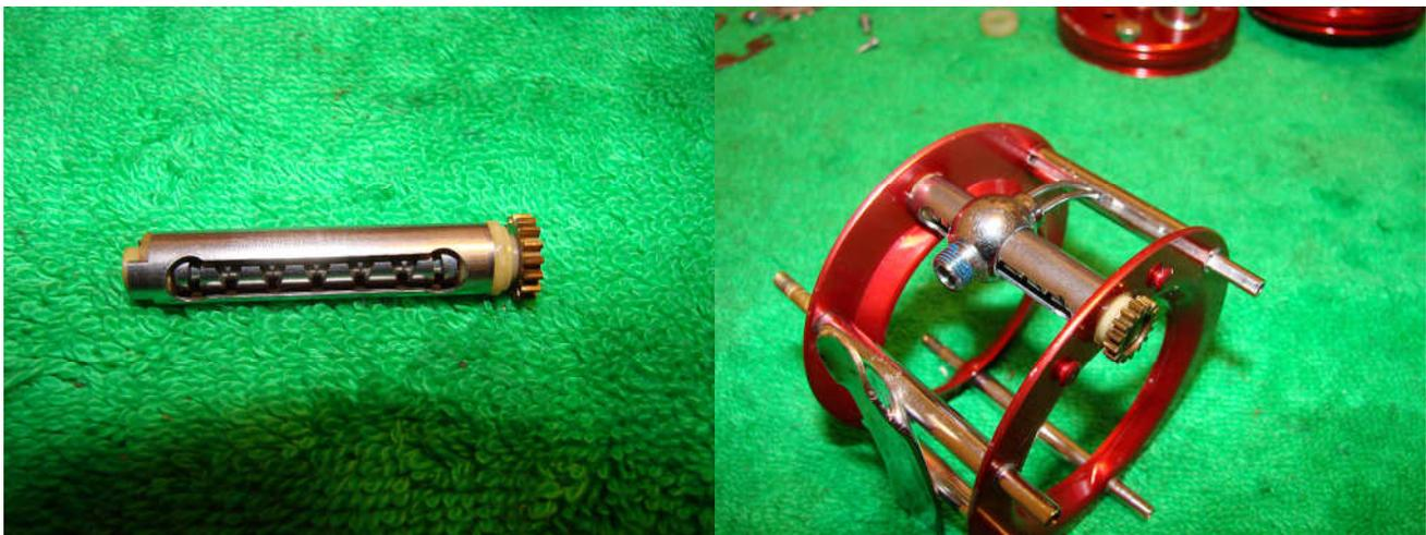
Add a drop of oil either side of the bushing on the carriage screw (near the gear) and one where it contacts with the plastic bushing in the cover. Place the assembly back in the frame. Grease the threads on the level wind.
