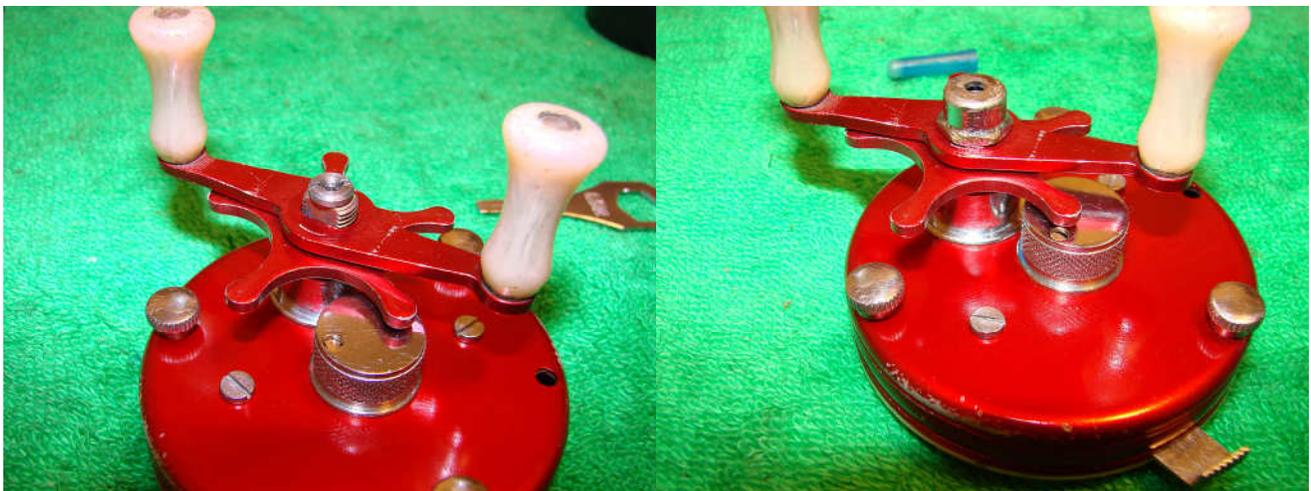
Replace the handle and drive shaft screw followed by the handle nut. Make sure it is snug as there is no handle nut lock on these older Ambassadeurs.
