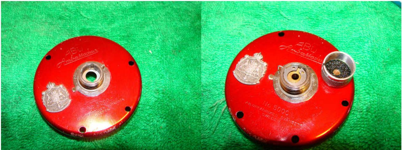
Replace the bottom circlip. Soak the bushing in oil and wipe of any excess and then replace it followed by the top circlip. Replace the shims in the spool cap (with a drop of oil), and then replace the felt washer. Apply oil to the felt washer and then replace the spool cap ensuring that the indicator wire fits properly into the slot.
