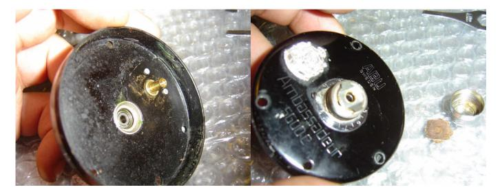
Remove the idler gear and then turn the plate over and remove the spool cap. There should be copper shims in the spool cap-these ones were bone dry and just dropped out. Note the spool-bearing cushion that sits under the spool cap. Remove this and then you have access to the bearing. Remove the bearing and give it a soak in a jar of lighter fluid, replacing the fluid as necessary until the bearing spins nice and freely. Leave it to dry on some kitchen towel while you do the rest of the service.
