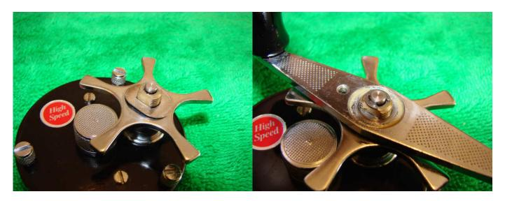
Replace the two screws holding on the side plate and then replace the star drag. Note the washer that sits on top of the star drag. Remember to add a thin smear of grease to the friction surfaces. Replace the handle and the circlip.
