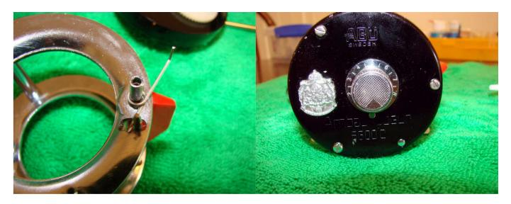
Note the orientation of the return spring for the thumb bar. Replace the left side plate and snug up the three screws holding it on.
