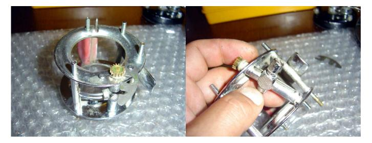
On narrow frame reels you may find it easier to remove the line carriage nut and pawl after you have removed the carriage screw lock, especially if you have big fingers! The carriage screw and worm guard will then simply slide out of the left side of the frame.
