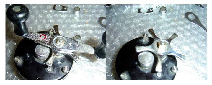
Remove the lock plate screw and lock plate, then the handle nut. Remove the c-clip and the handle will lift off. Remove the friction washer on top of the star drag and then unscrew the star drag.
