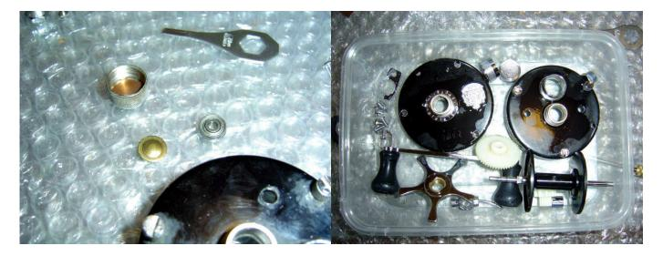
Unscrew the right spool cap. There will be a spool centering shim (brass colour) on top of the bearing. Remove this and then remove the bearing. The bearing can be soaked in a jar of lighter fluid while you work on the rest of the reel. Note the copper shims in the spool cap.
