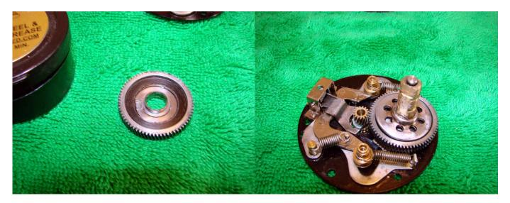
Lightly grease the top drag washer with drag grease and then place it in the main gear. Put the main gear on the drive shaft and replace the click wheel.
