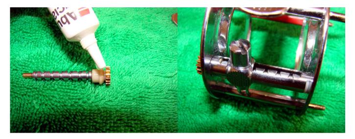
Apply a drop of oil to the plastic bushing making sure it soaks in. Apply another drop to the other end of the worm gear where it contacts the plastic bushing in the worm cover. Reinstall the level wind assembly back in the frame (opposite of removal). Apply a drop of oil either side of the worm gear (in the threads where the pawl contacts).
