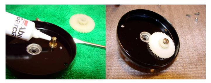
Turn the left side plate over and place a drop of oil on the idler gear post. Reattach the idler gear and retaining screw. I am happy to run the idler gear with no grease but if this is too noisy for you then use a light grease and apply it sparingly to the teeth.
