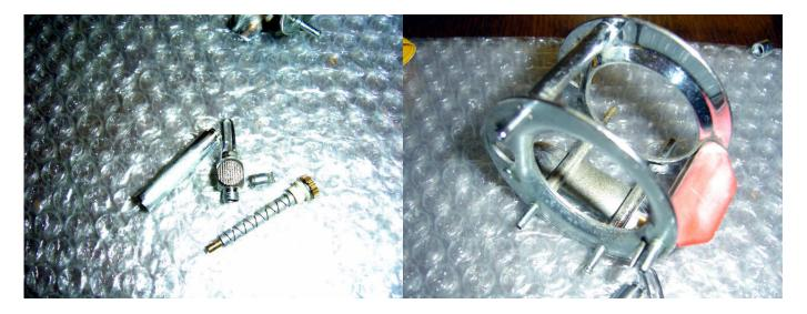
I'll replace the worm guard as it shows some wear but the pawl still looks good. The frame is showing some salt damage and this will need to be cleaned up.
