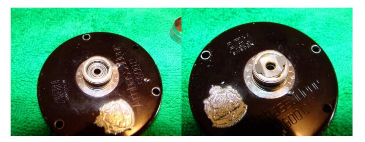
Apply a drop of oil of your choice to the bearing making sure that it penetrates fully. Replace the bearing in the left side plate and place the spool bearing cushion on top. Grease the o-ring and threads with a rubber friendly grease and then replace the spool cap (just a turn or two at this stage). Don't forget to place a drop of oil on the copper shims in the spool cap.
