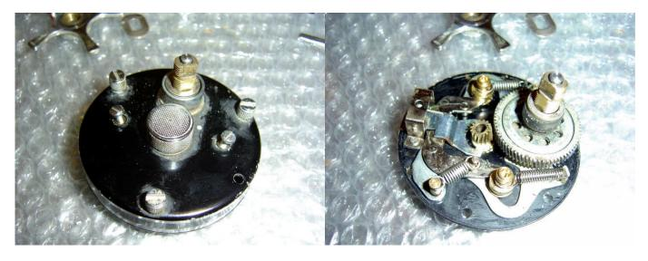
Remove the two bridge screws and the side plate will lift off. Not a spot of grease anywhere yet minimal corrosion-not so bad after all!
