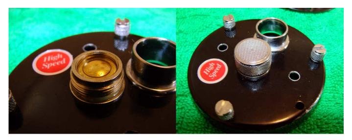
Replace the spool centering shim, add some grease to the threads and replace the right side spool cap making sure that it is screwed in FULLY. Don't forget to add a drop of oil to the copper shims in the spool cap.
