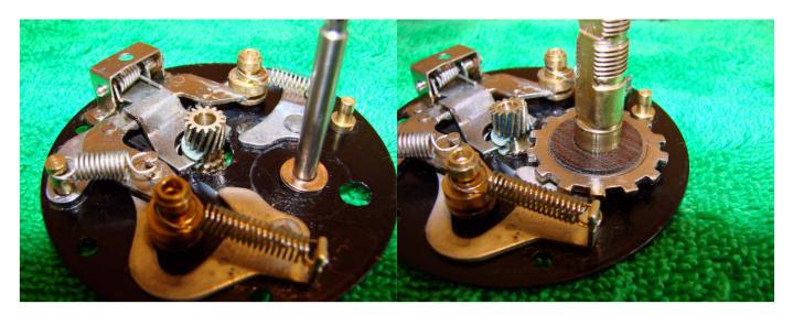
Replace the pinion gear adding a drop of liquid grease to where it sits in its' plastic collar. Smear some liquid grease on the drive shaft post and then replace the drive shaft. Apply a thin smear of drag grease to the base drag washer and place on the drive shaft.
