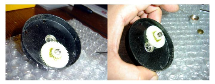
Turn the plate over for access to the idler gear. I have no idea what kind of lube that is, I'd rather not guess! Undo the screw holding the idler gear on.
