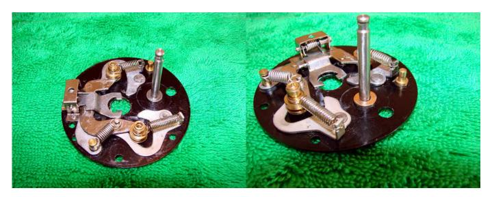
Carefully note where moving parts contact each other. You need to apply a *thin* smear of grease on these surfaces. An old toothbrush or small paintbrush is useful for this. Apply a drop of liquid grease (or mixture of oil and grease) to the base of the drive shaft post and then add the copper shim.
