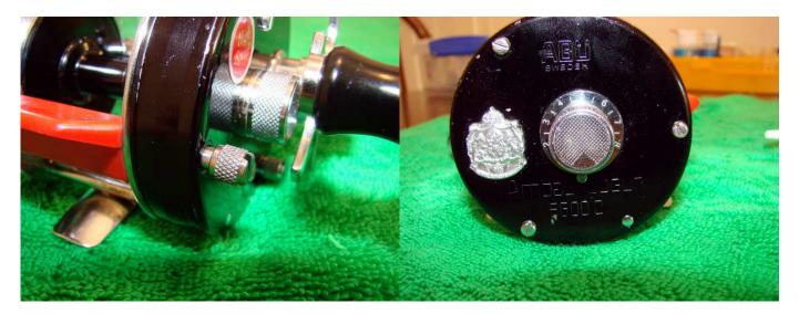
Tighten up the three thumb nuts on the right side plate. Place the reel in free spool and adjust the left spool cap until the spool just starts to rotate. Move the numbered ring until the zero corresponds with the mark on the spool cap.
