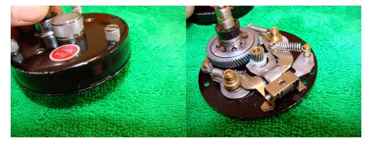
You may find it difficult trying to replace the right side plate to the brake plate because the press arm stops the side plate seating fully. An easy fix is to put the reel (i.e. the brake plate) in free spool. You can do this by
