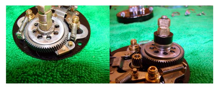
Make sure that the anti reverse pawl is properly engaged. Replace the metal washers and drive shaft bearing-note the orientation of the washers from your reels' schematic diagram.
