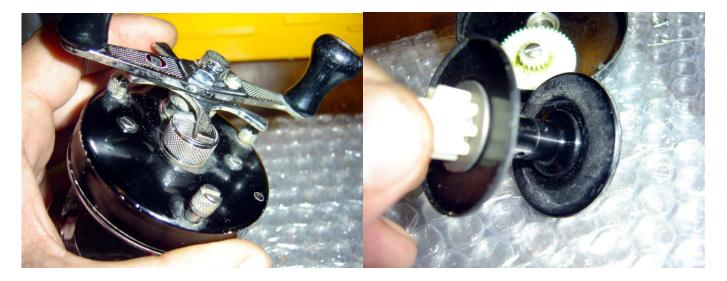
Unscrew the three thumbnuts holding on the right side plate, remove the plate and spool as one unit from the right hand side of the frame. It looks like the handle nut is cross-threaded here and someone has tried to tighten it with a pair of pliers.
