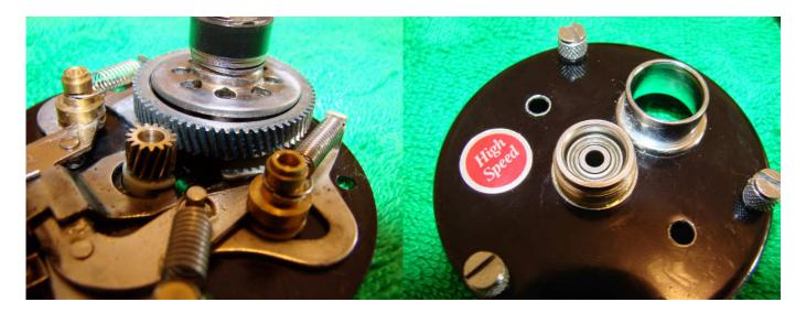
Apply grease sparingly to the gear teeth. Apply a drop of oil to the bearing and replace it in the right side plate.
