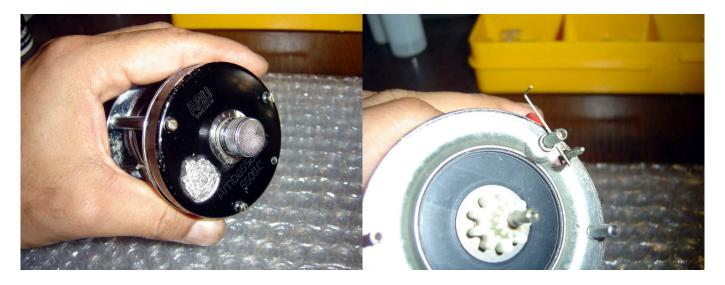
Undo the three pillar screws on the left hand plate and remove it. Note the return spring for the thumbar.
