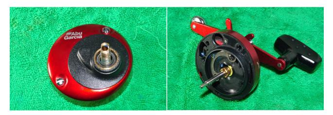
Replace the outer metal side plate. Clean the IAR bearing and sleeve (a cotton bud is good for this) and then very lightly coat with oil (too much lubrication here will make the IAR bearing slip).
