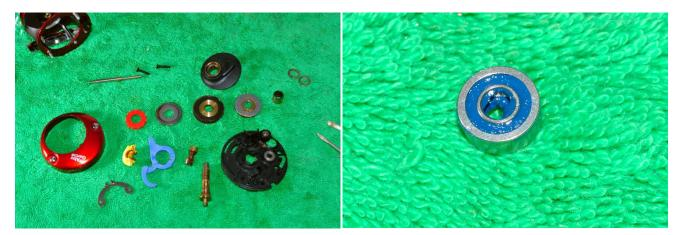
The entire right side plate can then be disassembled and given a thorough clean. Don't forget to remove the bearing at the base of the gear shaft (in the photo above it is still in the brake plate). Thoroughly clean this and then pack with grease. In this case I removed the shields to ensure it was clean and dry and then packed with grease before replacing the shields.
