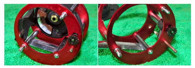
Below the level wind gear there is the guide bar for the level wind-note that the end is slotted and it screws into the left inner side plate. Unscrew this and remove from the frame and the left inner side plate can then be removed. Note the salt deposits.
