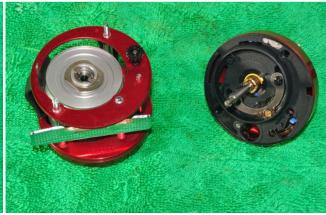
Note there are only two pillar screws on this model. Remove them and lift off the entire right side plate.
