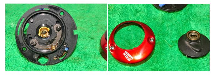
To remove the right side plate you will need to undo the two screws on the inner side of the brake plate (this photo shows the side plate already removed-I have replaced the screws for the purpose of the photo). The black plastic housing for the IAR bearing and the metal side plate can then be removed. To remove the main gear shaft you will need to remove the metal lock washer (on the first photo with the two screws).
