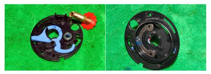
Replace the ratchet wheel (red plastic part) on the main gear shaft (note correct orientation) and then replace in the brake plate. Fix it in place with the metal lock washer.
