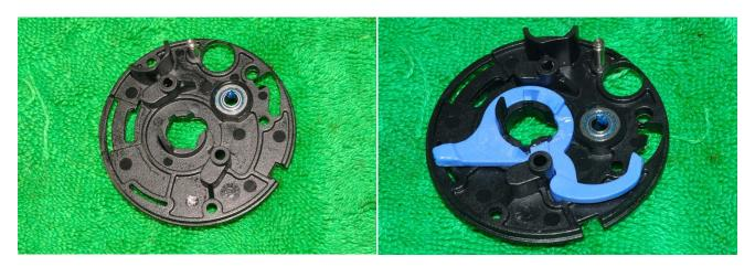
Replace the bearing in the brake plate. Lightly grease the friction surfaces on the clutch arm (blue plastic part) before replacing on the brake plate.
