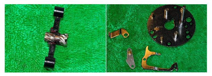
Remove the pinion gear holder. The pinion gear simply pops out of the holder-nice to see here that it is stainless steel. Finally remove the clutch arm, the release trigger, and the link arm from the brake plate.
