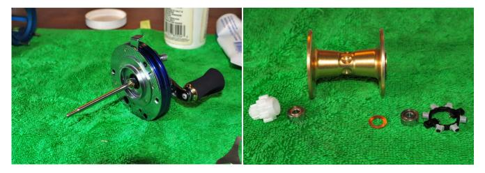
Replace the right spool cap. Add some oil to the main shaft where it contacts the pinion gear and then replace the shaft in the frame. It should click into place (the end of the shaft is held captive with a plastic clip in the right spool cap).
