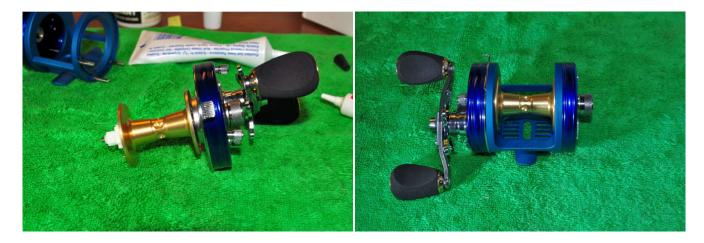
Ensure that the centrifugal brakes are pushed in enough to clear the brake ring on the brake plate and then slide the spool onto the spool shaft. You may find it easier if you put the reel in free spool. Slide the whole side plate and spool assembly into the frame and then tighten the thumb nuts.
