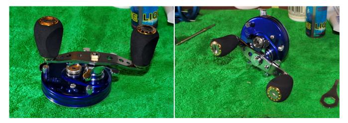
Replace the handle and c-clip and then fix the handle in place with the handle nut and locking plate and locking plate screw.
