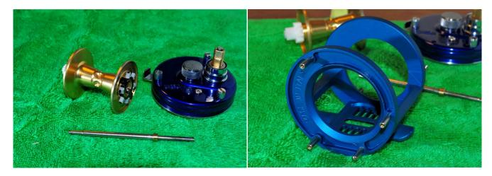
Remove the spool from the shaft and then pull the spool shaft out of the side plate-it is held in place with a plastic clip that sits in the right spool cap. The left side plate has been removed in order to have a good look at the frame. The left plate is held on by three pillar screws in usual Ambassadeur fashion.
