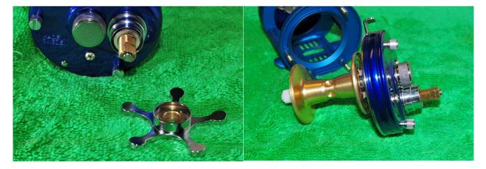
Unscrew the star drag. Undo the three thumbnuts on the right side plate and remove the side plate and spool assembly.
