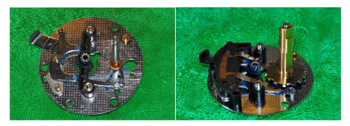
Replace the pinion gear in the pinion gear holder and replace on the brake plate. Add a light coating of grease to the gear teeth and also where the pinion gear contacts the pinion holder. Add a light coat of liquid grease (I find oil too light and grease too heavy) to the shaft and then replace the copper washer (add a drop of liquid grease to the copper washer as well). Replace the main shaft and the position holder.
