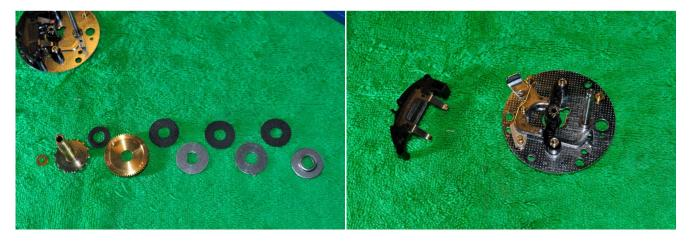
Main gear/drag assembly laid out in order (left to right = bottom to top). Interestingly the fibre base drag washer and middle drag washer are standard issue whilst the other two are the newer carbontex material. Remove the position holder from the brake plate.
