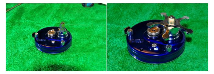
Replace the side plate and fix in place with the two screws. Replace the sleeve for the IAR bearing (use a very light oil and sparingly-too much lubrication will cause your IAR bearing to fail). Replace the two Belleville washers in () configuration. Replace the star drag and washer.
