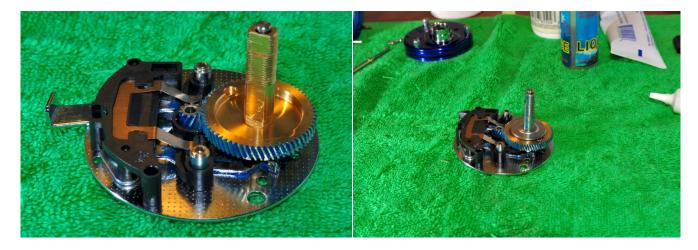
Replace the main gear (add a coating of grease to the teeth making sure you have total coverage). Replace the drag washers in the correct order (check the photo of the disassembled drag if unsure of the order). Make sure that the metal washer with 'ears' is seated correctly in the main gear.
