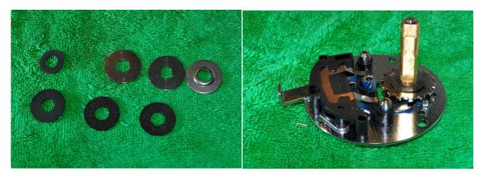
I like to run the drags with a light coating of drag grease on the fibre washers (Cal's drag grease is great). Replace the bottom fibre washer and add a smear of drag grease around the shaft where the main gear contacts-this is very important.
