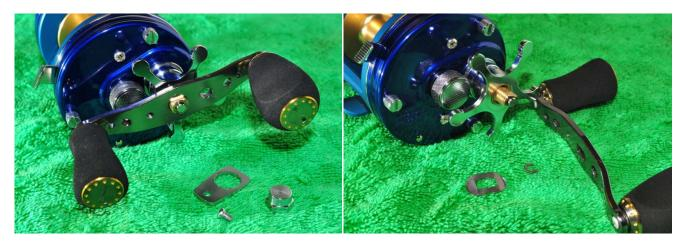
Servicing this reel should be no more difficult than a standard ABU CT reel. Remove the screw holding on the handle nut locking plate. Remove the lock plate and the handle nut. Remove the c-clip with the blade of a fine screwdriver and then remove the handle. Note the washer that sits between the handle and the star drag.
