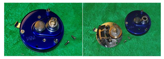
Remove the two post screws and then remove the side plate from the brake plate. It's nice to see that the brake plate is chrome plated brass. They feel a bit more robust than the aluminium ones. There is a stub for an old style anti reverse dog on the plate-with a thicker base drag washer you should have enough clearance to fit an anti reverse dog as a failsafe backup if your IAR bearing was to fail whilst fishing.
