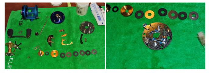
Give everything a thorough clean before reassembly. Remember when you reassemble to lightly coat the threads on screws with grease-this makes any future work much simpler and prevents any screws corroding and getting stuck.
