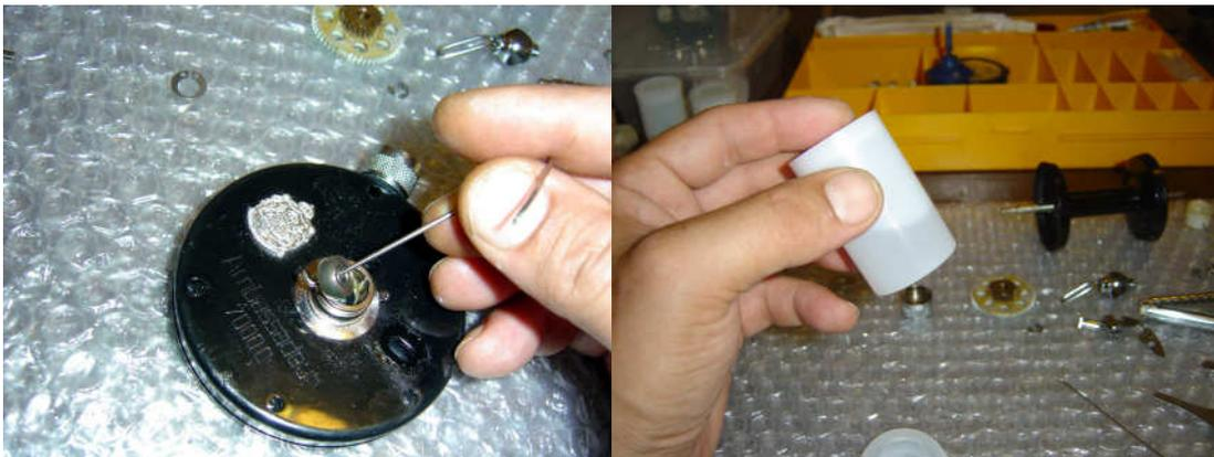
Remove the bearing. I find a bent paperclip works well.
