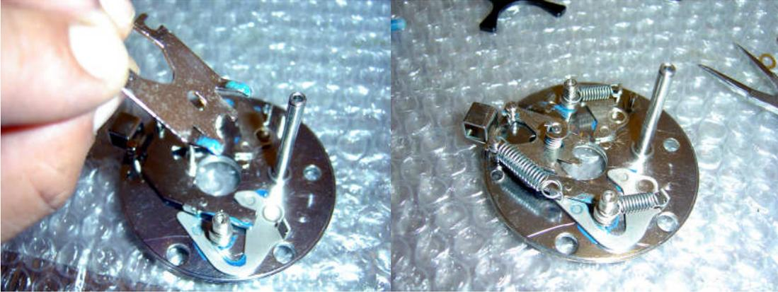
Replace the clutch arm and then the lock arm springs, clutch spring and pinion yoke spring.
