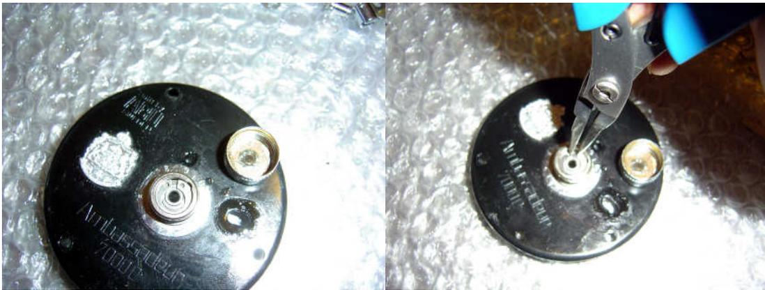
Unscrew the spool cap. If you have circlip pliers use them to remove the circlip (spool bearing lock) holding in the bearing. I use a pair of needle nose pliers with the tips filed down to fit.
