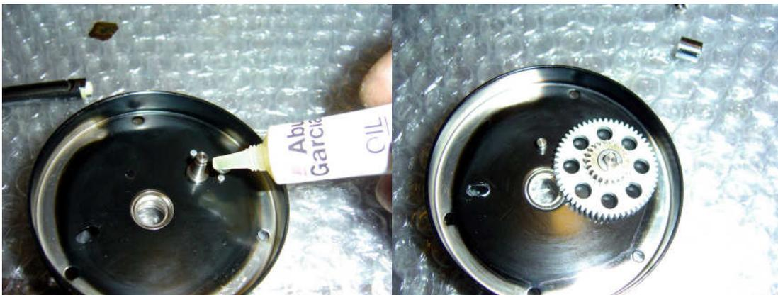
Put a drop of oil on the idler gear post then add the idler gear and c-clip.
