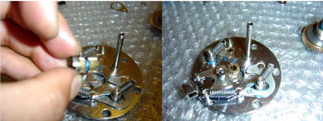
Add some grease where the pinion gear contacts the clutch arm. Newer reels have the pinion gear sitting in a plastic bushing. Replace the pinion gear in the clutch arm-you may find it easier from the other side of the brake plate.
