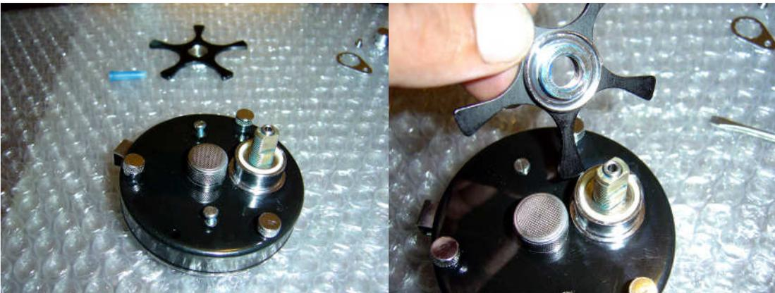
Replace the side plate and replace the bridge screws (make sure the threads are greased) taking care not too over tighten. Add a smear of grease to the base of the star drag where it contacts the bushing in the side plate.
