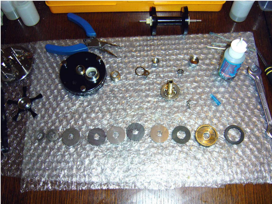
**PHOTO 49** Everything laid out in order top to bottom (left to right). The drive shaft bushing is to the right of the side plate. These drag washers are actually a bit worn-I have some carbontex fibre and metal washers on order and they will be replaced as soon as they arrive.
