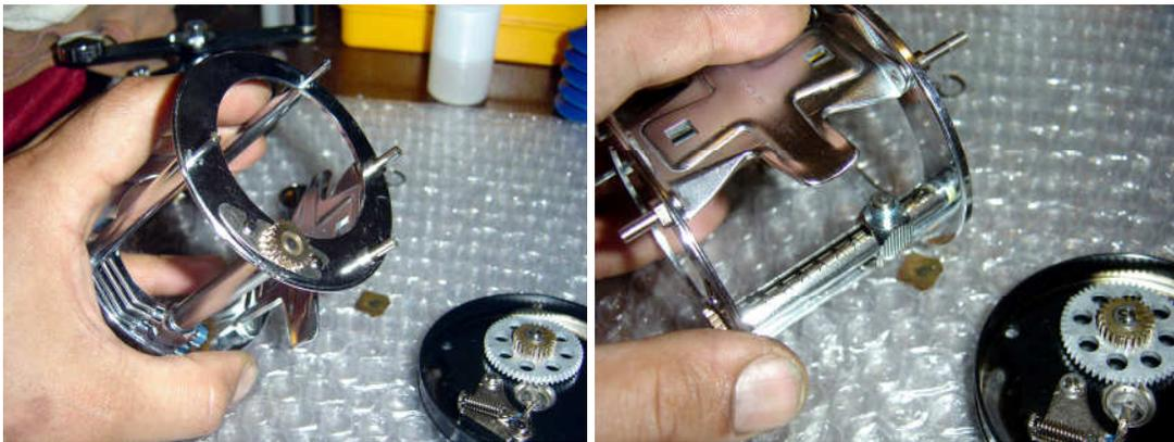
Reassembly back in the frame is the opposite of disassembly; make sure that the top of the line guide sits properly in the groove in the frame crossbar.
