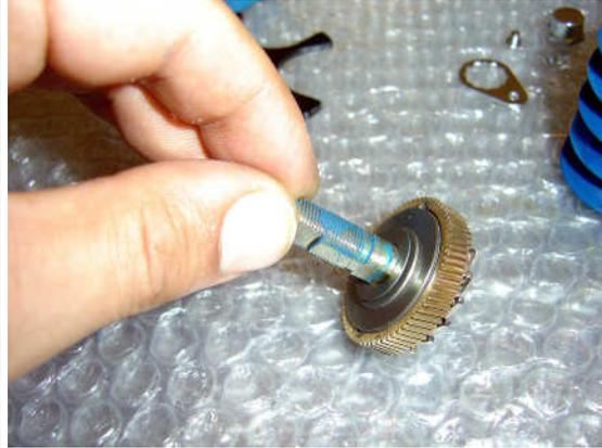
Replace the two spring washers on top of the drag stack. The larger diameter one sits on the bottom in this orientation ). Put a smear of grease on the shaft.
