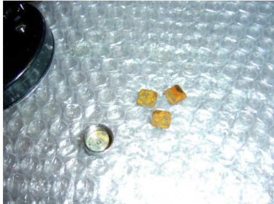
Unscrew the spool cap and remove the copper shims. It looks like salt water has been in here so I'm sure the bearing will be junk like the other one. It's best to replace them as a pair anyway.
