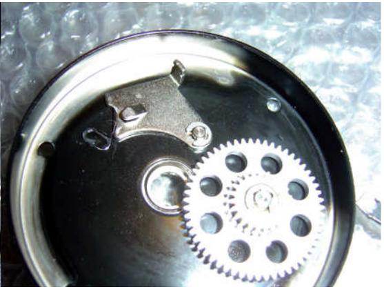
Replace the click plate post in the side plate and smear some grease on the back of the click plate. Place the click plate on the post and replace the circlip.
