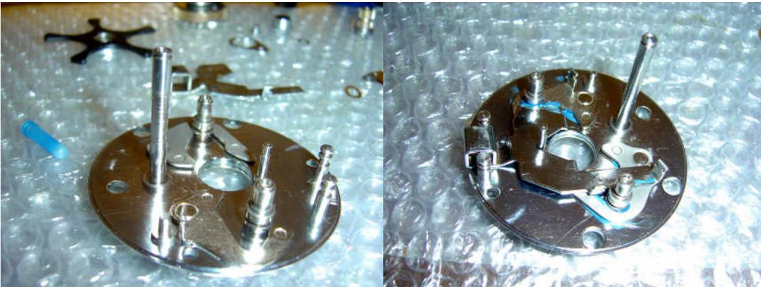
Note where moving metal parts contact each other and smear these surfaces with a thin film of grease. Replace the press arm (release trigger).
