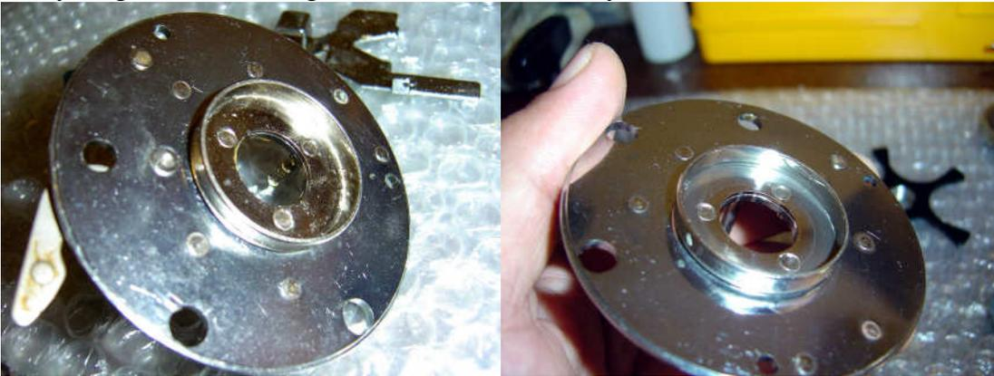
Check the brake drum (brake ring). In this case it looks like some saltwater has entered so it needs to be polished up
