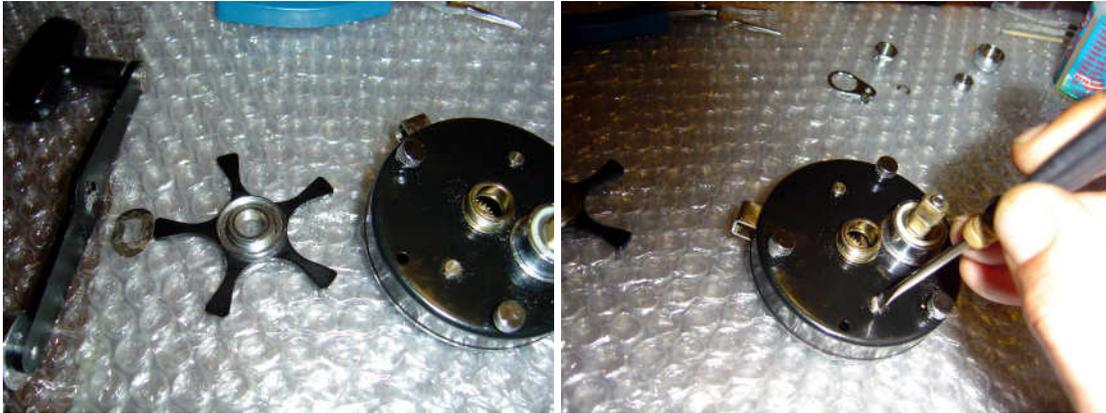
Remove the star wheel. Note that there is a friction washer between the handle and the star wheel. Remove the two bridge screws and then lift off the side plate.
