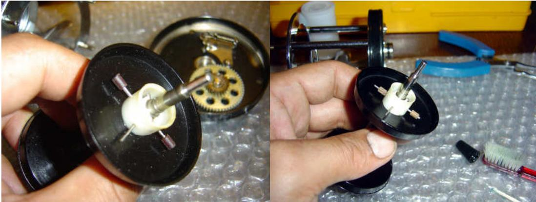
The centrifugal brakes look to be soaked in oil and the spool shaft needs a bit of a clean up too. The brakes can be cleaned with lighter fluid. If you find that dry brakes make too much noise for you then you can run a cotton swab with a miniscule amount of oil on it around the braking surface in the brake ring.
