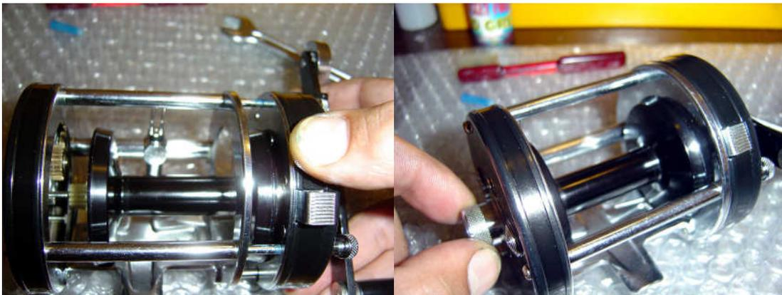
Grease the three studs on the frame and then the whole assembly can be slid into the frame. Tighten up the thumbnuts.
