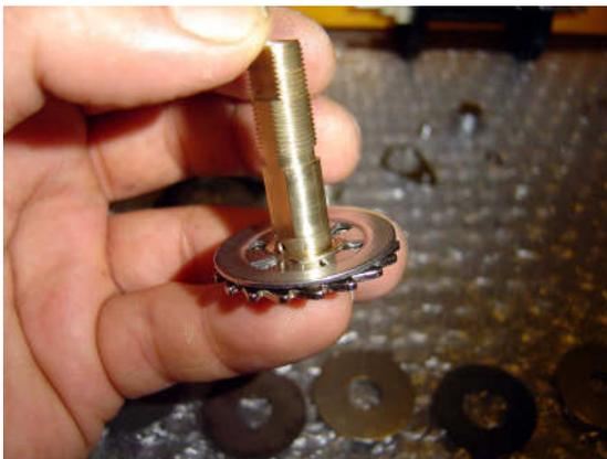
Before tackling the brake plate we'll start on the drive shaft assembly. Make sure that everything is clean and free from corrosion. The drag washers can be cleaned by wiping down with a soft cloth and some lighter fuel.
