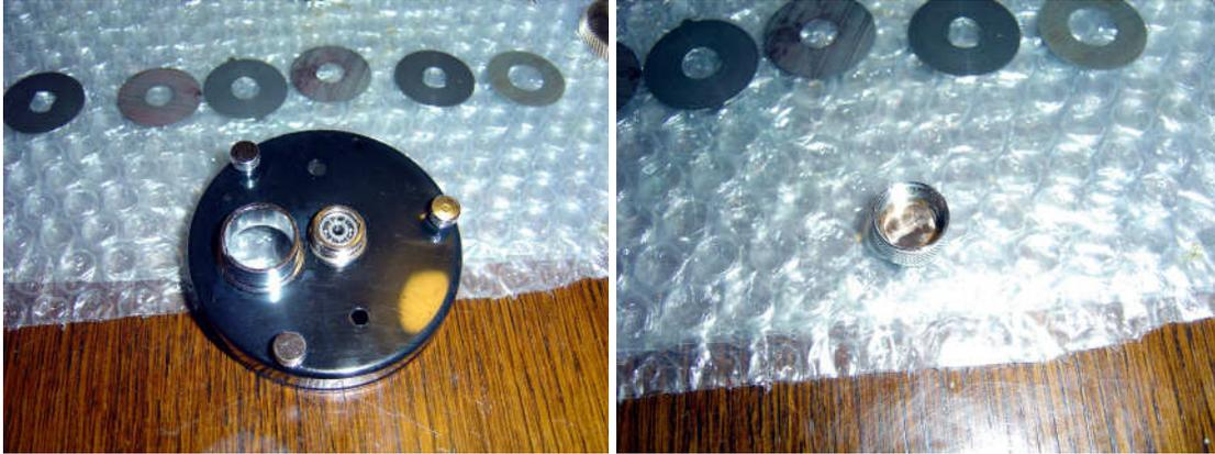
After cleaning the side plate in goes a new bearing lubed with a couple of drops of oil. Note there is no bearing lock in this side. Make sure the copper shims are nice and clean. Add a drop of oil and the spool cap is ready to go back on the side plate.
