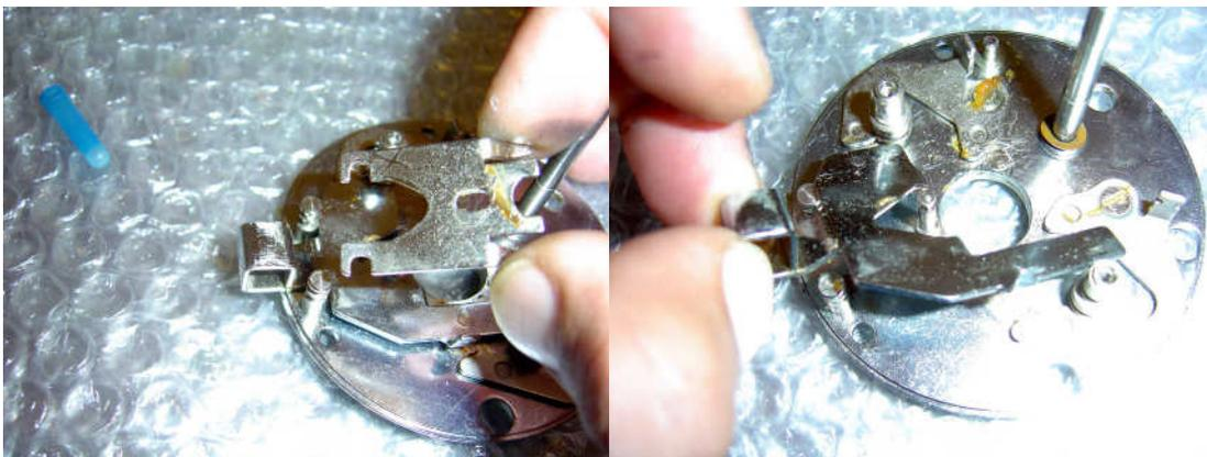
Remove the clutch arm and then the press arm (release trigger).
