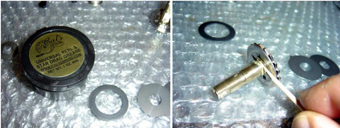
The base drag washer should be greased regardless if you like to run your drags wet or dry. Use a good quality drag grease-I find Cal's to be excellent. Make sure that you use the drag grease *sparingly*. A dry washer and a greased washer should look the same. In this case I will be using the other drag washers dry (no grease).
