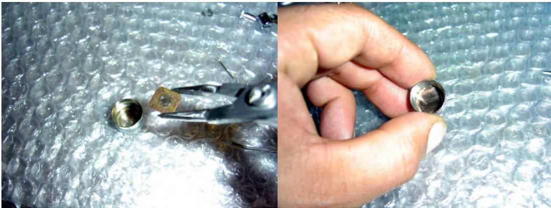
Remove the copper shims from the left spool cap and give them a good clean. They are then ready to go back into the spool cap with a drop of oil.
