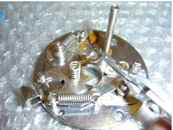
Remove the pinion yoke lock. This is easiest if you push down on the pinion yoke spring while you are removing it. Keep a firm hold on the spring as it will want to disappear into the distance.
