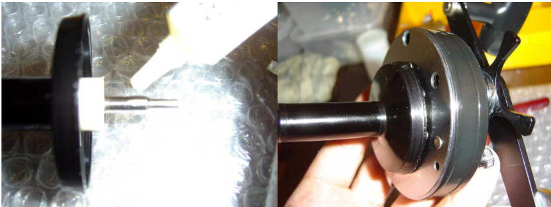
Add some oil to the spool shaft where it contacts the pinion gear. Make sure that the centrifugal brakes are pushed in fully and then place in the right hand side plate making sure it is seated properly.
