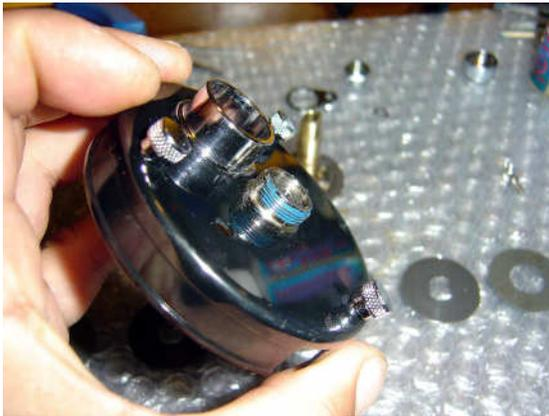
Add some grease to the threads and then screw down the spool cap *fully*. Note that there is no o-ring on this side and so the spool cap *must* be screwed in fully.
