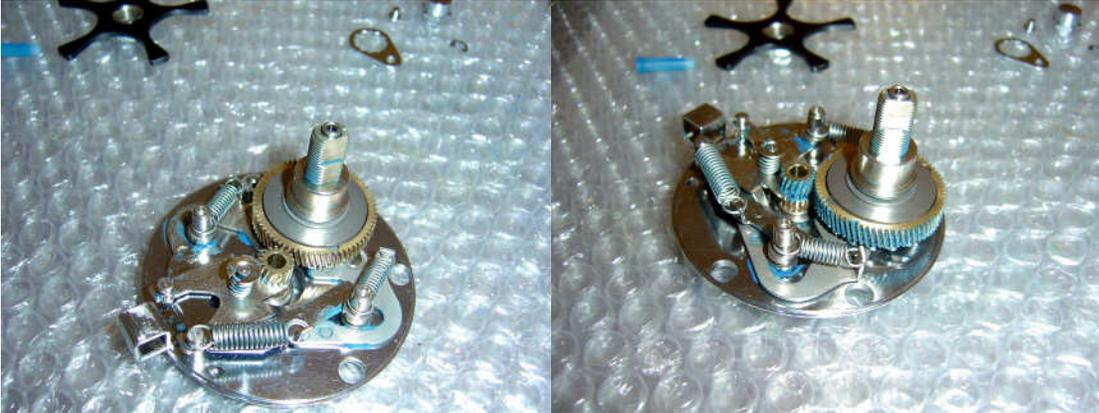
Add a thin smear of grease to the gears-you can use a toothpick or a fine paintbrush to spread evenly. I like to turn the gears to ensure coverage on the pinion gear.
