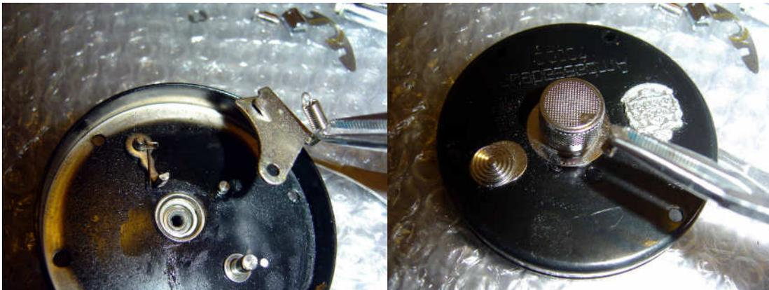
You can then remove the click plate. Normally the click plate post should drop out; here it's a bit of a tight fit. In this case you can push it through and then remove from the other side.
