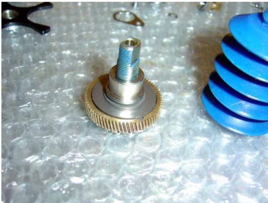
Replace the bushing. I place a smear of liquid grease on the outer surface of the bushing where it contacts with the plastic in the side plate.
