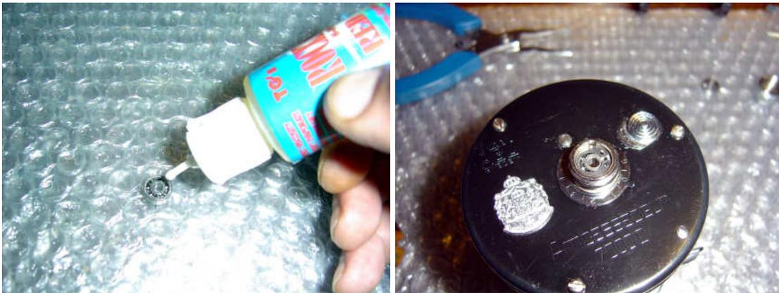
Add a drop of oil to the bearing before putting it back in the side plate. I like Rocket Fuel Red Label for 7000 size reels.
