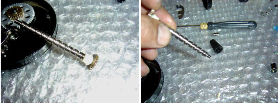
Put a drop of oil either side of the plastic bushing on the carriage screw making sure it soaks in properly.
