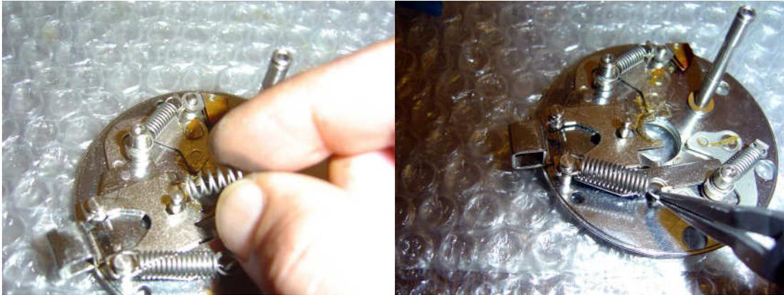
Remove the pinion yoke spring followed by the clutch spring.
