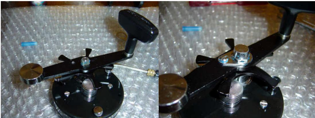
Replace the handle and c-clip and then tighten up the handle nut (don't over tighten). Add a thin smear of grease to the base of the handle nut lock and then replace the locking screw (don't forget to grease the threads).
