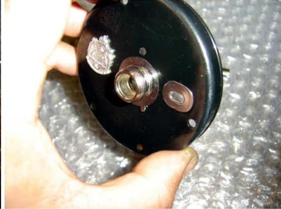
Smear some grease on the back of the click button plate and replace it in the side plate.
