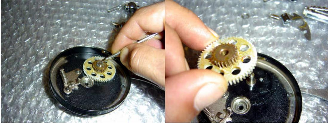
Remove the c-clip holding on the cogwheel (idler gear). Be careful as it will fly off somewhere if you're not holding on to it.
