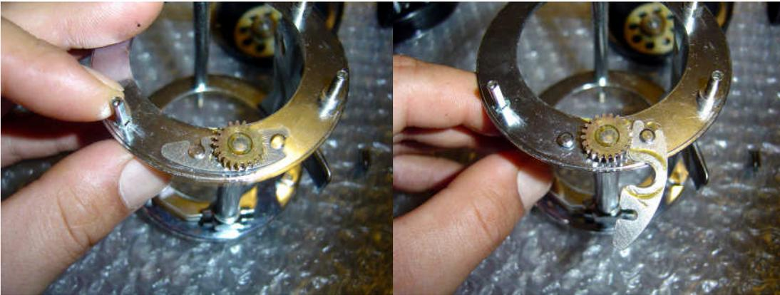
Note orientation of carriage screw lock. Remove carriage screw lock by sliding the top off first.
