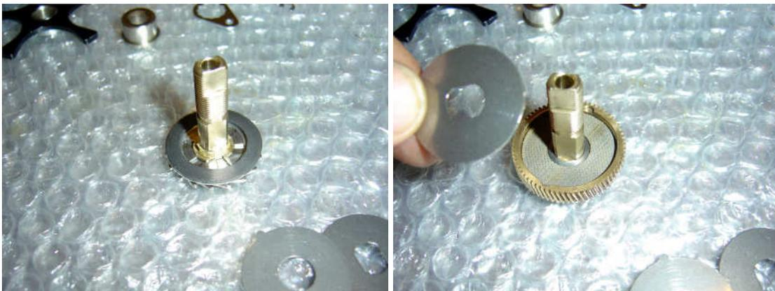
Replace the base drag washer and then the main gear followed by the base fibre drag washer. Note that the base fibre drag washer has a larger diameter inner hole than the two other fibre washers. After the base drag washer replace the first metal drag disc as shown in the photo above.
