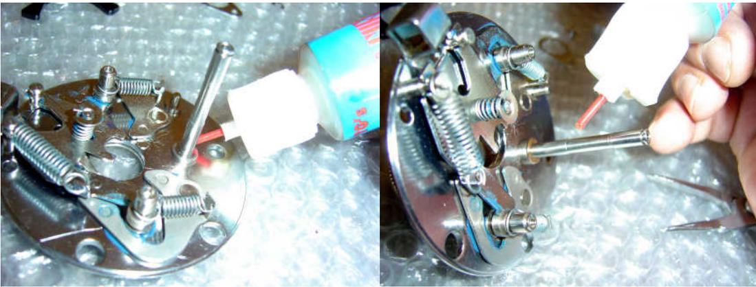
Add a drop of liquid grease to the base of the drive shaft and add the copper shim. Grease the drive shaft with liquid grease-I find oil too thin and grease too thick.
