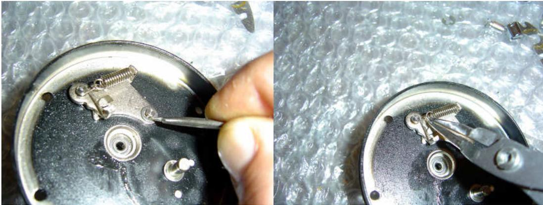
Remove the c-clip holding on the click plate and unhook the click pawl spring.
