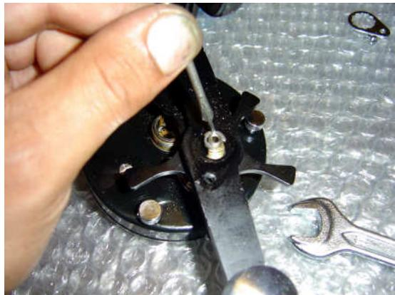
Remove the screw holding on the handle nut lock. Remove the handle nut lock and the handle nut. Remove the c-clip and then the handle. Be careful with the c-clip as it will want to spring off.
