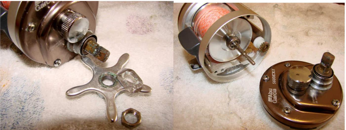
Remove the friction washer and undo the star drag. Undo the two side plate screws (the ones at the top and the bottom of the side plate) and remove the side plate. If the side plate seems hard to remove try pushing on the clutch plate from the inner side of the frame.
