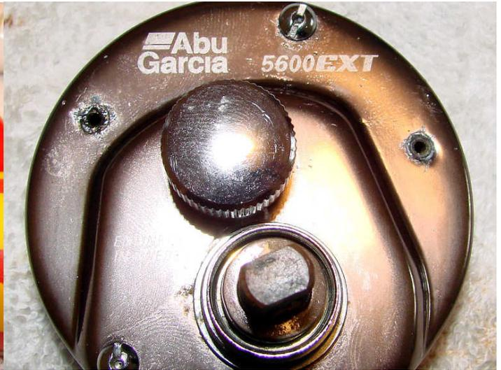
The clutch plate shows some salt deposits-interestingly it is made of plastic; no corrosion worries at least! Remove the two remaining side plate screws and lift the side plate from the clutch plate. Unfortunately the right side plate is showing a little bit of corrosion around the screw holes.
