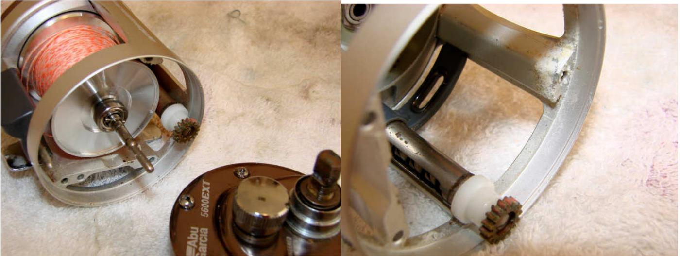
Remove the spool from the right side of the frame. The frame and level wind look as if they have been affected by salt water.
