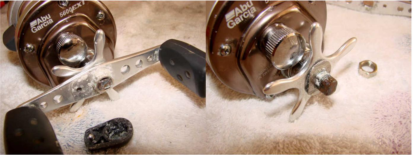
Remove the handle nut cover and the handle nut. Lift off the handle. Salt deposits are very evident.
