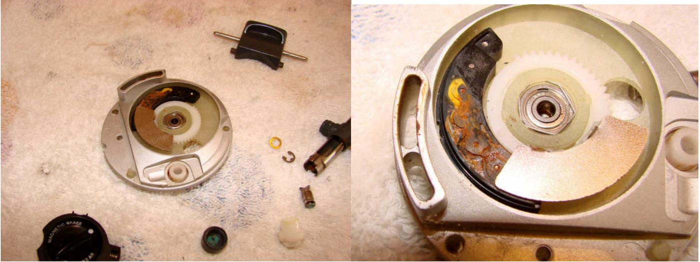
Push the inner side plate out from the frame-there are no screws holding it in place. The corrosion on the magnet carrier doesn't look good.
