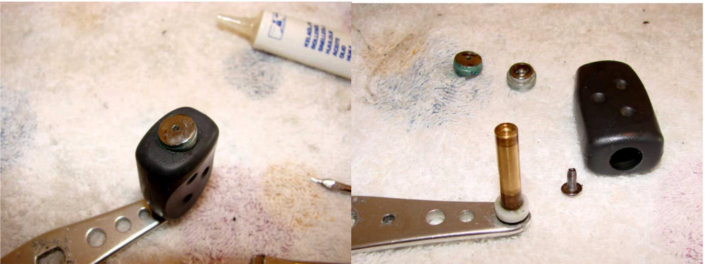
Before replacing the handle you can grease/oil the spindles for the handle knobs.
