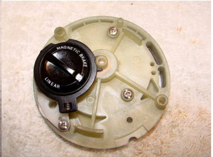
Replace the mag carrier in the inner side plate and fix in place with the two screws. The mag adjuster can then be replaced on the side plate.
