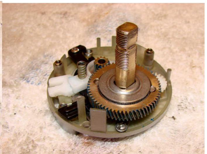
Apply some light grease to the teeth on the plastic level wind drive gear and ensure it is sitting correctly underneath the main gear before replacing this on the drive shaft.
