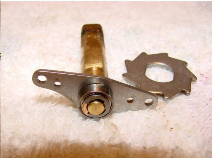
Remove the two screws holding the main shaft assembly and remove from the brake plate. The ratchet slides off the main shaft. Note the circlip at the base of the main shaft. Remove this and separate out the parts.
