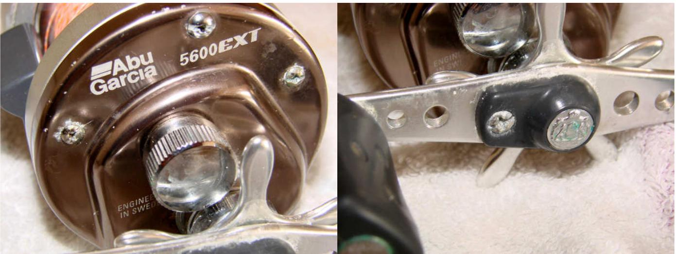
The screws and part of the side plate have suffered from saltwater corrosion. The screws were actually seized tight and wouldn't move. Don't try to force stuck screws-this may cause them to snap off, especially if they have been badly corroded by salt. In this case the screws were liberally coated with penetrating fluid and left overnight. Fortunately this did the trick.
