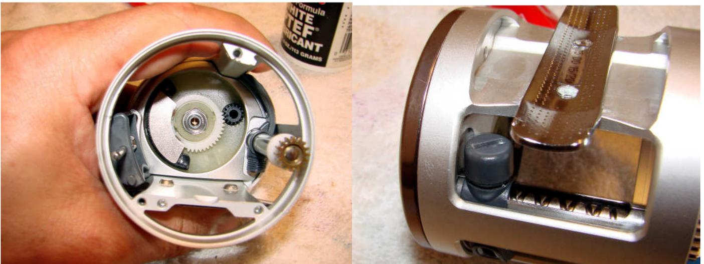
Make sure that the line guide is sitting correctly in the frame and then replace the pawl and washer and the line guide nut. Add a few drops of oil to the grooves in the worm gear.
