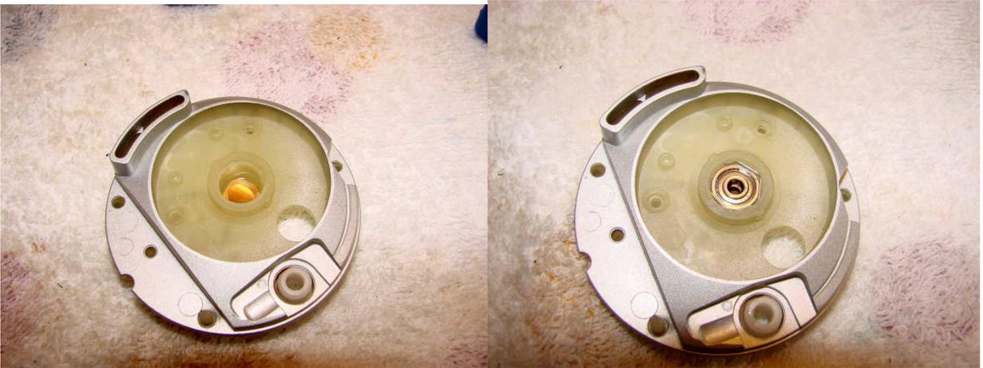
Add a drop of oil to the copper shim and then replace the bearing and clip.
