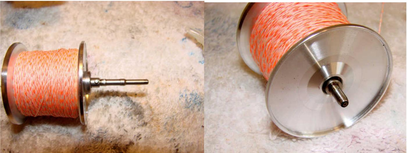
Add a drop of oil to the bearing on the right side of the spool. Clean the spool shaft thoroughly and smear some oil on the right hand shaft where it contacts the pinion gear. Clean both spool tips and add a drop of oil to each end.
