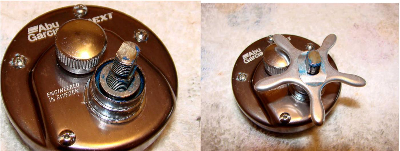
Grease the o-ring and the threads for the spool cap and then replace it on the side plate. Make sure that the threads on the main shaft are greased and then replace the star drag and the friction washer.
