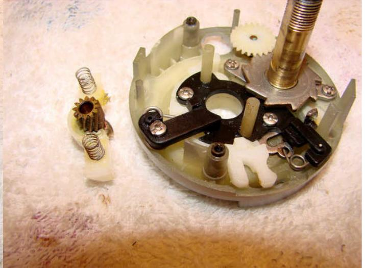
The left photo shows the clutch plate before disassembly. Firstly remove the pinion yoke (with two springs) and the pinion gear.
