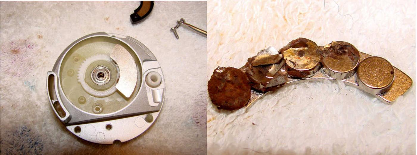
Replace the mag adjustment plate by lining up the notches.
