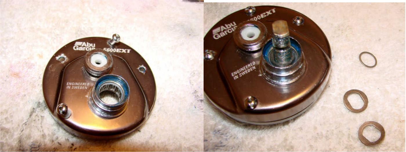
Replace the side plate on the clutch plate and fix in place with the side plate screws-of course the threads are greased now! Three washers need to be replaced on top of the bearing sleeve-the small washer is first followed by the two curved washers. Note that the correct orientation is ( ).
