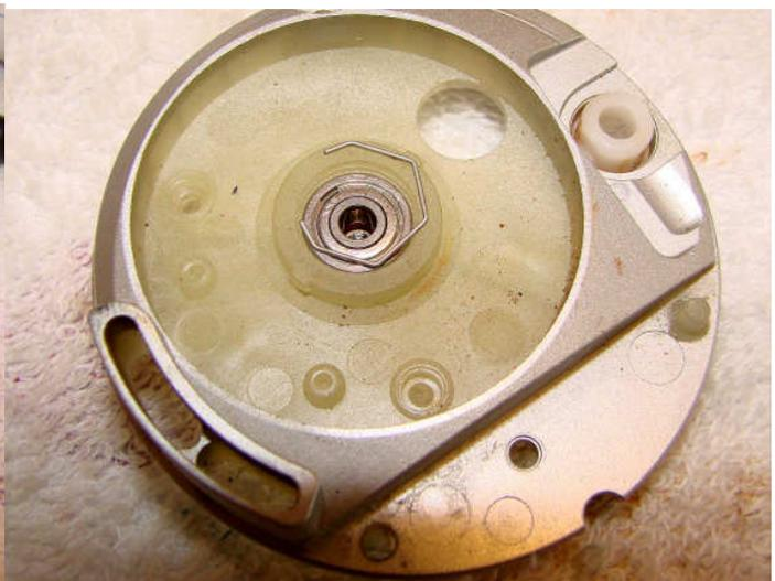
Remove the bearing from the left inner side plate-it is held in place with a clip. Give the bearing a thorough clean and when it is dry add a drop of oil of your choice. There will be a copper shim underneath the bearing-clean this off and then replace in the side plate.
