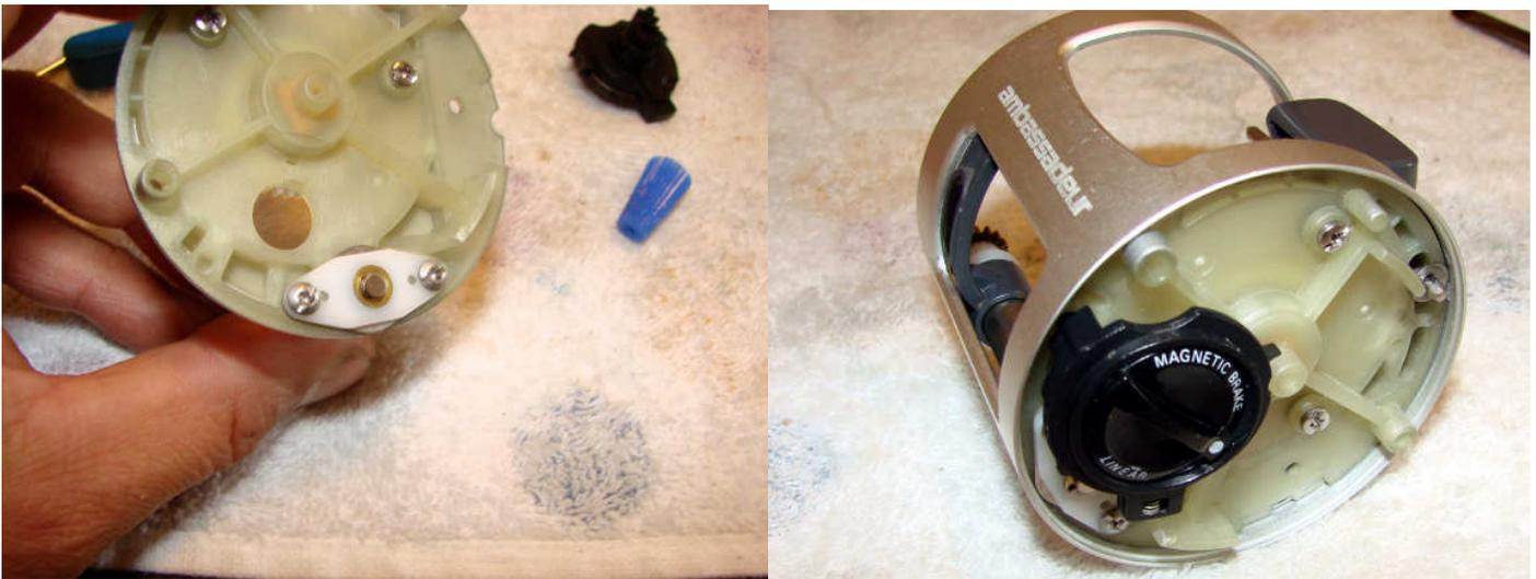
Reassemble the whole level wind assembly and replace it in the side plate. You may find it easier to do this if you replace the side plate in the frame first and without the mag adjuster in place.
