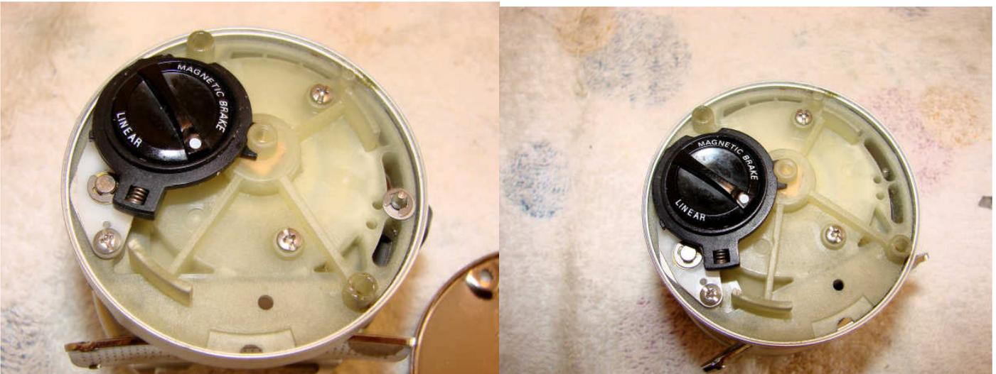
Interestingly the inner side plate is also plastic-note the drain holes at the bottom of the inner side plate. To the right of the inner side plate is a circlip holding the thumb bar in place. Remove this to free the thumb bar from the inner plate.
