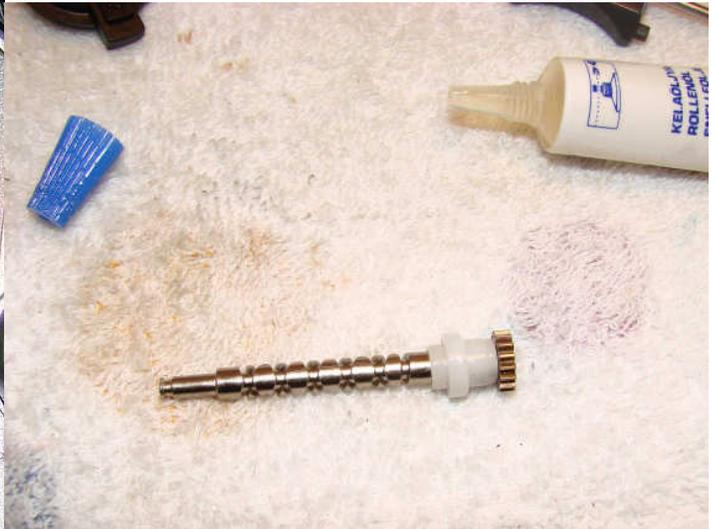
Note the reference marks for the mag adjuster. You need to line up the marks correctly or you will not have full adjustment for the mag control.
