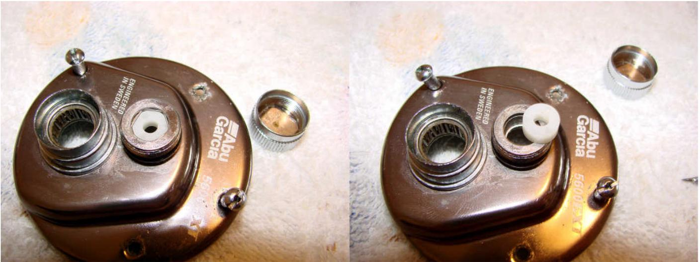
Remove the right spool cap. Remove the clip and take out the plastic bushing. Give the bushing a thorough clean before replacing and fixing it back in place with the clip. Remove the copper shims from the spool cap and give the cap and shims a thorough clean. Add a drop of oil in the spool cap before replacing the shims. Add a drop of oil on top of the shims (the spool shaft contacts here).
