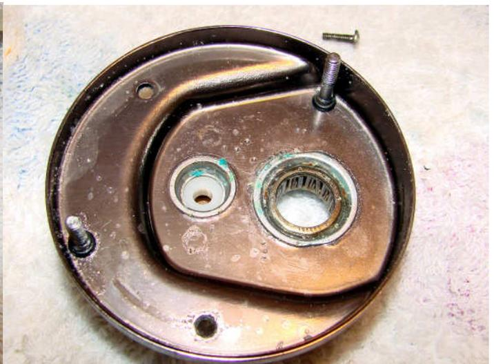
These screws need to be replaced. Fortunately the inside of the side plate is not as bad as it looks. The IAR bearing works fine and the corrosion on the plate can be cleaned off. To prevent future corrosion you can put a little bit of grease on your finger and smear it on the inside of the side plate.
