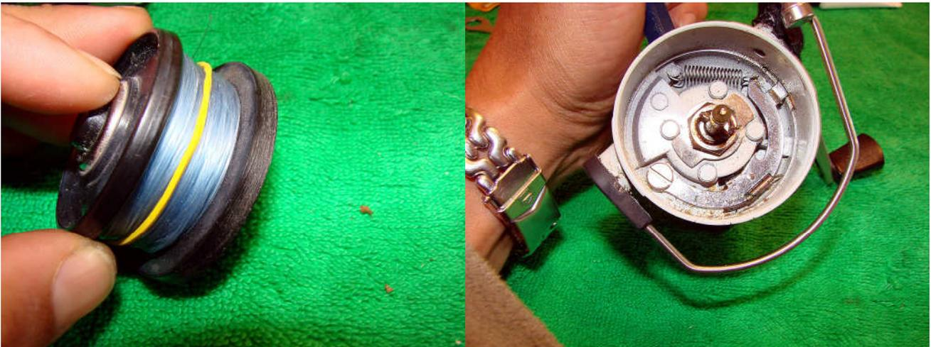
When the spool was removed it looked like it had been rubbing on the inside of the rotor housing-this would suggest that the main shaft may be off true. A service will reveal any problems.
