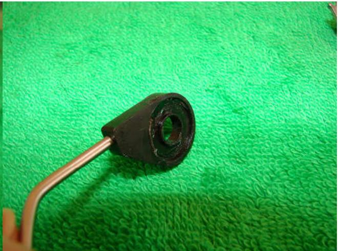
Replace the other bail spring (add a light coat of grease). Add a light coat of grease to the friction surfaces and fix in place with the remaining bail screw.
