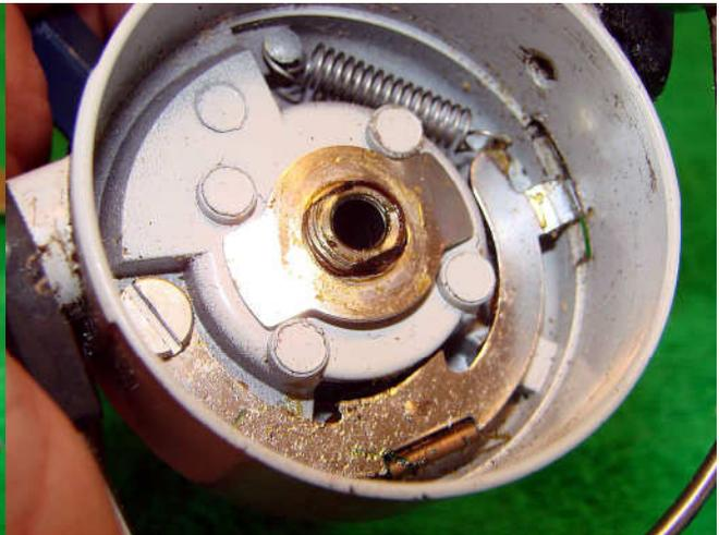
To remove the rotor unscrew the rotor nut and remove this along with the locking washer.
