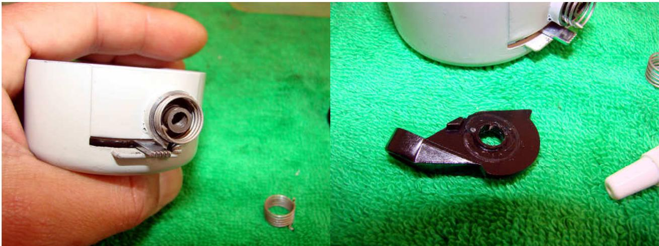
Replace the bail spring and bail arm adding a light coat of grease to the spring and all friction surfaces.
