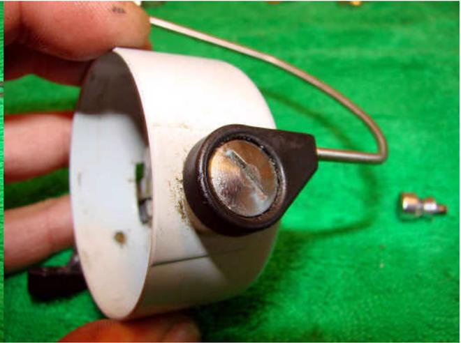
Bail wire, 'roller' (on this reel is does not roll), and bail nut. Unscrew the bail screw.
