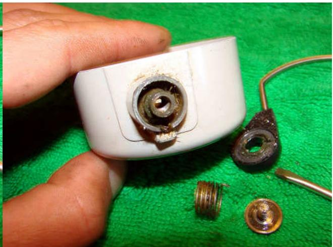
Remove the bail screw, bail attachment and the bail spring. Note that the two bail springs are different-do not mix them up.
