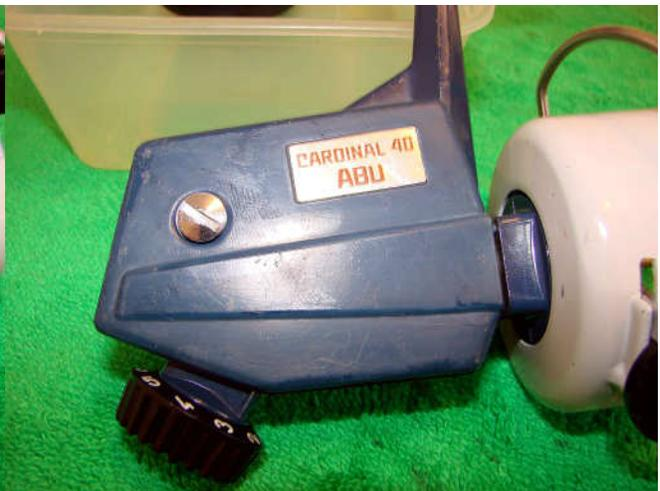
Replace the link arm making sure that there is grease where it contacts the main gear. Replace the side plate.
