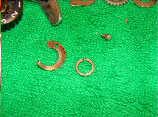
The drag knob spring is showing some corrosion so it will be removed and cleaned up-just the one screw to undo. Note the copper washer that sits between the reel body and the drag knob.
