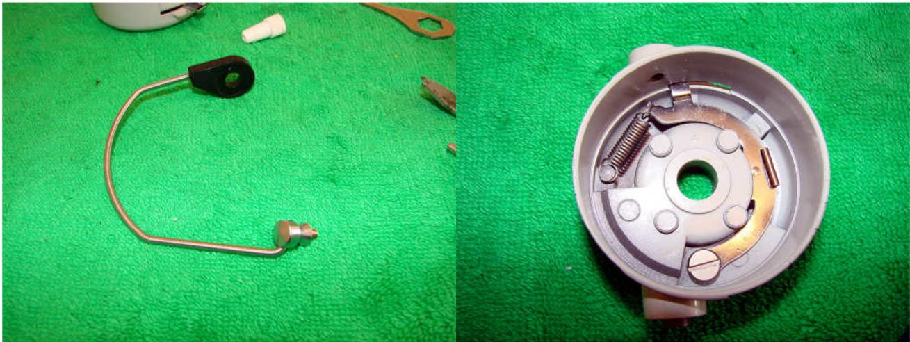
Add grease to the threads and replace the line roller. Replace the trip lever and spring adding a light coat of grease to the friction surfaces.
