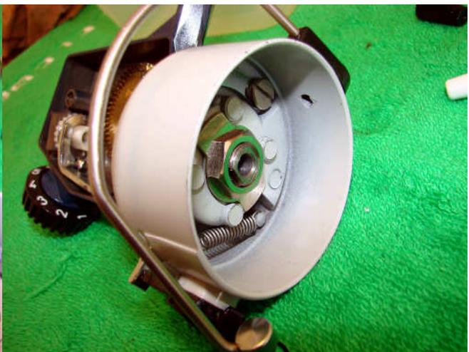
Add a dab of grease where the trip lever will contact and then replace the entire rotor assembly and fix in place with the locking washer and nut.
