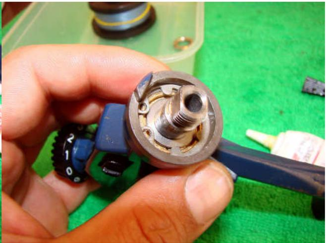
Replace in the reel body and fix in place with the circlip.
