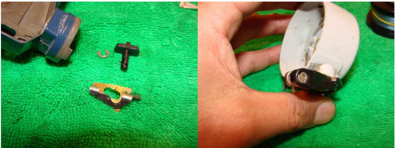
It shouldn't be necessary to disassemble the AR assembly though it only involves removing the circlip on the AR knob; the AR knob can then be removed from the other side of the body. Note how the parts fit together. Remove the bail wire by unscrewing the bail nut.
