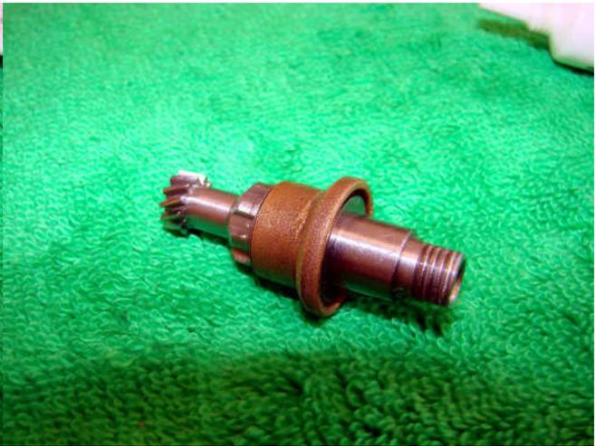
Flood the bushing for the pinion gear with oil then remove the excess. Replace the small washer, the bushing and then the large washer. You can add a light coating of grease to the outside of the bushing.
