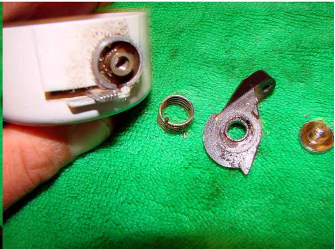
Unscrew the bail screw and remove the bail arm and bail spring. Both bail springs seem to be ok-just very gummed up with old dried on grease.
