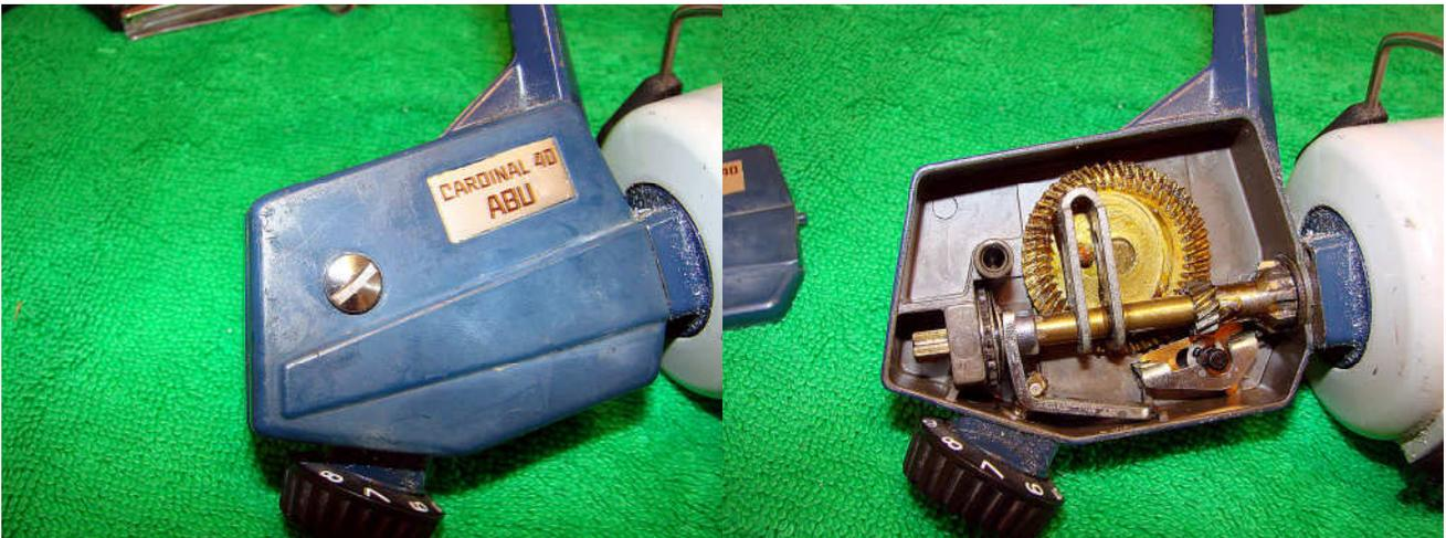
Firstly remove the handle by winding backwards, and then remove the side plate-just one screw.
