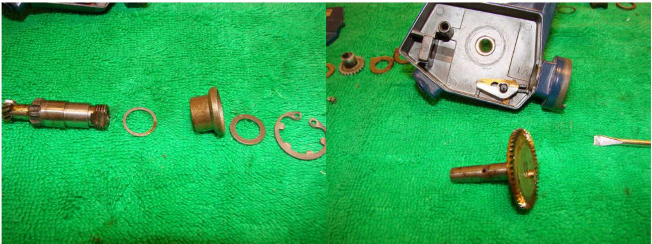
Everything is laid out in order here from left to right; pinion gear, small washer, bushing, large washer, circlip. The main gear simply pulls out of the reel body.
