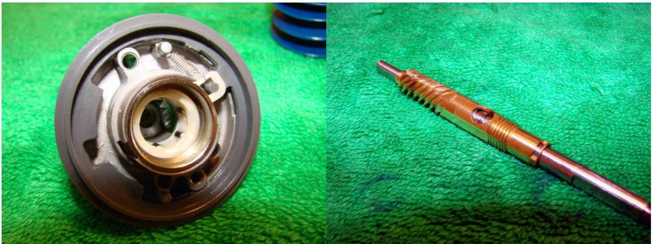
Replace the stopper lever ensuring that the pin stays in place. Snug down the sleeve and replace the spring. Smear liquid grease on the main shaft and grooves for the pawl and then replace in the pinion.
