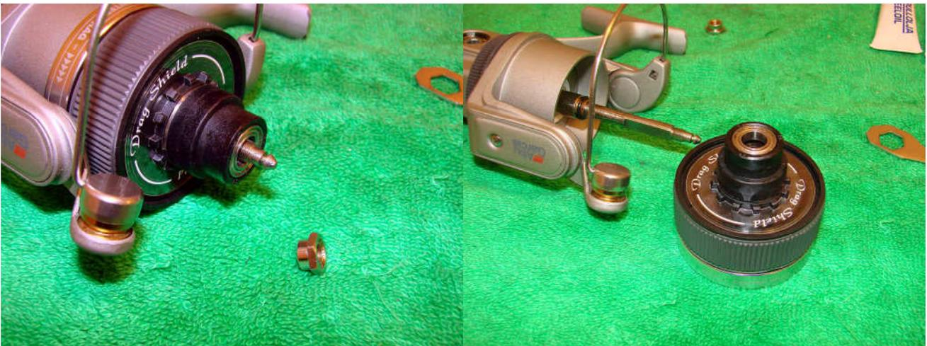
Remove the spool and undo the nut holding on the centre drag assembly. Put the drag assembly to one side as we do the rest of the reel.
