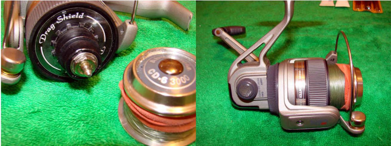
Replace the whole drag assembly back on the main shaft ensuring that it is seated properly. Replace the nut and spool.
