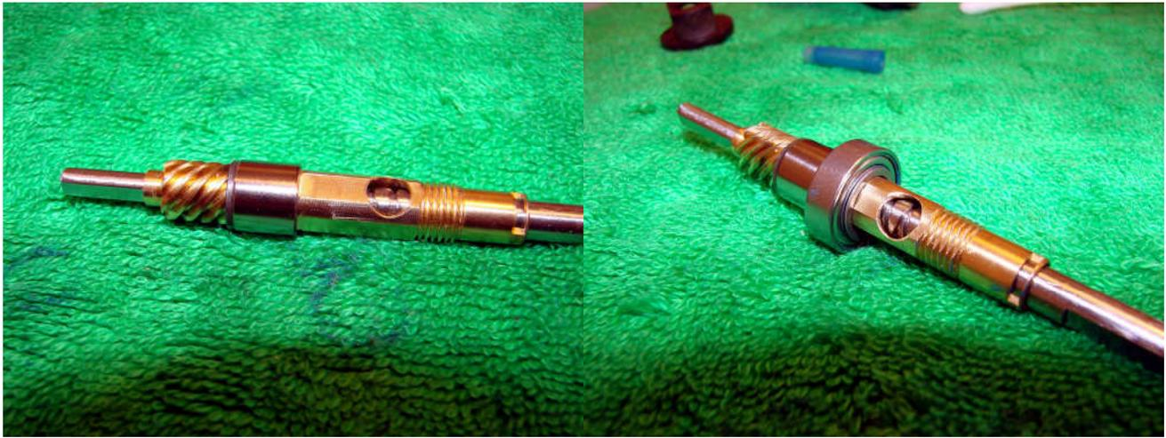
Replace the washer, the sleeve, and then the bearing. Add some grease to the pinion teeth.
