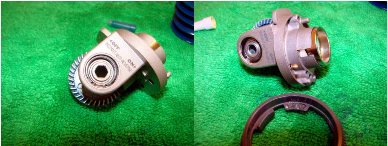
Replace the bearings and retaining clips. Pull the sleeve up slightly so that the stopper lever can be replaced. Smear some grease where the pin contacts.
