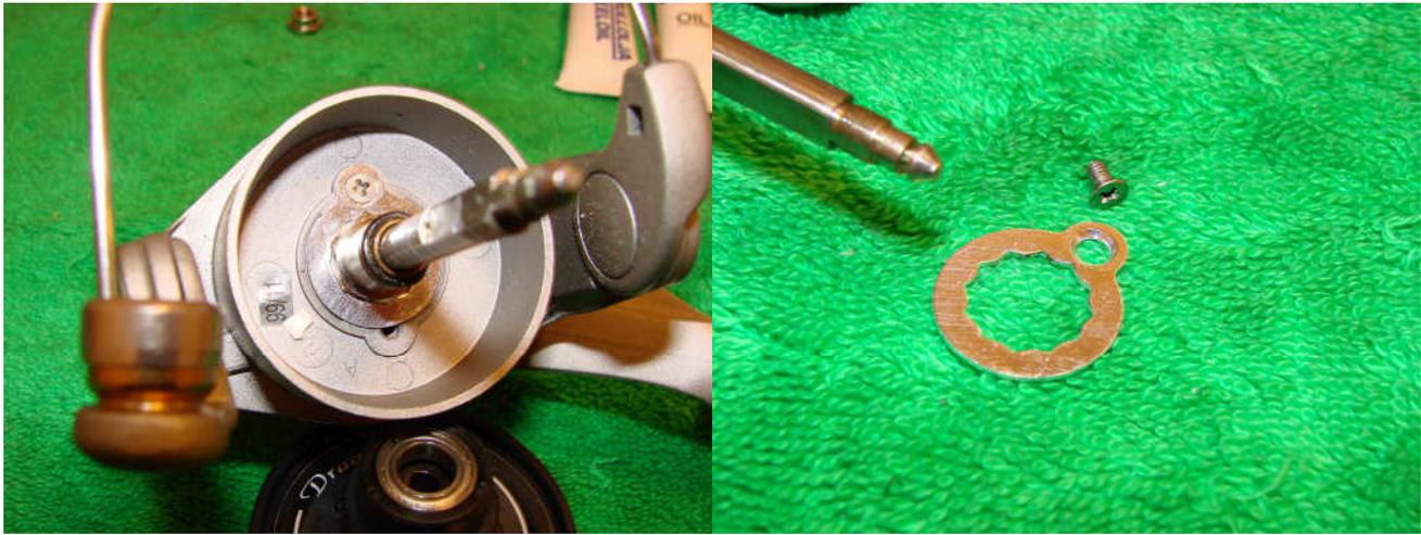
Remove the rotor nut lock plate screw and the rotor nut lock plate.
