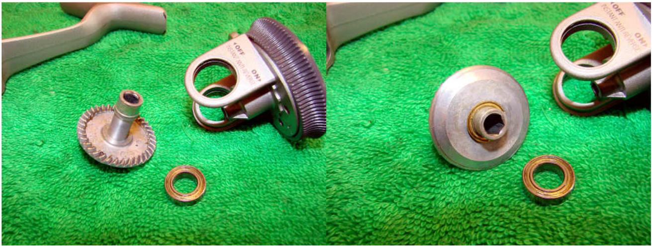
Remove the drive gear from the gear box-it looks like there is no grease here. Note the washer on the other side of the drive gear.
