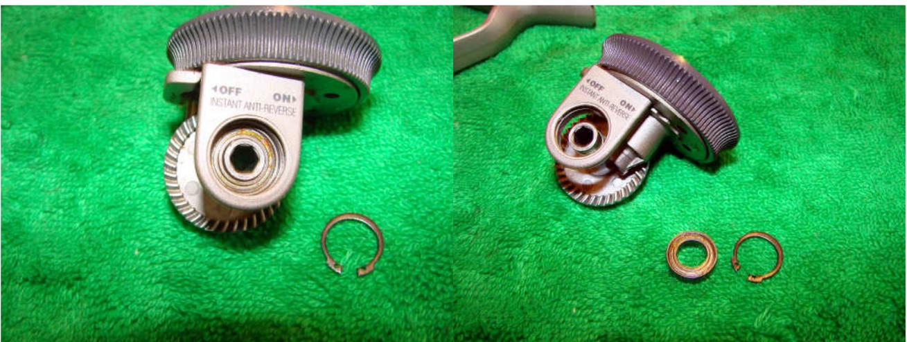
Remove the circlip holding the bearing in place and then remove the bearing. Do the same for the other side.
