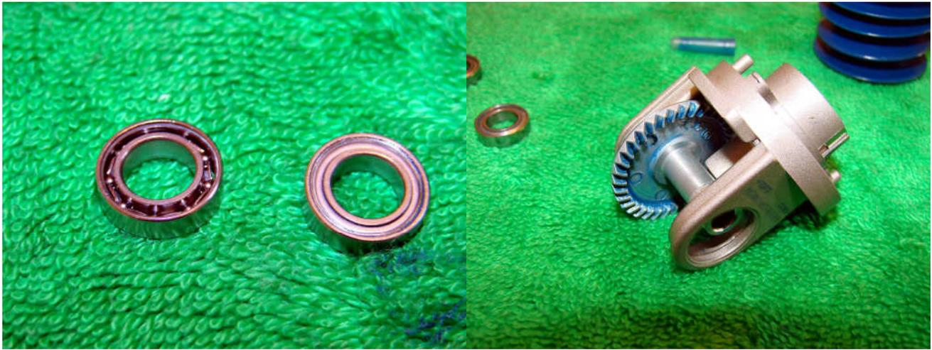
Pack the bearings with your lubricant of choice. I found grease alone to be a bit too thick so I used a mixture of oil and grease. Replace the shields and retaining clips. Put grease on the main gear and place back in the gear box. Don't forget the washer on the other side of the main gear.
