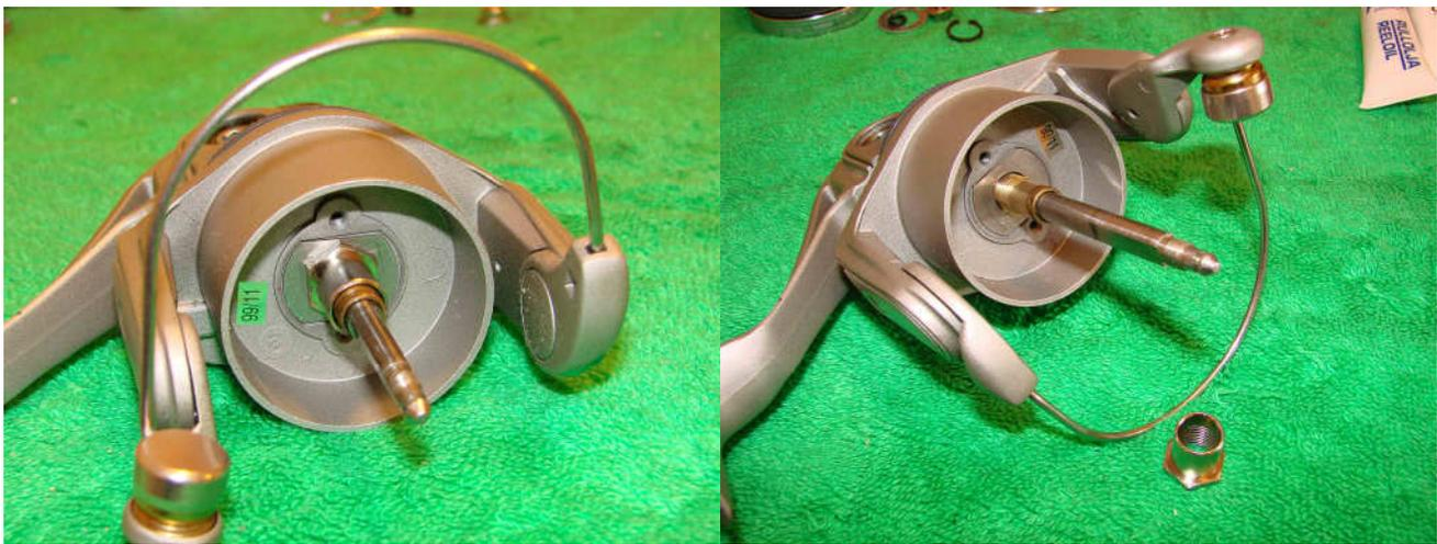
Remove the o-ring and undo the rotor nut.
