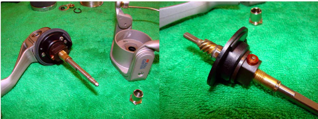
The rotor will lift off. Remove the four screws holding on the flange cover and remove the whole assembly.
