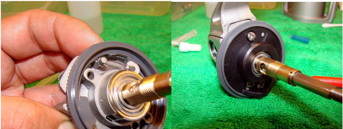
Replace the main shaft assembly back in the gear box. Slide the gear box into the reel body, make sure that everything is seated properly, replace the flange cover and then replace the four screws.
