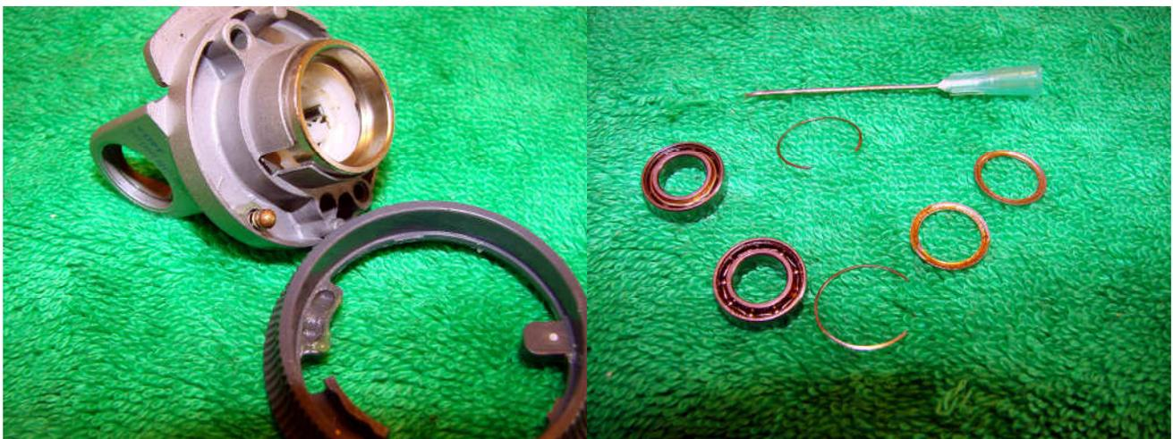
Make sure that you don't lose the stopper and spring-it sits in the gear box. Clean everything before reassembly. Shields can be removed from the bearings to clean out old grease.
