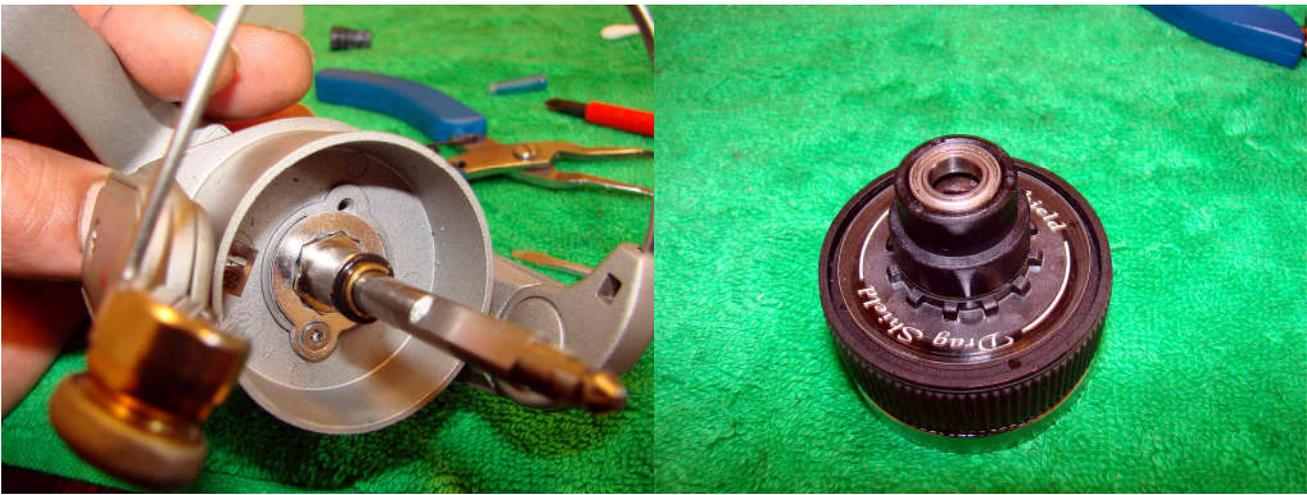
Replace the rotor nut, rotor nut lock plate, the lock plate screw and the o-ring. Put the reel to one side as we give the drag assembly a service.
