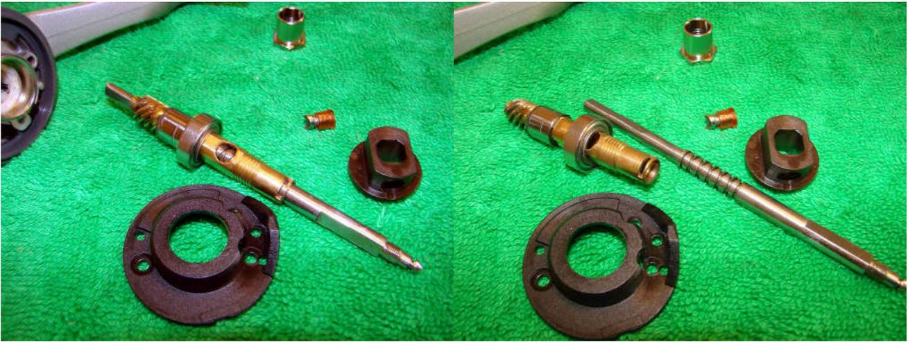
Remove the pawl, pawl holder and the flange cover. The main shaft can be removed from the pinion gear.
