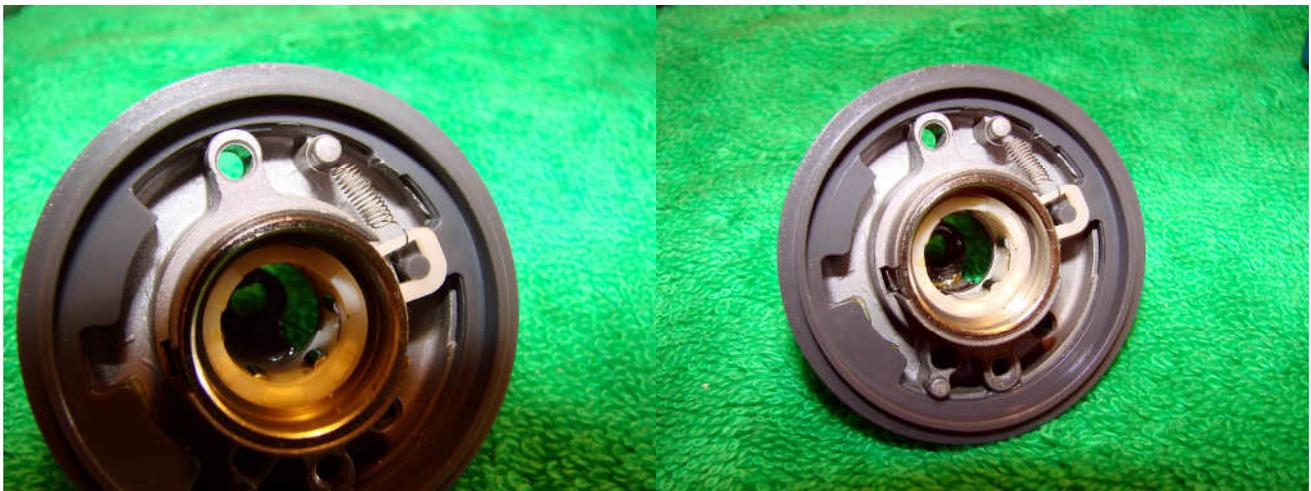
Remove the spring and slide out the sleeve just enough so that the clutch lever can be raised to allow the stopper lever to be removed. Clean the rollers on the one way bearing with a cotton bud soaked in lighter fuel. When completely dry run a bud with a drop of oil on it around the rollers. Do NOT over lubricate the one way bearing.
