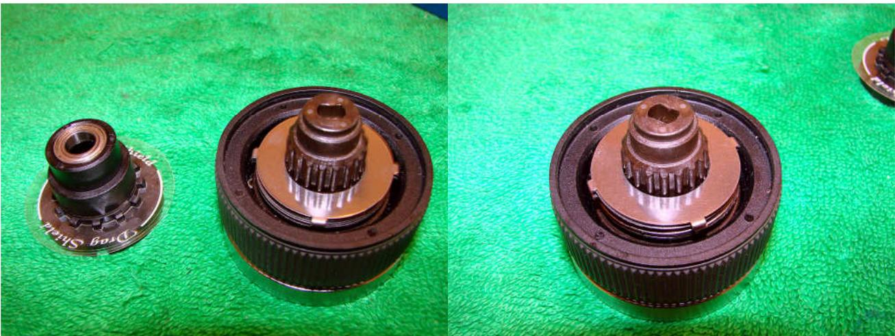
Remove the upper spool bushing (contains the bearing and drag shield). Close inspection of the drag assembly shows that the washers are not in the correct sequence.
