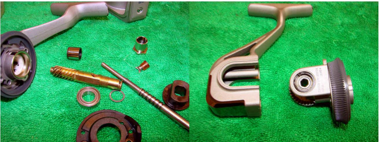
You can then remove the bearing, sleeve and washer. The gear box slides out of the body.
