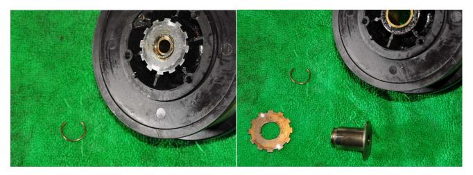
Turn the spool over and remove the c-clip holding the anti reverse gear and spool bushing in place. Give everything a thorough clean before reassembling.
