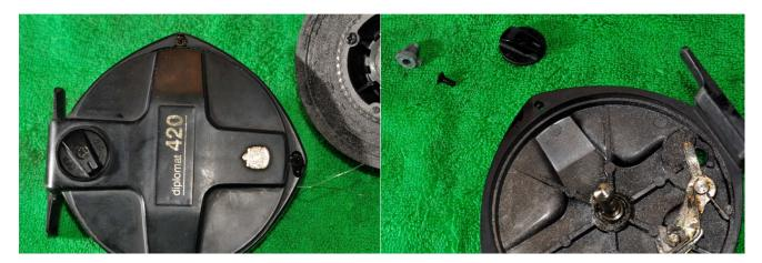
The screws are seized so soak them in oil before attempting to remove them. Remove the screw for the click button and remove whole assembly.
