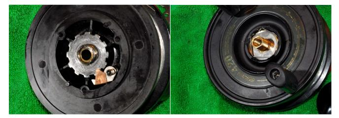
Replace the spool bushing, anti-reverse gear and anti-reverse pawl and fix in place with the c-clip. Give the spool bushing a light coat of oil. Give a light coat of grease to the anti-reverse gear and make sure that the 'ears' on the anti-reverse pawl are gripping the gear. Replace the drag stack and fix in place with the retaining clip.
