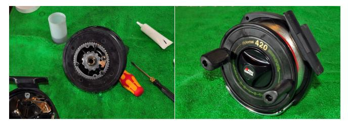
The on/off clicker mechanism was not working properly as the clicker cog had worn down. Ideally this part needs to be replaced. As a quick fix, until a new part is ordered, the clicker cog has been turned over so at least it's functional.
