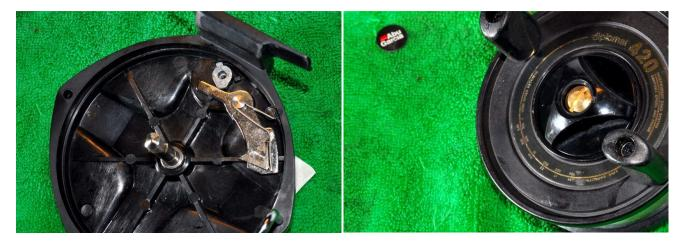
The inside of the reel body needs a thorough clean to remove the metal dust. Reinstall the clicker mechanism adding a light coat of grease to all friction surfaces. Remove the cover for the drag knob-it can be carefully pried out. Remove the brass screw under the cover.
