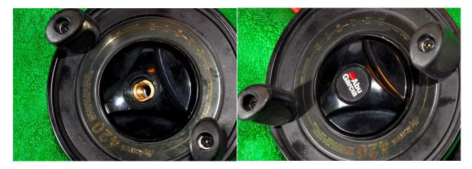
Replace the spool knob and brass screw (remembering to grease the threads), and then pop the screw cover back in place-it should 'click' in. Add a couple of drops of oil to the handles.
