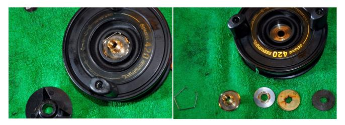
The drag knob lifts off. Remove the retaining clip for the drag assembly and then remove the drag washers. They are laid out top to bottom (left to right).
