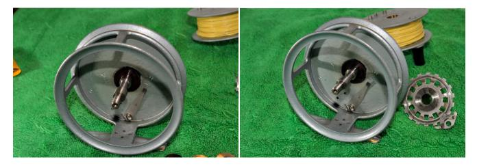
Lightly grease the fibre washer at the base of the spool shaft with drag grease. Add oil to the spool shaft. Note that the reel can be configured to be other left or right hand retrieve, I assume V is left and H is right in Swedish. If you wish to retrieve with the left hand move the spring on the reel body to V or L-with the right then leave it at H or R.
