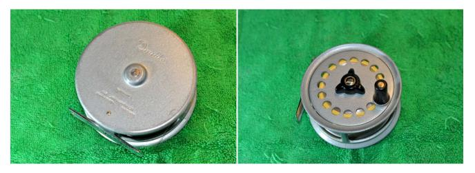
This reel is in lovely condition and appears to have no mechanical issues. Firstly remove the screw in the centre of the drag knob.
