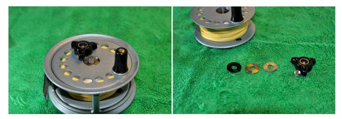
Unscrew the drag knob and then remove the spool. Note that there are three washers in the spool. They are laid out left to right = bottom to top (the fibre washer is on the bottom, curved metal washer on the top).
