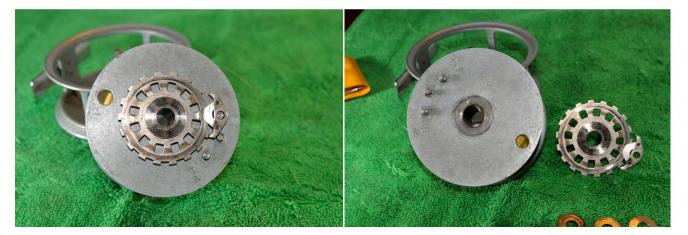
Remove the click wheel assembly from the spool-it simply lifts out. The anti reverse dog can be removed from the click wheel.
