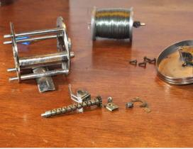
The level wind assembly removes in typical ABU fashion; retaining clip on right side plate, screw to remove pawl, and the whole assembly being removed from the right side of the frame.
