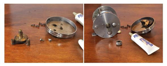
Three bridge screws hold the bridge assembly and gears in place on the right side plate; the gears simply lift off the bridge assembly.
