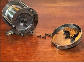
Start by removing the handle and then remove the four pillar screws holding the right side plate on to the frame, the spool can be removed from the frame.
