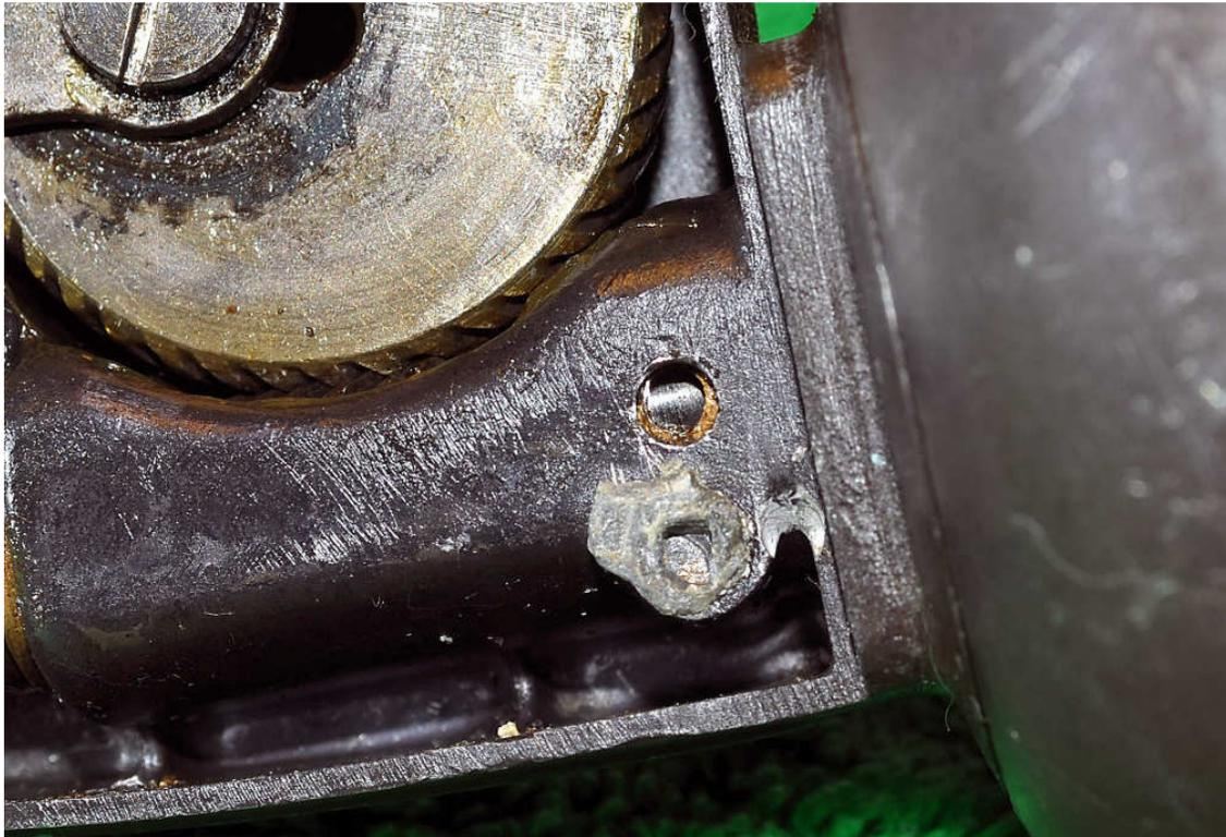
A closer look shows that someone has already tried to drill out a screw and made a bit of a mess. Note the oil port above the mangled screw-use this to lubricate the pinion gear.
