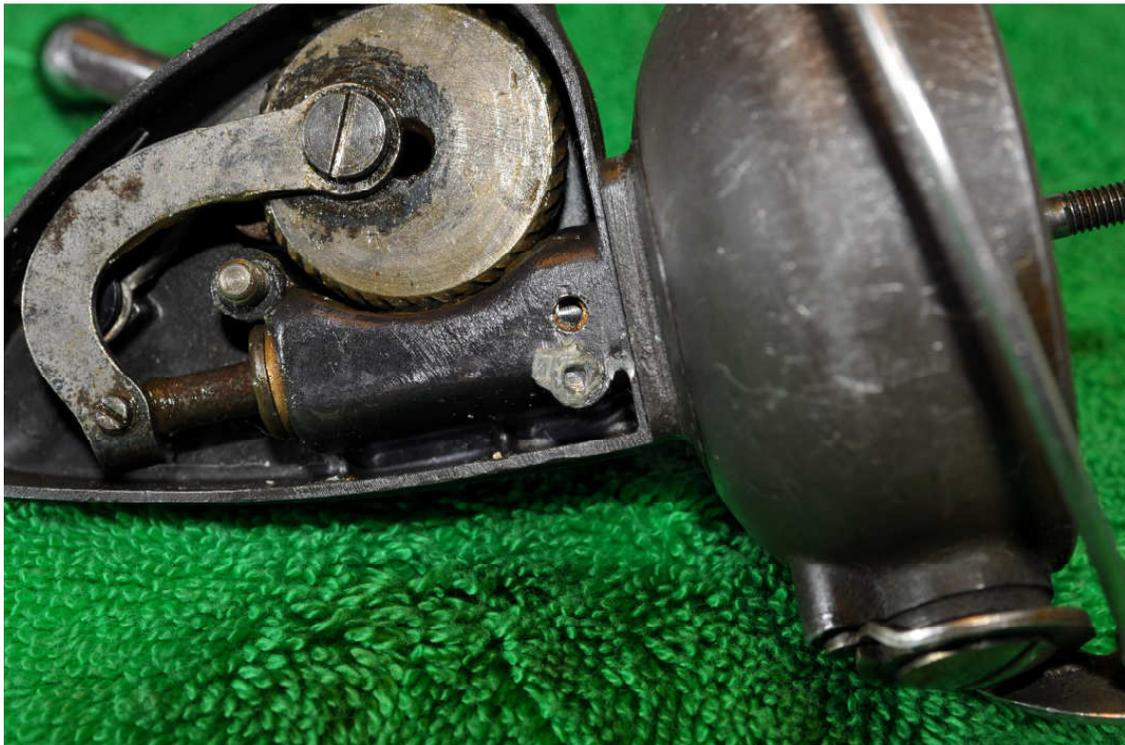
It should be a simple matter of undoing the screws holding the oscillating arm to the main gear and to the end of the main shaft.
