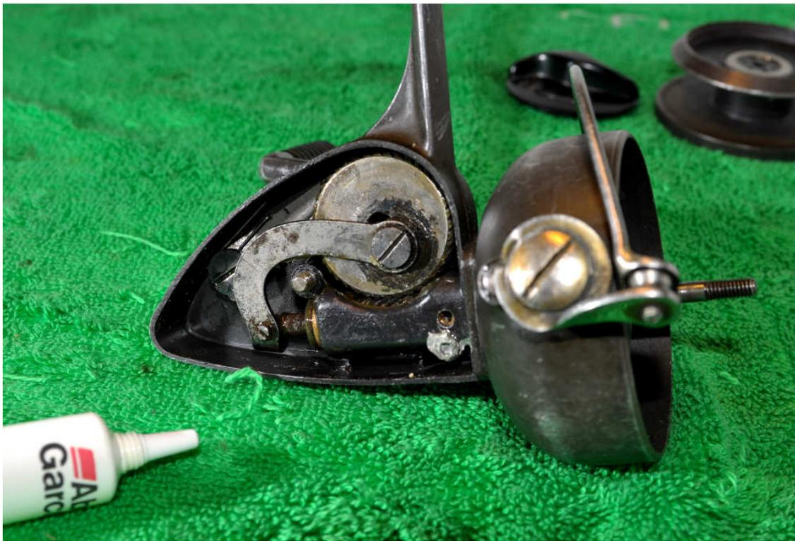
Apply a light coat of grease to the gear teeth and where the oscillating arm contacts the main gear, and oil to the main shaft and oil port on the pinion gear casing. Replace the side plate. The reel works fine and as it is an original display reel it is not worth risking further damage, assuming you could get original ABU parts for it.
