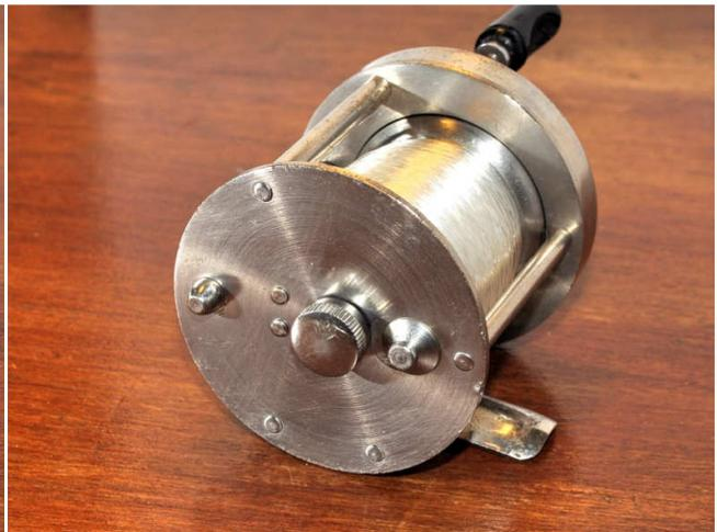
Before reassembly give everything a thorough clean. Add grease to the gears and all screw threads (to stop them seizing), and a light oil to all other friction surfaces.
