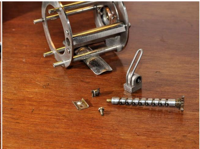
The level wind assembly removes in typical ABU fashion; remove the retaining clip on the right side of the frame, undo the pawl cover and remove the pawl, and then the whole assembly can be removed from the right hand side of the frame.
