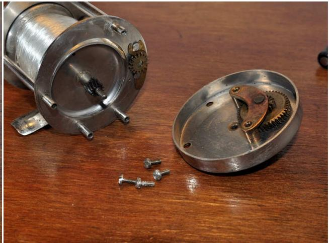
Remove the handle nut and handle. Undo the four pillar screws and remove the side plate from the frame.
