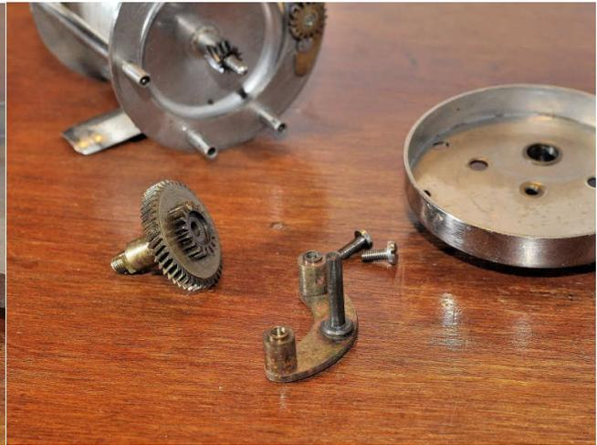
The bridge assembly can then be removed from the side plate. The main gear simply lifts off the bridge assembly.
