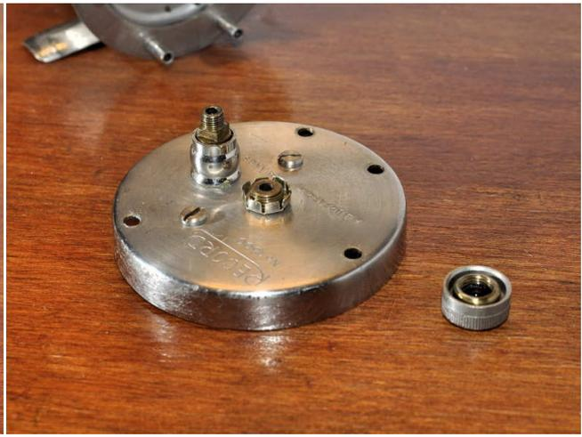
Remove both screw caps and add a drop of oil. Remove the two bridge screws on the right side plate.
