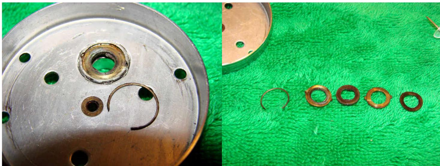
The washers can then be removed. The order here is left to right =bottom to top (I have called the washers with 'ears' keyed washers). Split ring, keyed washer/fibre washer/keyed washer/spring washer. The fibre washer that sits on the main gear is not shown.
