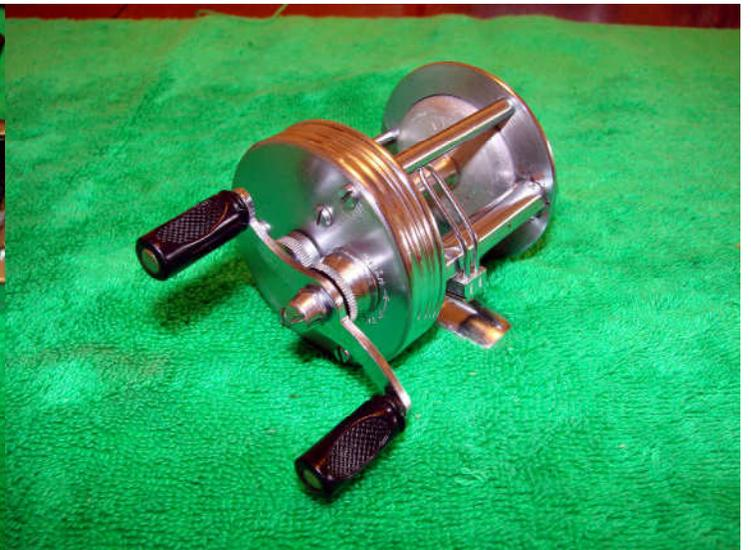
Place the spool back in the frame and then reattach the right side plate. Replace the four (greased) pillar screws. Adjust the spool caps so there is barely discernible side to side play i.e. they are lightly touching the ends of the spool shaft.
