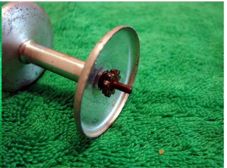
Place the whole bridge assembly back in the side plate and then replace the three bridge screws-remembering to grease the threads! The left side of the spool shaft will need to be cleaned up.
