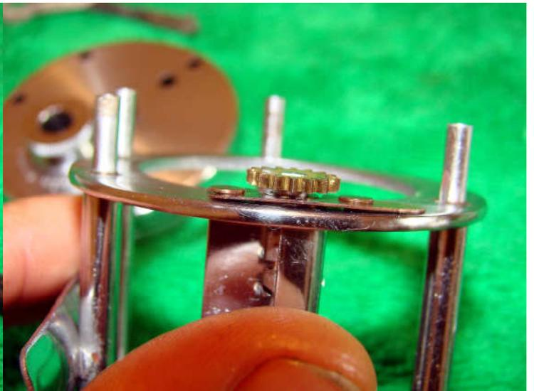
The bushing will need to be pushed flush with the frame before the locking washer can be replaced.
