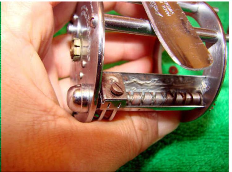
The locking washer for the worm gear-the design hasn't changed on present day Ambassadeurs. To remove the line carriage (level wind), first unscrew the screw holding on the plate at the base of the level wind.
