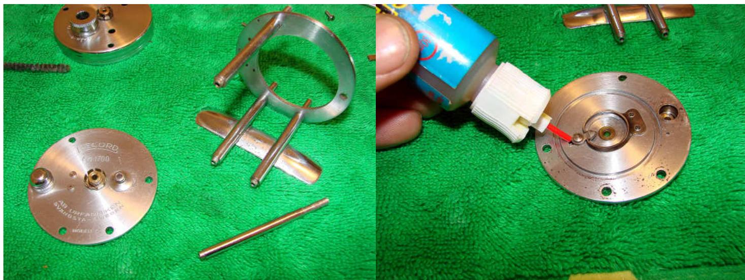
Note that one of the frame bars is not attached to the frame. Add a drop of liquid grease to the clicker assembly-if you work the clicker button backwards and forwards (other side of side plate) it will ensure proper coverage. Add a drop of grease to both sides of the click hammer where it contacts the click spring.
