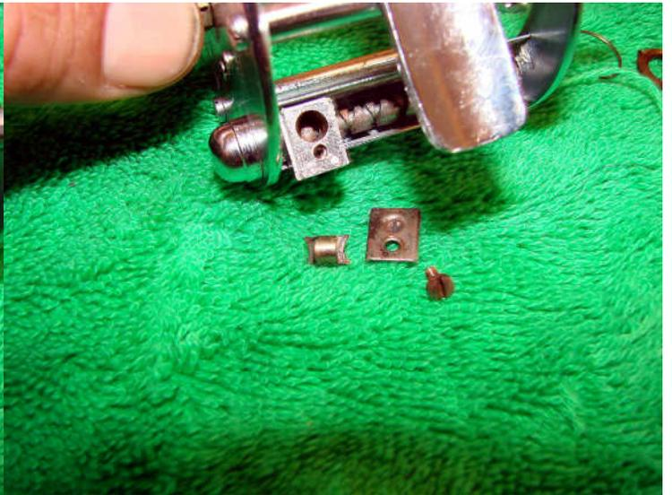
Remove the plate for access to the pawl, this can be removed with a pair of tweezers. Note it is 'double ended'-when one side wears out you simply flip it over-ingenious!
