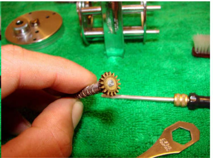
The gear cog on the end of the worm gear pulls off. Remove the bushing and place liquid grease where it contacts the worm gear. Replace the bushing and then press the cog back on to the worm gear so it is a snug fit.
