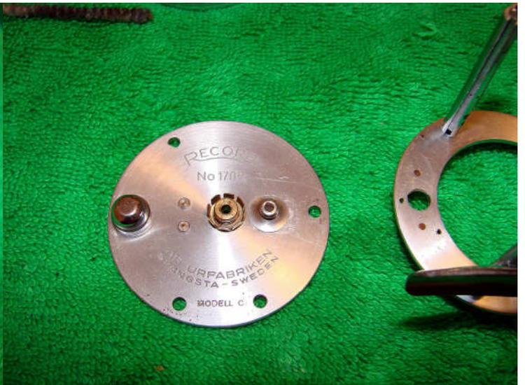
Slide off the locking washer-the worm gear can then be removed from the side of the frame. If you remove the four screws holding on the left side plate this lifts off. The worm cover can then be removed.
