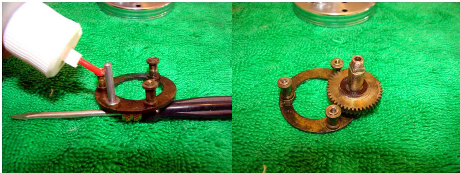
Smear some liquid grease on the post for the main gear ensuring complete coverage and then replace the main gear. Add a light coating of drag grease to the fibre washer before replacing on top of the main gear. Add a light smear of grease to the three posts on the bridge where they contact the side plate.
