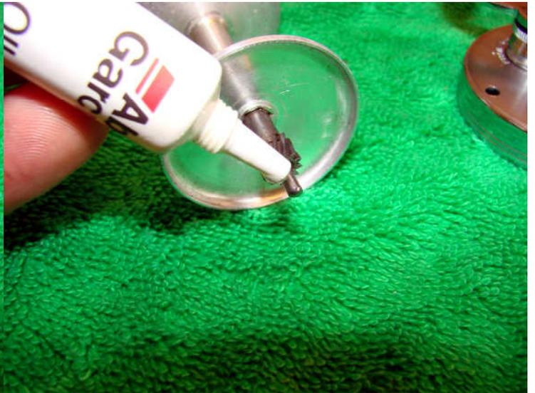
As will the right side. When clean add a drop of oil to the shaft where it contacts in the side plate (both sides), and some grease to the pinion gear.
