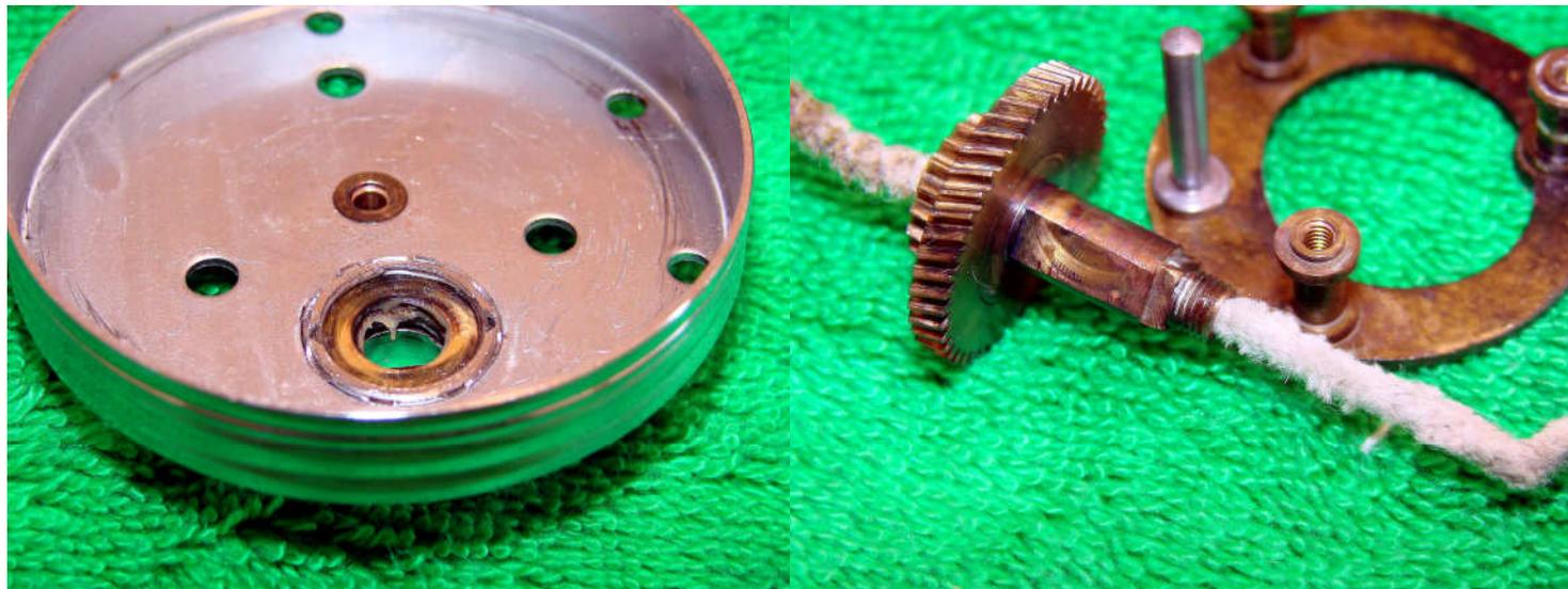
Lightly coat the washers with drag grease and replace in the right side plate making sure that the retaining clip is seated fully. In this photo there is actually a lot of grease! A pipe cleaner dipped in lighter fuel is great for cleaning the inside of the main gear.
