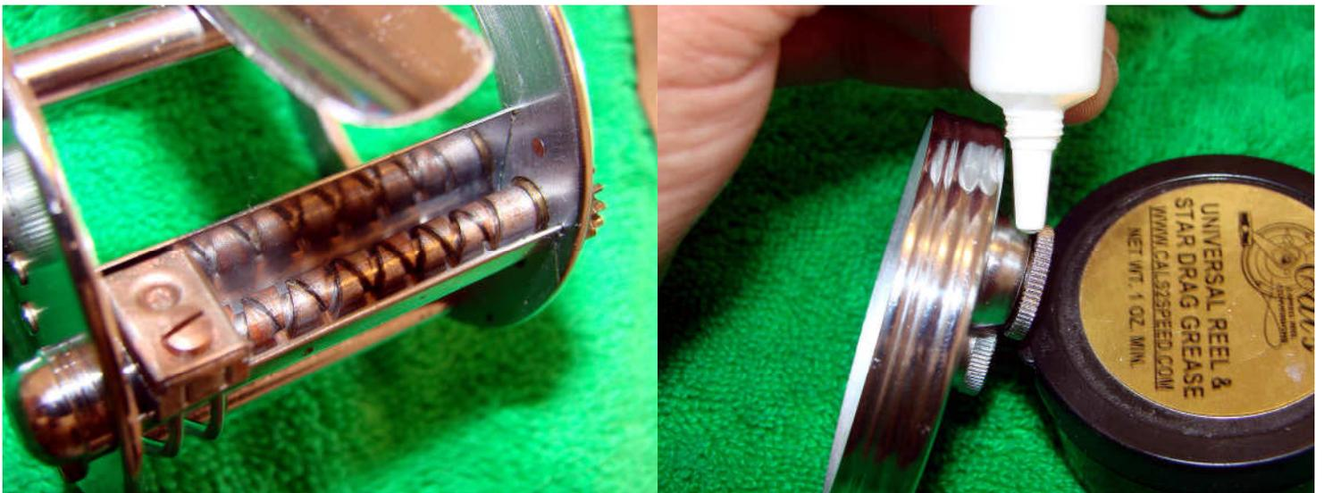
Place liquid grease on the entire worm gear-not just in the threads-the level wind is supported by the worm gear (unlike modern Ambassadeurs where it is supported by the worm gear cover). Add a drop of oil or liquid grease to the base of the crank ring (?) when it is fully screwed out. Screw it in and out a few times to ensure proper coverage.
