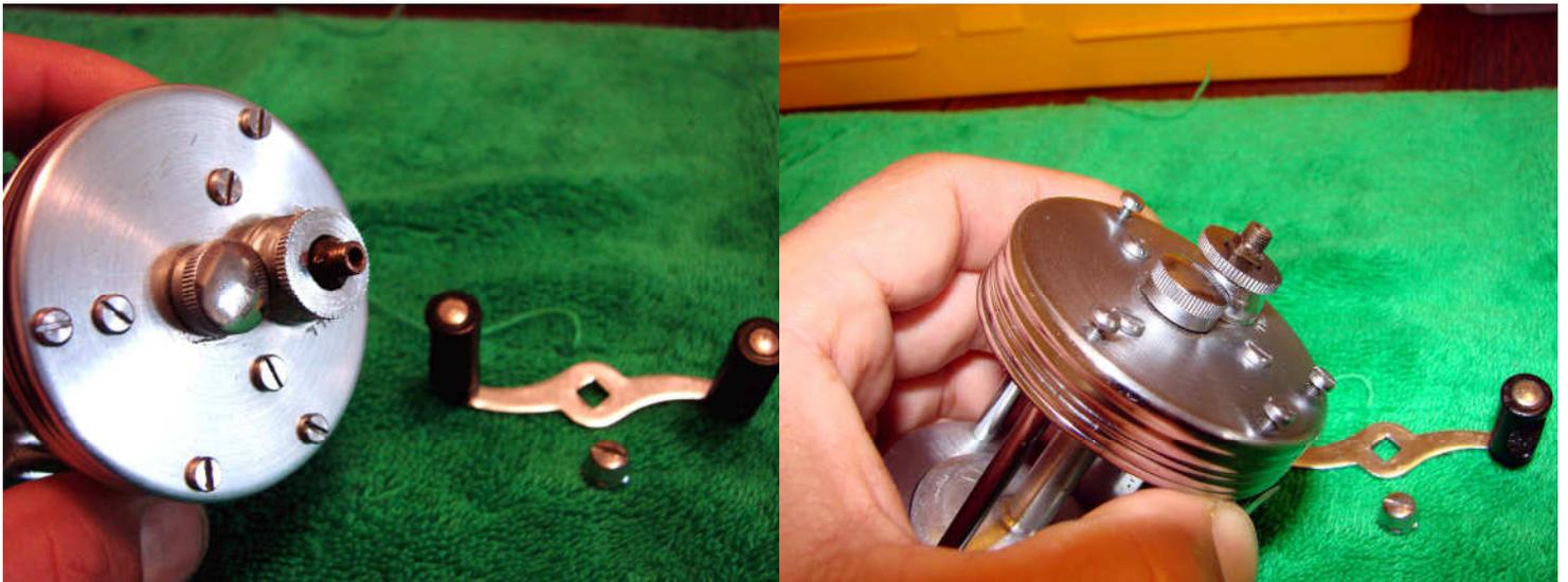
Starting on the right side plate (called head cap on the schematic), remove the handle nut and the handle. Undo the four pillar screws holding the side plate to the frame-the importance of having properly fitting screwdrivers cannot be overstated. Nothing makes a reel look old quickly as mangled screw slots. It is nice to note that the threads on these screws are greased.
