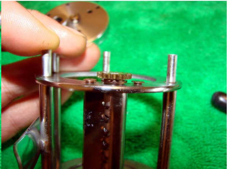
Place the level wind so that it sits in the left side plate-this makes it easier when replacing the worm gear. Note in the above picture that the bushing is not yet flush with the frame.
