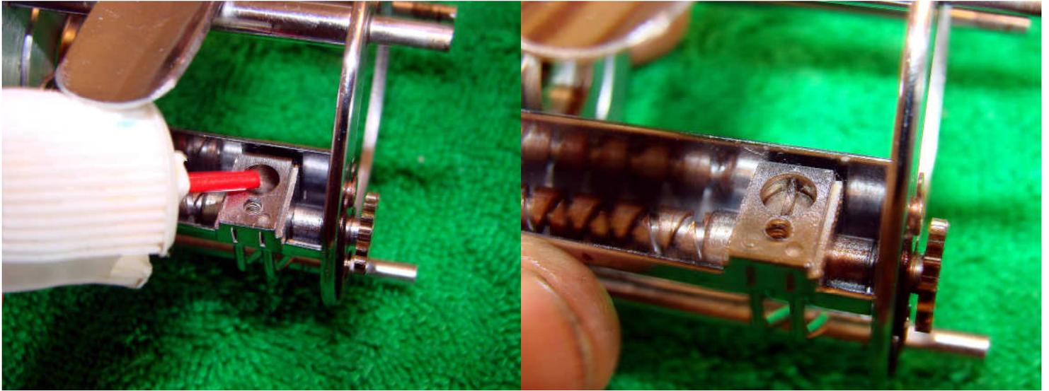
Add a drop of oil or liquid grease to the inside of the level wind before replacing the pawl. Make sure that it seats properly in the grooves on the worm gear-do not force!
