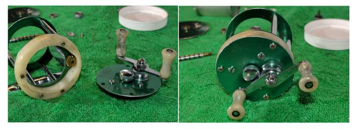
Add a drop of oil to the shaft of the worm drive gear and then replace it in the frame. Replace the plastic side plate spacer and then replace the side plate-not forgetting to grease the screw threads. Reattach the worm gear and the level wind in the frame. Add a few drops of oil to the worm gear where the pawl sits and also to the shaft where it contacts the frame.
