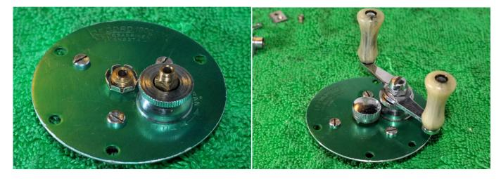
Replace the bridge gear assembly on the side plate and fix in place with the three bridge screws (don't forget to grease the threads). Replace the handle and handle nut. Add a drop of oil to the felt washer in the spool cap and replace it on the side plate.
