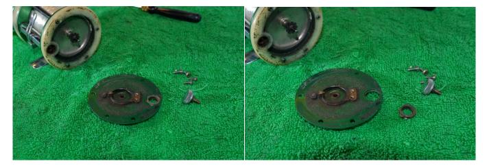
Remove the side plate and the plastic side plate spacer. Note the bushing for the end of the worm gear-this is not fixed to the side plate.
