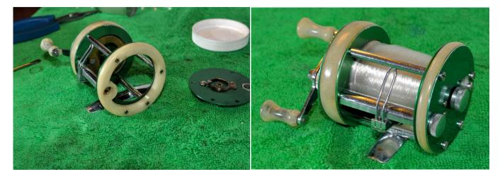
Add a drop of oil to the ends of the spool shaft and then replace in the frame. Replace the plastic side plate spacer and then fix the side plate in space with the four pillar screws (you can add a drop of oil to the clicker before replacing). Replace the thumbscrew for the worm gear.
