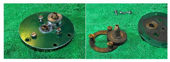
Remove the spool cap. Remove the three bridge screws and then remove the entire bridge/gear assembly from the side plate. Note the fibre washer on top of the main gear.
