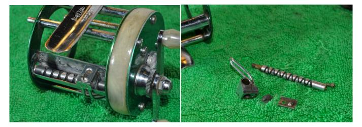
Remove the screw and cover from the bottom of the level wind. The pawl can be removed from the level wind, and the level wind and worm gear removed from the frame.
