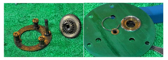
The main gear lifts off the bridge assembly-note the idler gear is under the main gear. A clip holds the drag washers in place in the side plate. Carefully remove this and then remove the drag washers.
