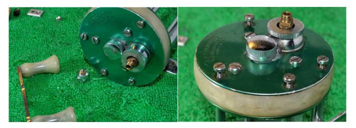
Remove the handle nut and handle. Remove the four pillar screws on the right side plate.
