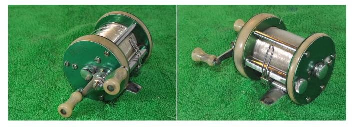
On the outside this is a very clean reel. Unfortunately the colour is the same as the background but the photos should be clear! Remove the thumbscrew for the worm cover and the four pillar screws holding on the left side plate.
