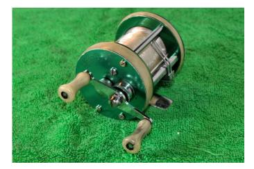
Add a couple of drops to the handle knobs and you're finished.
