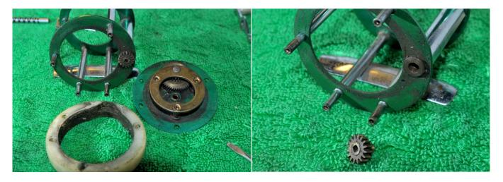
Remove the side plate and plastic spacer ring. The metal gear for driving the worm gear simply lifts from the frame.
