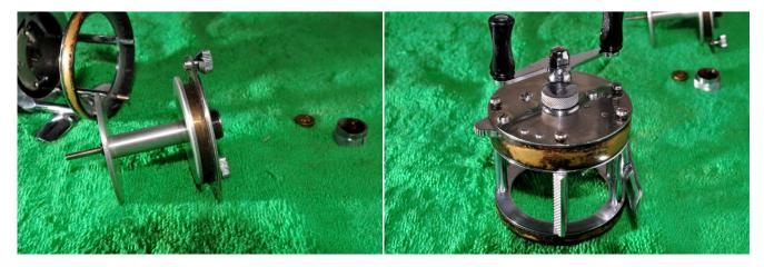
The spool was stuck firm. As this is a display reel the spool was left as is-it worked fine and removal may have caused some damage to the reel. In this instance a couple of drops of oil were added to the bearing and the spool cap was replaced.
