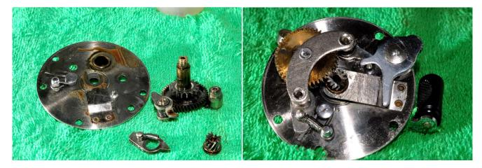
You can now remove the whole gear bridge assembly and the pinion gear. Give everything a thorough clean before reassembly.
