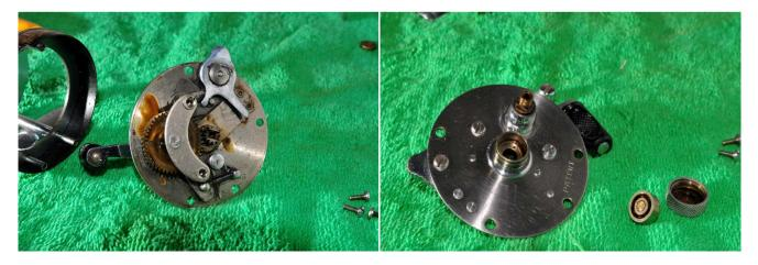
Lift off the whole plate assembly. Remove the spool cap and bearing, and the handle nut and handle.
