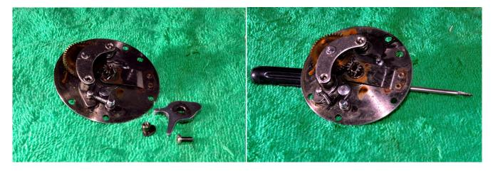
Remove the screw and nut holding on the free spool lever. Remove the spring for the 'anti reverse' dog from the post on the side plate.
