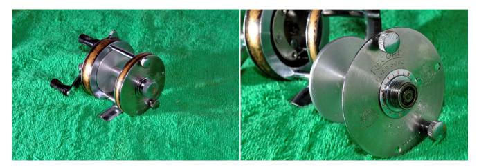
Loosen the thumb nuts and lift off the left side plate. In this reel there was a problem-the spool shaft was stuck to the bearing in the side plate (under the spool cap).
