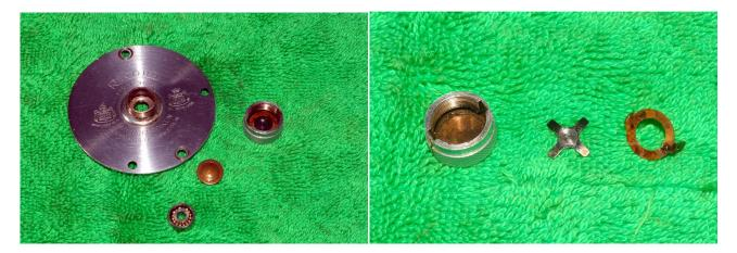
Unscrew the spool cap and remove the bearing shim and the bearing. Give the bearing a thorough clean by soaking in shellite/lighter fuel. When clean and dry add a couple of drops of oil of your choice.
