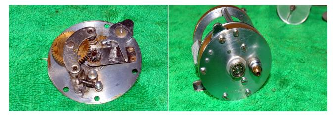
On reassembly apply a light coat of grease to all friction surfaces where there is metal-metal contact. The exception is to the main shaft-apply oil to where it contacts the side plate. Reattach the side plate to the frame and replace the bearing in the plate. Lightly grease the threads for the spool cap. Replace the spool cap (add a drop of oil), and handle and handle nut.
