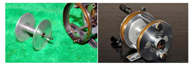
Add some oil to the spool shaft where it contacts the pinion gear and also to both ends where they contact the bearings (to stop them seizing in place as was the case in the Modell C). Replace the spool in the frame and then reattach the left side plate. Using the spool caps centre the spool in the frame so that there is slight side to side 'knock' when in free spool. All done!
