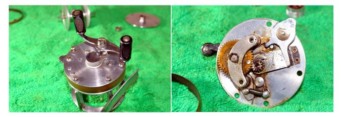
Remove the four post screws and then remove the entire right side plate assembly.
