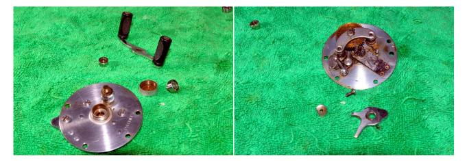
Remove the handle nut and handle, and the spool cap and bearing. Give the bearing a thorough clean (same as the left side plate bearing). Undo the screw and nut holding on the thumb release. At this stage remove the two bridge screws and carefully unhook the anti-reverse spring from the post on the brake plate. Remove the entire main gear assembly from the brake plate and give everything a thorough clean.
