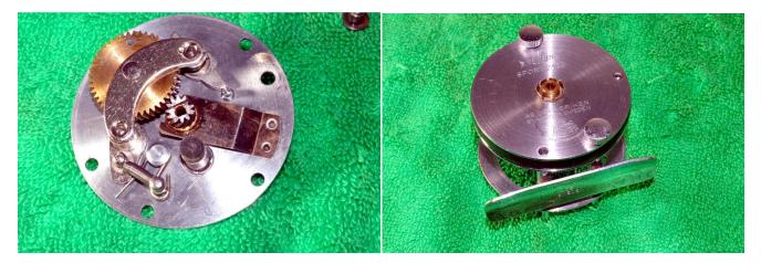
Ensure that the gear teeth have a light coat of grease. Replace the free spool lever and fix in place with the screw and nut. Replace the left side plate and spacer on the frame and then replace the left spool cap.
