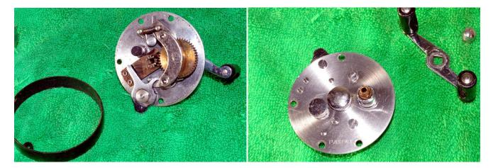
Lift off the whole side plate assembly and black spacer from the frame. Remove the handle nut and handle. Remove the right spool cap and clean it in the same fashion as the left cap. Note that there is another knob/cap on the side plate.
