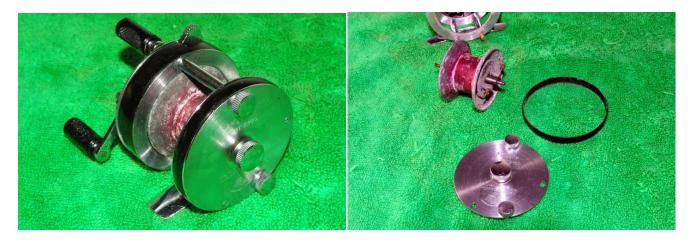
Start by undoing the two thumb screws on the left side plate. Remove the side plate and the plate spacer. The spool can be removed from the frame. Take care not to lose the centrifugal brakes.
