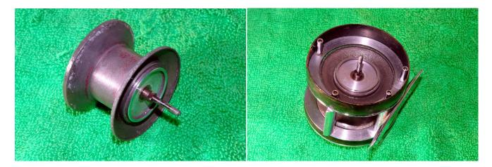
The spool has cleaned up nicely with some warm water and an old toothbrush. Add a drop of oil to the shaft at both ends and also where it contacts the pinion gear. Make sure that the centrifugal brakes are pushed in before replacing it in the frame. Note the metal ring on the spool where the felt washer contacts. This ring was not present in the ABU Sport 2100.
