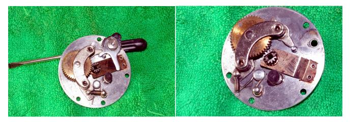
This cap adjusts the height of the felt washer (to the lower right of the pinion gear in the photo). This felt washer rubs against the side of the spool. This could be a casting control (although the reel does have centrifugal brakes) or perhaps a type of drag mechanism.
