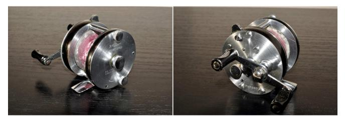
This reel seems to be working fine although the spool is showing some corrosion and salt deposits. The red colour could be colour bleeding from old dacron line.
