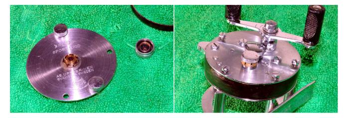
Remove the spool cap. There is a felt washer in it. Carefully remove this and soak in shellite/lighter fuel to remove any dirt. When it is clean and dry replace it in the spool cap and add a couple of drops of light oil. Apply a thin coat of light grease to the threads in the spool cap.
