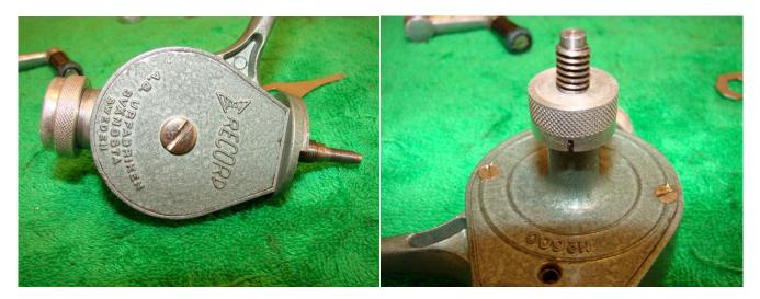
Replace the other side cover and then reattach #5026 ensuring that the wire spring is seated in the groove.
