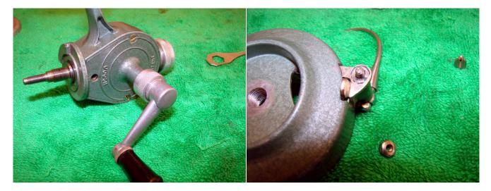
Reattach the handle. Remove the nut holding the bail arm on.
