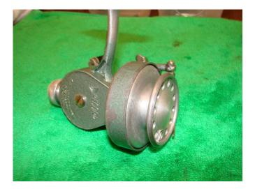
Screw the spool back onto the main shaft and you're finished.
