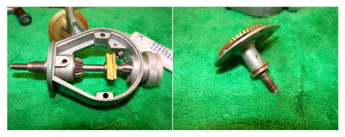
Lightly coat the oscillating slider (#5020) with grease and place it on the main shaft. Add a couple of drops of oil to the shaft of the main gear and replace it in the side plate.
