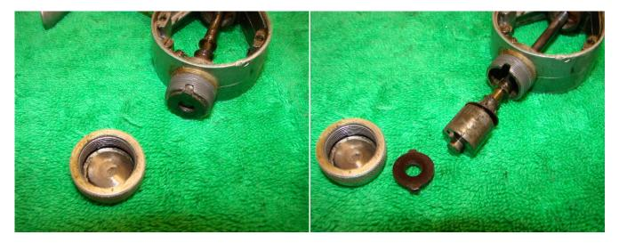
Unscrew the drag knob from the reel body-the entire drag assembly and main shaft can then be removed from the reel body. Note the metal washer in the drag knob.
