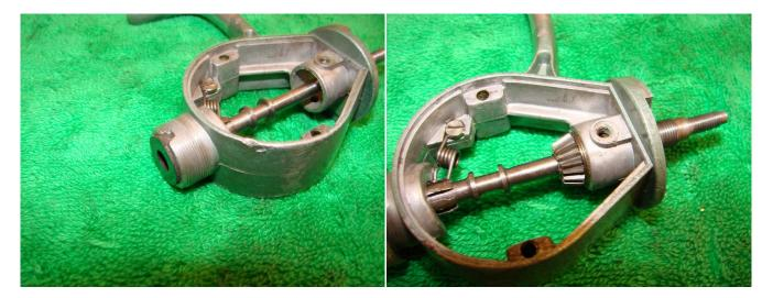
Replace the main shaft in the body (lightly coat the shaft with a drop of oil) and then replace the keyed drag washer (#5015). Add some grease to the threads and replace the drag knob. Add some oil where the pinion sits in its housing and then replace the pinion gear in the reel body. Fix in place with screw #271.
