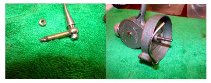
Lightly oil the shaft before replacing. Screw the rotor cup back onto the reel body.
