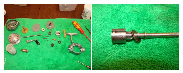
Place the drag washer (#5016) on the rear of the main shaft and then the spacer (#5017) using a light coat of grease.
