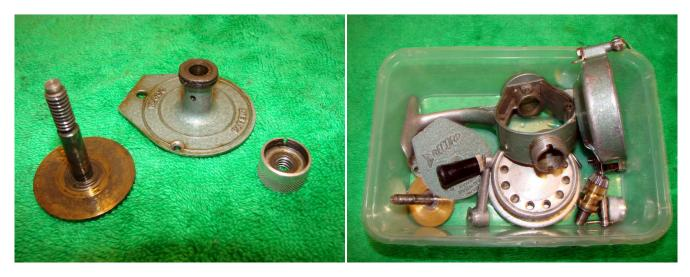
Remove the main gear and #5026 from the side cover. Clean the parts thoroughly before reassembly.
