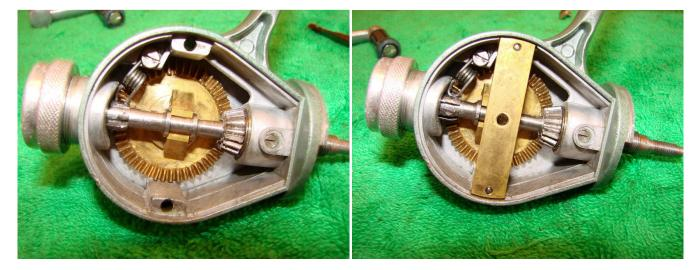
Add a light coat of grease to the gear teeth and where the oscillating slider contacts and then replace the side plate.
