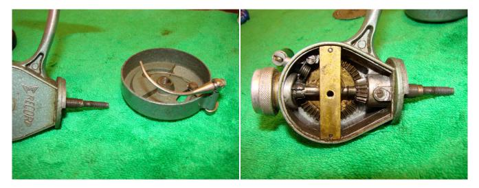
Start by unscrewing the spool and the rotor cup (# 5051). Undo the side cover screw (#278) and then remove the side cover.
