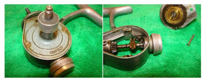
Remove the two side plate screws on the other side and then remove the side plate.
