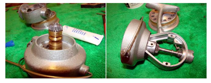
Add a light coating of grease to the pinion gear teeth and then replace the whole rotor assembly onto the reel body.
