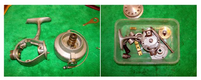
The entire rotor assembly can then be removed from the reel body. Give everything a thorough clean before reassembly. As this is a display reel I'll use very light oil and grease on all friction surfaces before reassembly.
