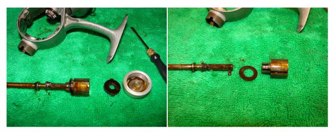
The entire main shaft assembly can then be removed from the rear of the reel frame.
