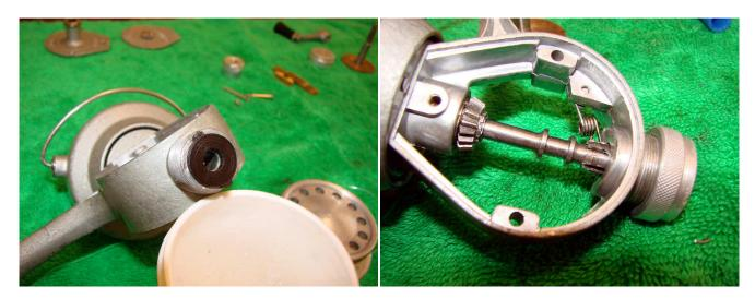
Replace the rear drag washer (#5015) and then replace the drag knob.
