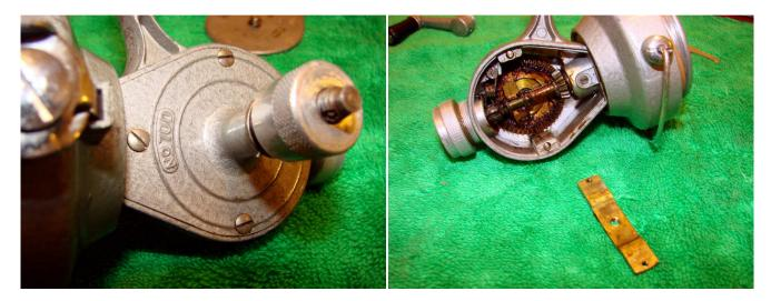
Loosen the two screws (#27)3 on the left side reel cover. Part #5057 can then be removed.
