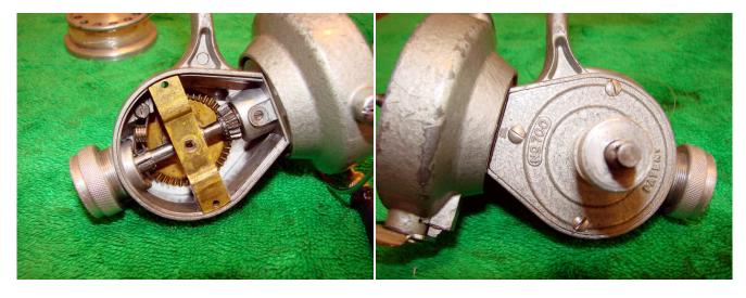
Replace part #5057 and then replace the screws on the left reel plate. Reattach the right hand reel plate.
