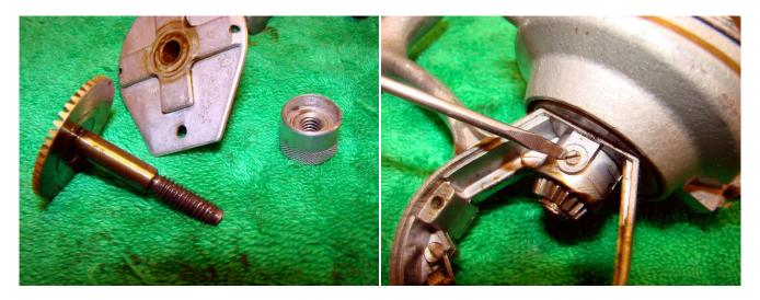
The main gear can then be removed from the side cover. Remove screw (#271).
