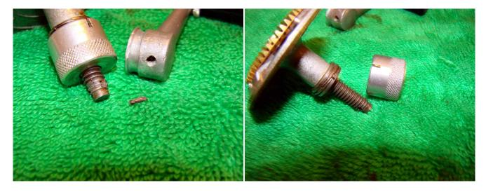
Odd find-someone has drilled a hole through the handle. There was a broken off drill bit stuck in the shaft of the main gear. Remove part # 5026 from the shaft of the main gear.
