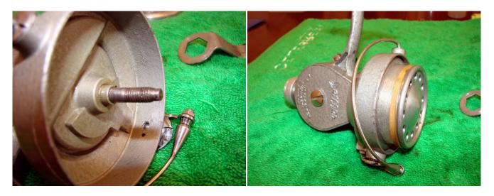
Lightly grease the threads for the spool and then reattach the spool. Reattach the handle and the reel is finished.
