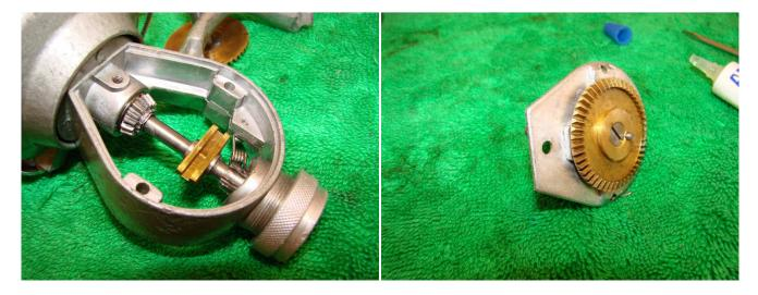
Reaffix the slider (#5020) to the main shaft. Oil the shaft on the main gear and then replace the main gear in the side plate.
