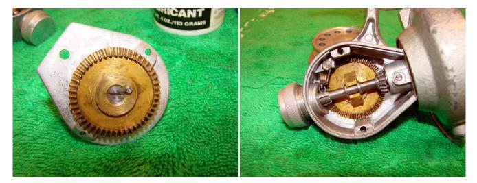
Lightly grease the main gear including where the slider contacts and then replace the side cover on the reel body.
