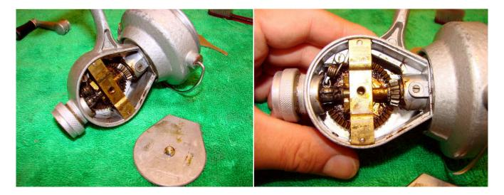
Unscrew the screw (#278) holding on the side cover and then remove the side cover. In order to remove #5057 you will need to loosen two screws on the left side reel cover.
