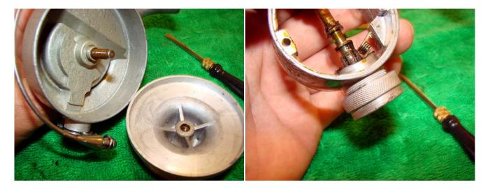
Unscrew the spool and remove the rear drag knob completely.
