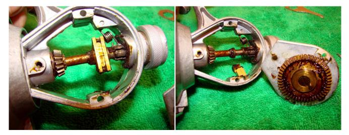
Remove the remaining screw on the left side cover and then lift off the left reel cover with the main gear. Remove the slider (#5020) from the main shaft. Looks like this reel has been lubed with Vegemite?!
