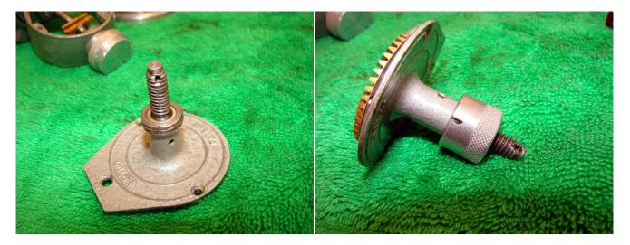
Lightly grease #5028 and then replace #5026 making sure that the #5028 is properly seated. Note the lubrication hole on the side cover for oiling the main gear shaft-a nice touch on such an old reel.
