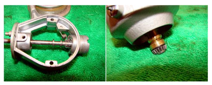
Add a light coating of oil to the main shaft and replace in the reel body. Add oil to the lubrication hole in the brass housing that the pinion gear sits in.
