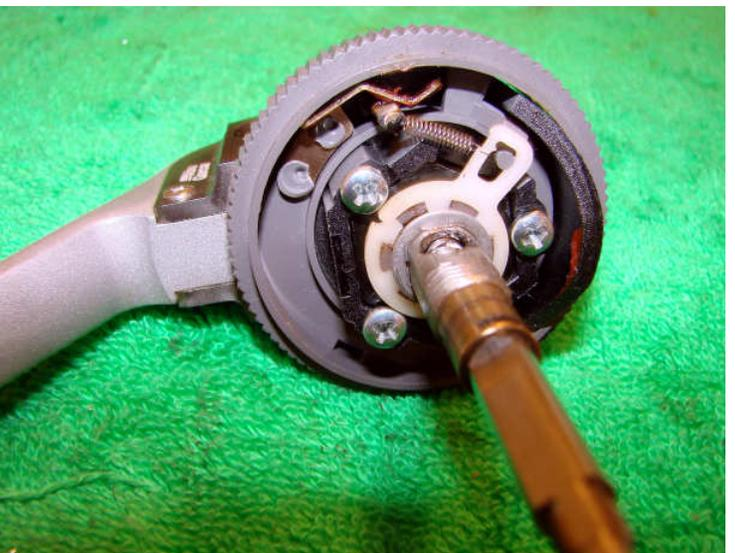
This seems to be the problem with the lack of line lay-the pawl is missing completely. Remove the pawl holder and then remove the three screws holding the anti reverse selector to the body.
