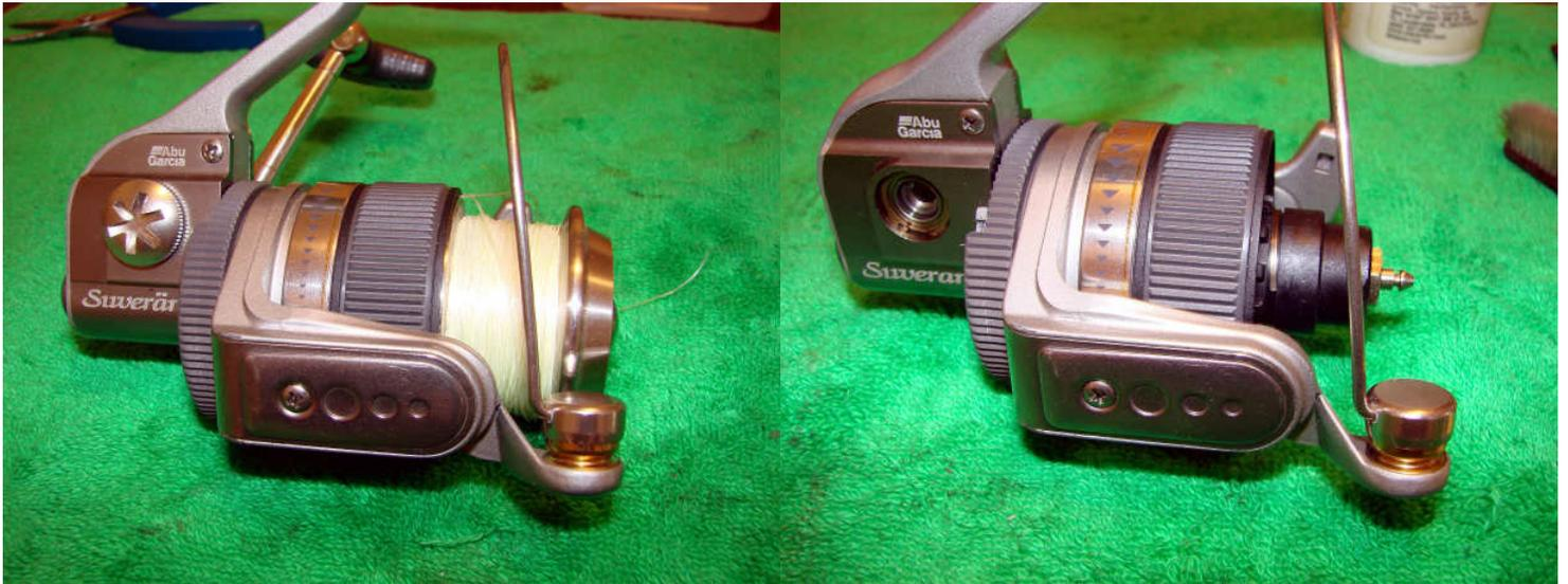
When this Suverän came to me it appeared to have a major problem-the spool did not move in and out when reeling the handle. As line lay is controlled by a worm gear and pawl I suspected that these were damaged. Overall the rest of the reel was in very nice working condition though.
