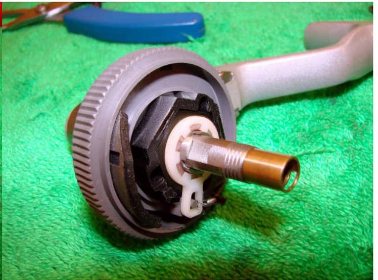
Grease the threads on the shaft nut and then replace. Replace the anti reverse assembly on the gearbox
