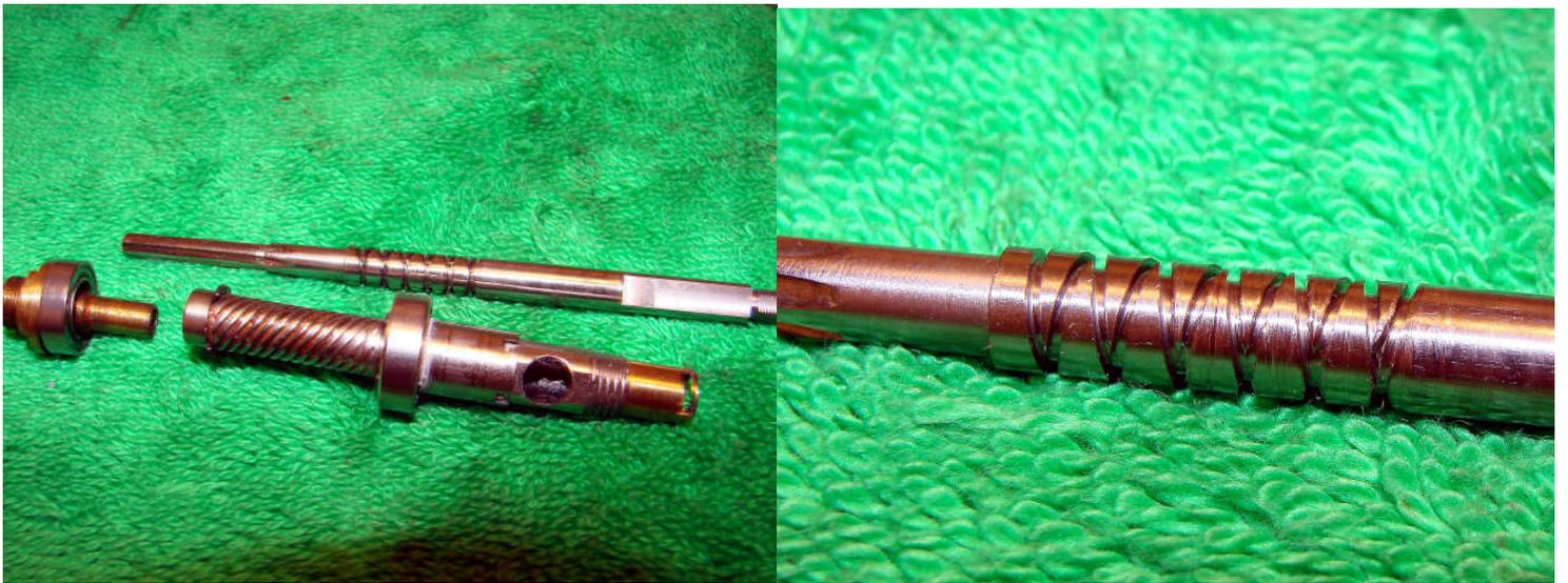
Remove the main shaft from the pinion gear-note the damage to the worm gear on the main shaft (teeth on far right). It looks as though the pawl and worm gear were jammed at some stage-the pawl is the only part holding the main shaft in the body and it is likely that a combination of a heavy drag and low stretch braid caused this problem.
