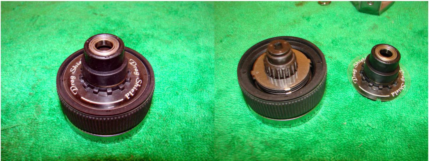
Remove the upper spool bushing (this contains the bearing and drag shield). Thoroughly clean the bearing and lubricate with light grease.
