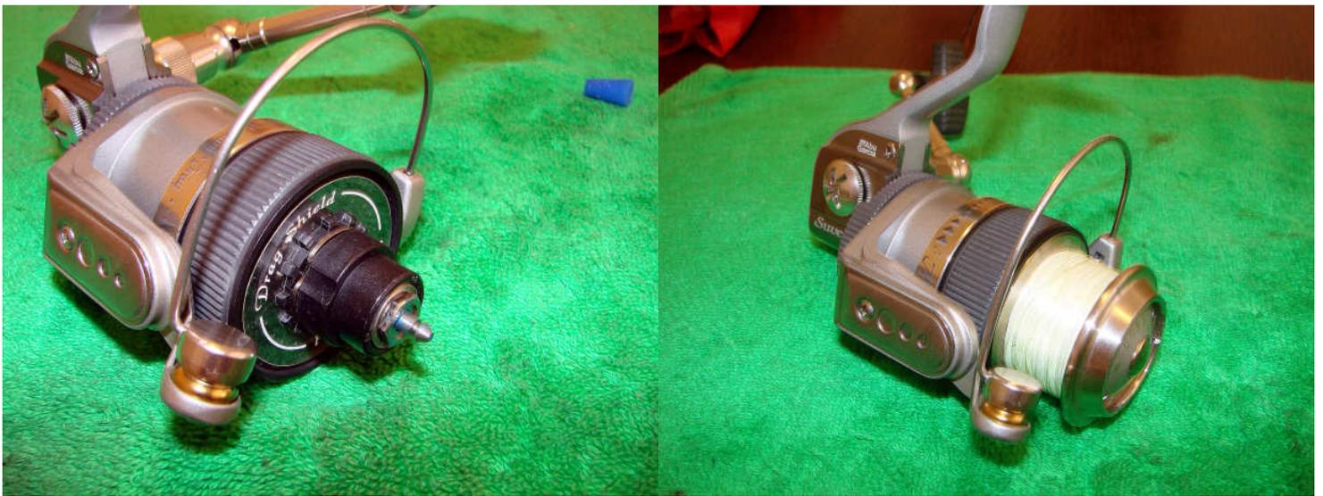
Replace the nut and finally replace the spool ensuring that it clicks into place properly.
