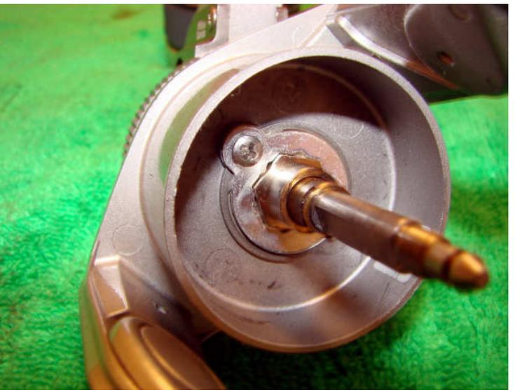
Note there is a rubber o-ring missing. Remove the rotor nut lock plate screw and the rotor nut lock plate.
