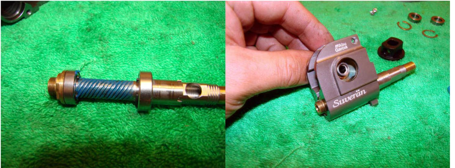
Clean and then lubricate all the bearings with a light grease (I use liquid grease). Grease the pinion gear and the main gear and then replace in the gearbox.
