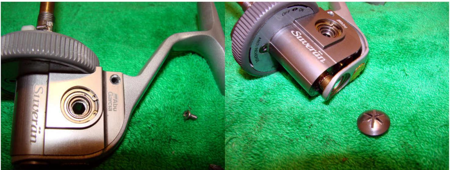
Undo the two screws holding the gearbox to the body (one either side) and then remove the screw securing the main shaft to the body.
