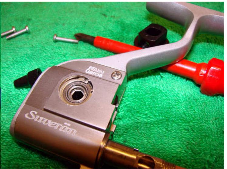
After cleaning and lubricating the bearings replace them in the gearbox and fix in place with the circlips. Replace the gearbox in the reel body and replace the two screws holding it in place.
