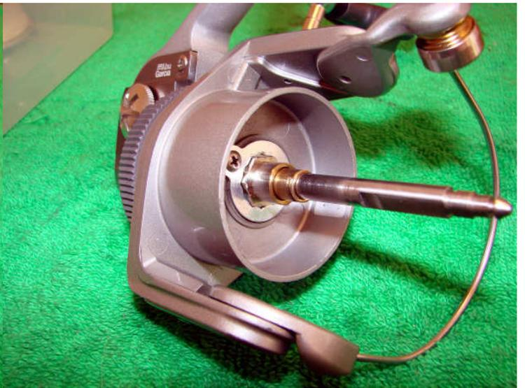
Replace the rotor (note that you have to line up the pawl assembly with a slot underneath the rotor). Replace the rotor nut, rotor nut lock plate, and rotor nut lock plate screw.
