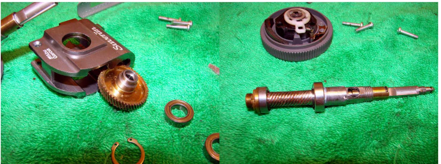
And then remove the bearings and main gear. The main shaft and pinion gear can then be removed.
