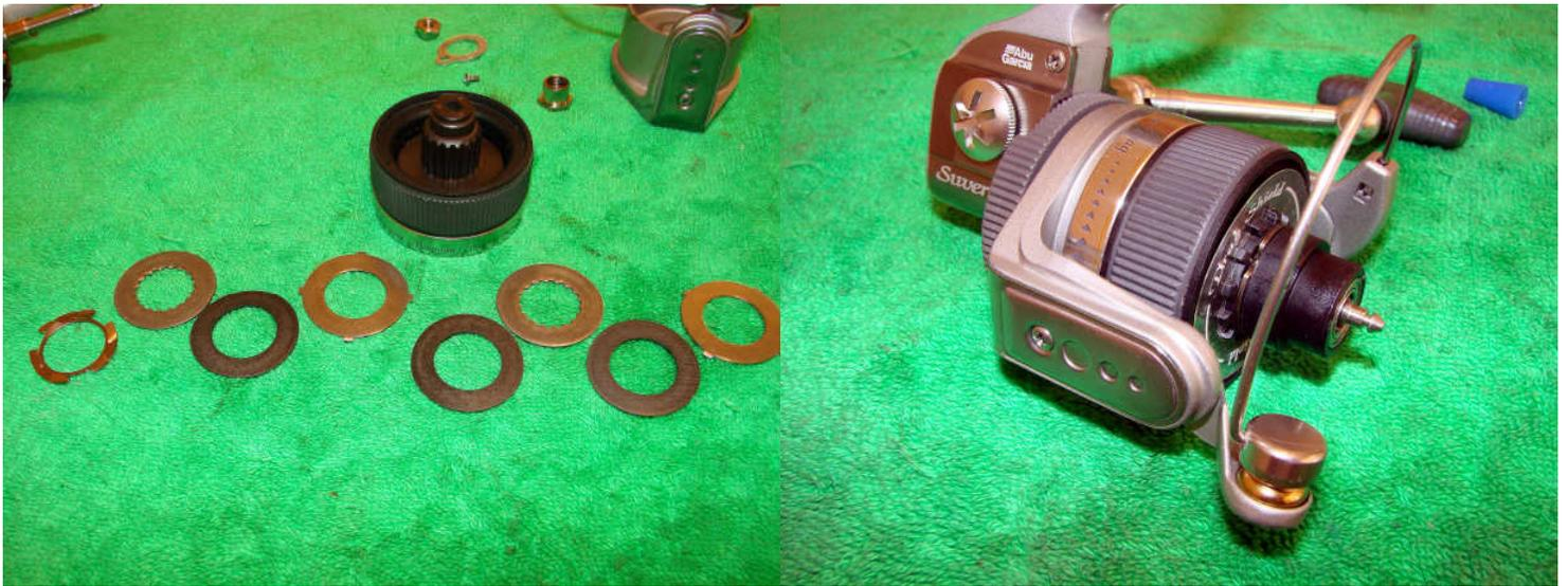
Separate out drag washers (left to right = bottom to top). Thoroughly clean the washers with a clean cloth soaked in lighter fluid. I don't have much faith in the drag shield and so I have greased the clean fiber washers with drag grease (Cal's drag grease). Replace the drag washers in the correct sequence and replace the upper spool bushing.
