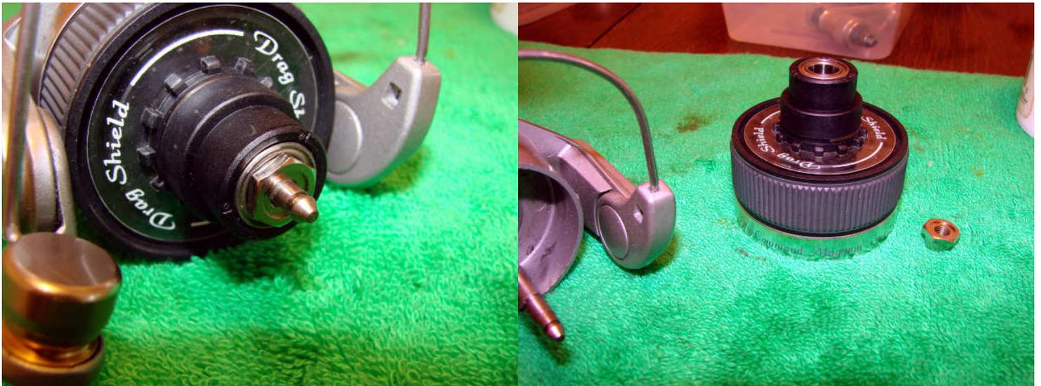
Remove the nut at the end of the main shaft and remove the entire drag system. Put this to one side to be worked on later.
