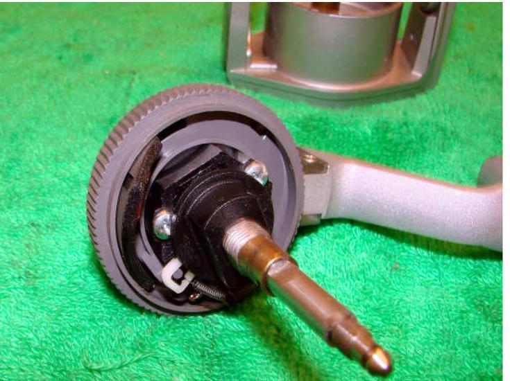
Undo the rotor nut and lift off the rotor.
