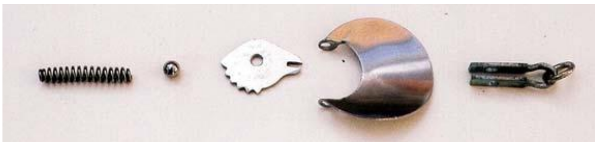
The clicker mechanism of an early Hi-Lo plug.
