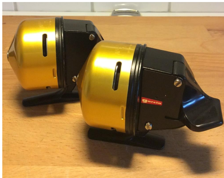
Two seemingly identical Abumatic 152 reels. But the one with the Garcia sticker is a regular 'on-top' reel, sold in the USA only, while the other is a prototype 'under-the-rod' reel that preceded it, but was never marketed. (Collection Leif Markström)
