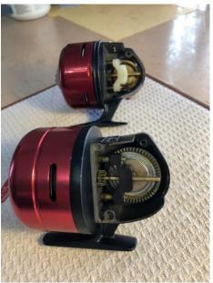
Next, we remove the side plates: Similar set up on both reels, but the oscillating block on the 170i is made of a black plastic while the original 170 is made of a white Teflon/Nomex compound that is more durable. Also, the side plates differ significantly from one another. On the original, the cover is made of aluminium and on the reproduced reel the side plate is made of graphite. Not a big issue for me on the latter material used.
