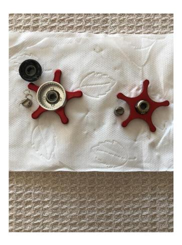
Both reels have aluminium handles, but the original have a smaller grip made from hard plastic while the remake have a larger more comfortable soft rubber paddle grip. The 170i's handle and star drag wheel are both painted red and is not properly anodised as the classic 170. Unfortunately, this painted finish is not durable and is easily chipped.
