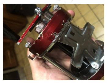
Back to the review, the original 170's body sleeve is made of solid brass which stand up way better to saltwater than aluminium.
