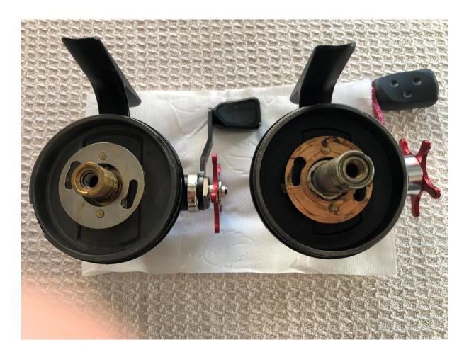
The body sleeve in which the pinion turns, is made of aluminium and is not the best choice for use in saltwater. Everybody knows aluminium does not rust, BUT pits and corrodes until the part breaks down. Just look what saltwater did to an Ambassadeur 7000's side plate if the anodizing got chipped and saltwater is not rinsed off properly!
