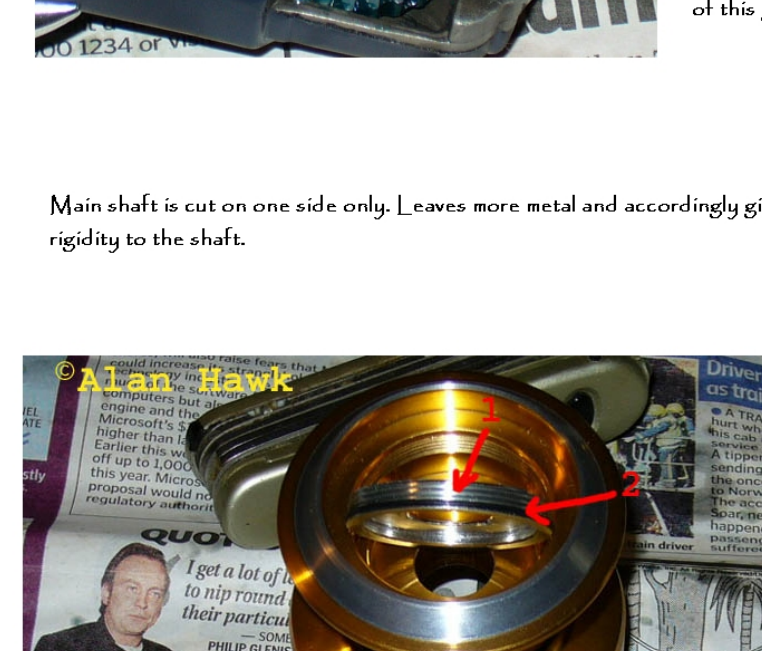
In most other reels, including some pricey ones, they simply keep the drag washers in place by a wire spring. But here they machined a metal disc with threads on its side (red arrow #1) that locks the drag washers securely in place, and it even has a rubber seal to keep water out (red arrow #2).
