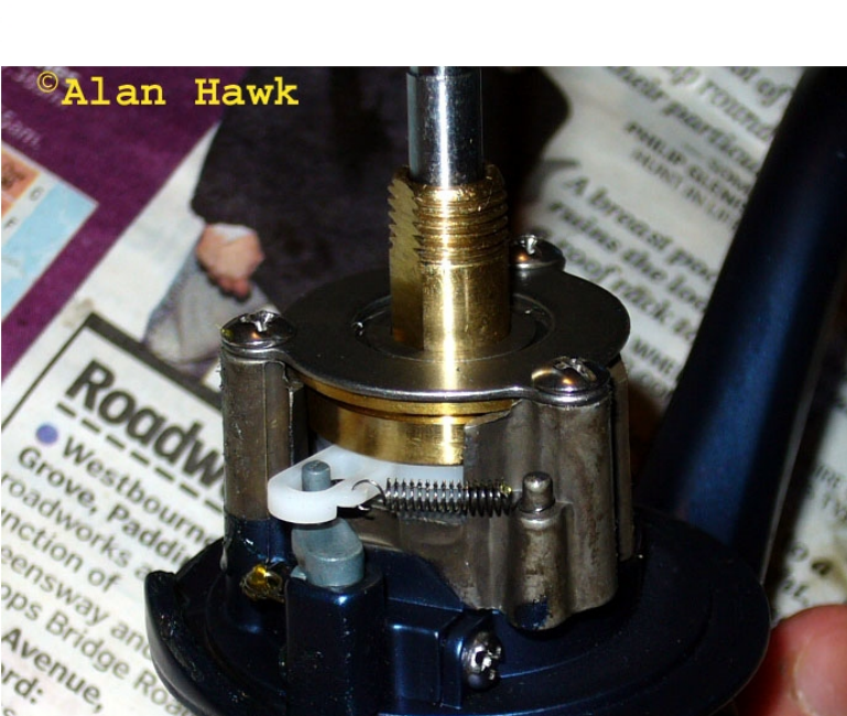
Looks like a regular one way clutch. But there is a twist...
