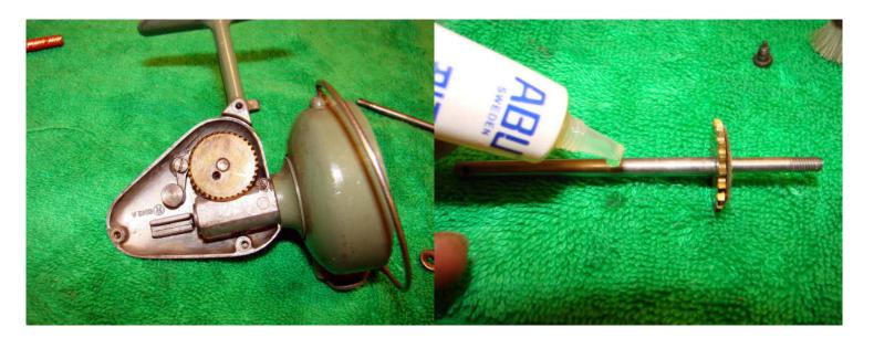
Clean the main gear and apply a light coat of grease to the gear teeth and the upper surface where the arm contacts. Apply a drop of oil to the clicker mechanism. Remove the screw on the pinion gear casing and apply a couple of drops of oil. Apply a light coat of oil to the main shaft.
