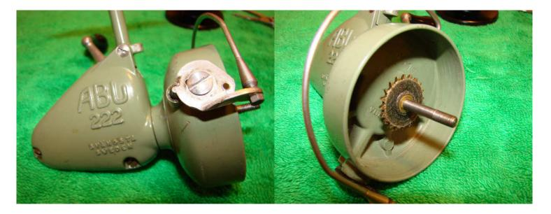
Apply a drop of oil to the side of the screw holding the bail arm on. Add a few drops of oil to the felt washer that sits under the spool and then replace the spool and drag knob.
