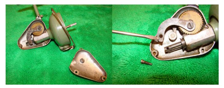
Remove the three screws holding on the side cover and remove the side cover. Remove the screw attaching the arm to the end of the main shaft.
