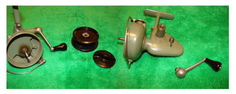
Remove the spool and unscrew the handle by turning backwards.
