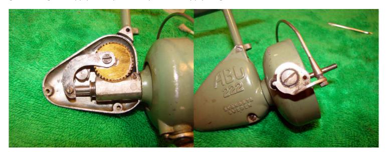
Replace the main shaft and arm. Note the screw in the housing for the pinion gear-remove this and add a couple of drops of oil. Replace the side cover and the three screws holding it in place. Remove the screw holding on the bail arm and apply a light coat of grease to the bail spring. Add a drop of oil to the bail trip mechanism (it sits below the bail spring).
