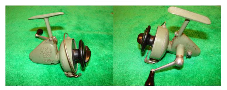
This reel seems to be working fine and just needs a quick service. The drag knob was broken but this can be easily repaired with some glue.
