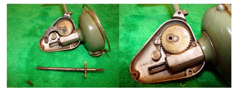
Remove the shaft and then remove the screw attaching the arm to the main gear. Remove the arm.
