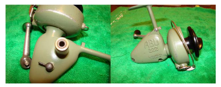
Add some oil to the shaft on the main gear ensuring that it penetrates fully and then replace the handle. Give the reel body a wipe down and you're done.
