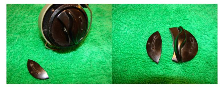
Unscrew the drag knob. Carefully clean both halves of the crack so that no oil/grease or other contaminants remain. Apply glue sparingly to the surfaces and join the two halves making sure they are lined up properly.
