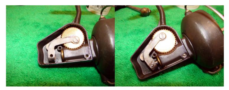
Add a light coating of oil to the main shaft and then replace it. Attach the arm to the end of the shaft.
