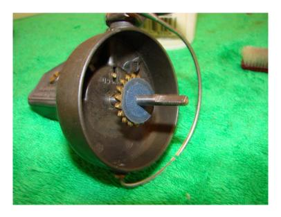
Add a few drops of oil to the felt washer sitting on top of the main shaft and then replace the spool and drag knob-this reel is ready to fish or to go in your display case!
