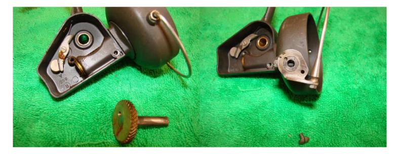
The main gear lifts out of the body. Remove the screw holding on the bail arm.
