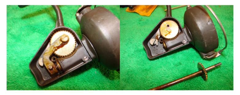
Remove the screws that connect the arm to the main gear and the end of the main shaft. Remove the main shaft and the arm.
