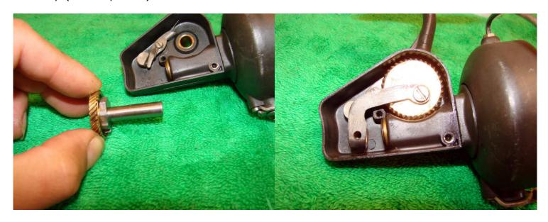
Clean the shaft of the main gear and give it a light coating of oil. Grease the teeth on the main gear with a coating of light grease and replace the gear in the reel body. Add a light coating of grease to the surface of the main hear and then replace the arm.
