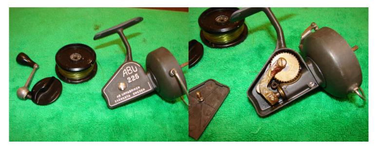
Remove the drag knob and spool, and then remove the handle by winding it backwards. The side cover is held in place by just one screw.
