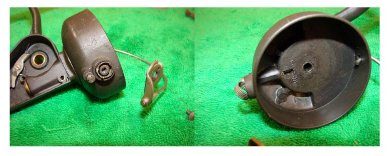
Fortunately the bail spring is not broken-it just needs a clean. Remove the bail spring and clean it and then give a light coat of grease. Lubricate the bail trip lever with a drop of oil where it
