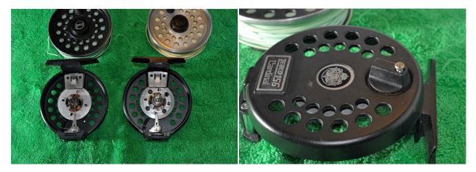
The spool is removed by simply pressing the push button in the middle and lifting it off. Internally there are no differences apart from the fact that the Zebco does not have the holes in the drag plate. In addition in the Zebco you can see the studs used to fix on the name plate. Servicing is the same for both reels. Undo the screw for the drag knob and remove it.
