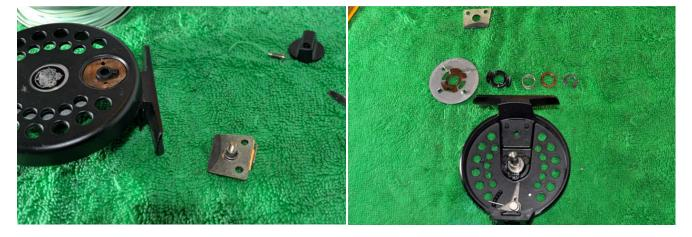
Note the copper washer under the drag knob. The outer cork drag plate will fall out from the other side-note the spring. Remove the c-clip on the spool shaft and remove the components. They are laid out left to right=top to bottom; drag disc, plastic cam, spring, copper washer and c-clip. The other cork drag plate at the top of the photo sits under the metal drag disc-it is the last part to be removed from the reel body.
