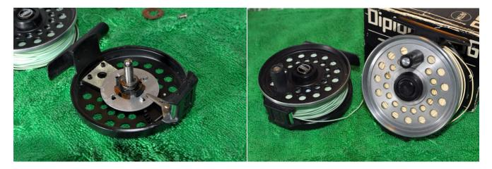
Give everything a thorough clean before reassembly. The cork drag plates can be lightly greased with drag grease. Use light oil on the other friction surfaces including the spool clicker. The spool clicker will need to be pushed out of the way before the metal drag disc can be replaced.
