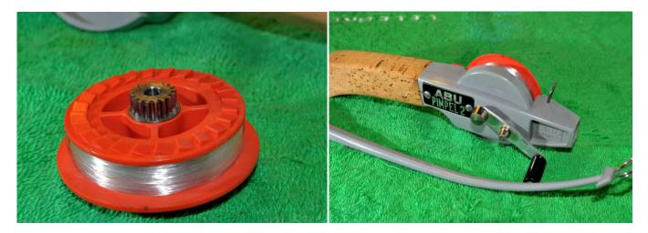
Add some grease to the teeth on the main gear and some oil to the spool shaft. Replace the spool on the body and you're finished-very quick and simple!
