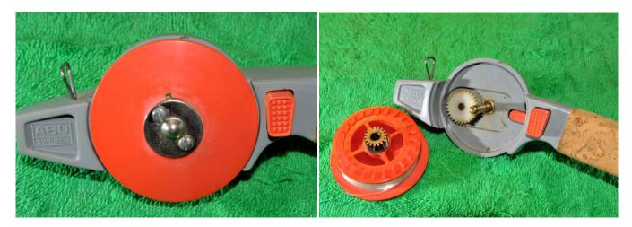
A lever on the spool allows it to be removed-simply push the lever to one side and the spool lifts off. The pinion gear is fixed to the bottom of the spool and is brass, note that the main gear is plastic.
