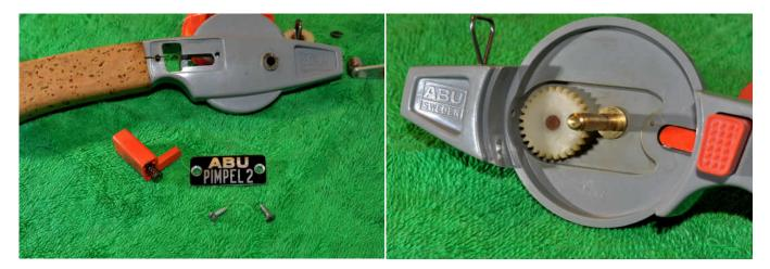
The anti reverse mechanism simply lifts out. Check that the spring is in good order-give a light coating of grease and then replace. Give everything a thorough clean and then reassemble. Add some oil to the shaft of the main gear and then replace in the body. Fix in place with the c-clip and then replace the handle and handle nut.
