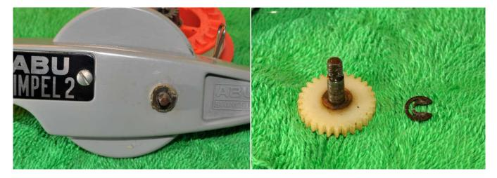
Remove the handle nut and handle. There is a c-clip on the shaft for the main gear holding it in the body. Remove this and the main gear can be removed from the other side. Note the copper washer on top of the main gear.
