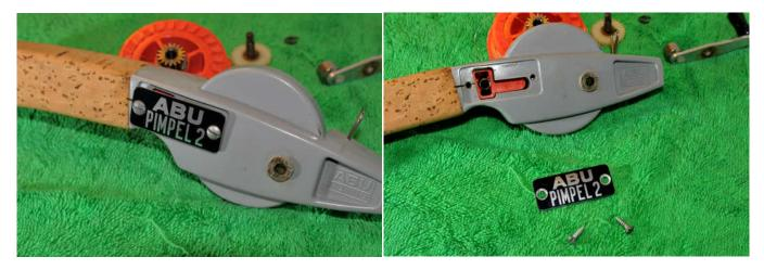
To access the anti reverse mechanism remove the two screws on the metal plate and then remove the plate.
