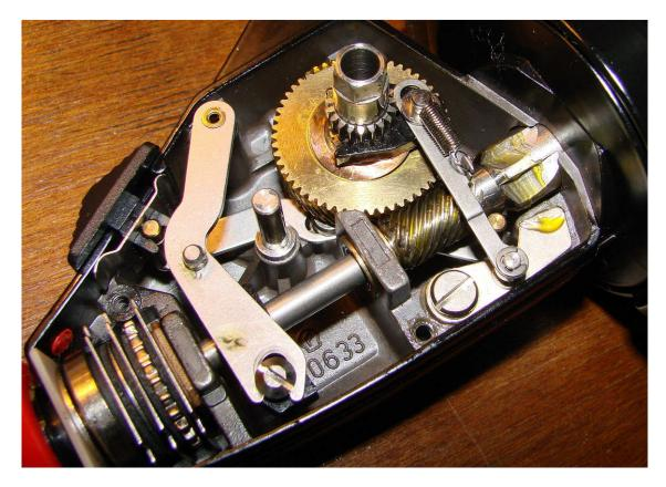
If you turn the rotor backwards you can see if the anti reverse dog engages-in this photo it is not engaged.
