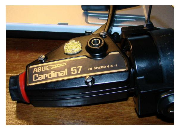
Remove the three side plate screws and remove side plate (after removing handle)
