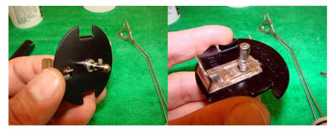
Insert the spindle and add the spring on the other side.
