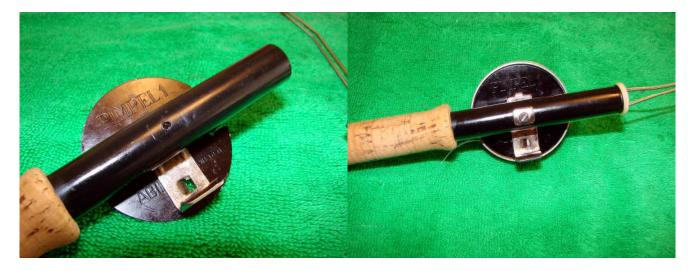
Place the whole assembly back on the rod handle and fix in place with the washer and screw (lightly greased).
