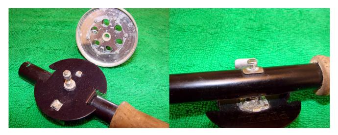
There is some corrosion here. Turn the reel over and unscrew the screw on the other side. Remove the screw and washer.
