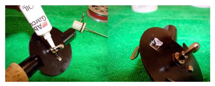
Add a drop of oil to the spindle and a dab of grease where the click plate contacts the studs on the spool. Reattach the spool.
