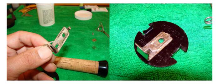
Smear some grease on the free spool button/clicker plate and place back on the reel plate.
