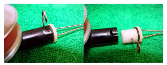
The rod part is bayonet fit and you simply twist and pull to remove.
