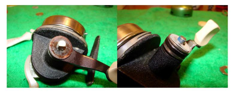
Then add a fibre washer/handle/fibre washer, flat metal washer, curved metal washer.
