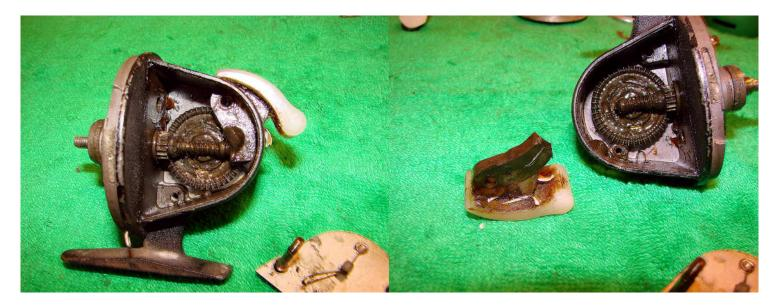
Oh dear-looks like the reel is filled with tar. No wonder it felt sluggish. The thumb button simply pulls out; it pivots on one of the side plate screws. Give everything a thorough clean. I prefer not to use solvents on plastic but this means *a lot* of scrubbing with washing up liquid and warm water.
