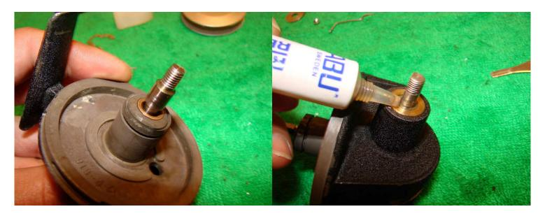
Push in the throw out spring with your finger and then turn the reel over. Apply oil to the gap between the winding cup shaft and the reel body. Wipe off any excess. Apply oil to the drive shaft/drive shaft bushing and let it penetrate. Wipe of excess.
