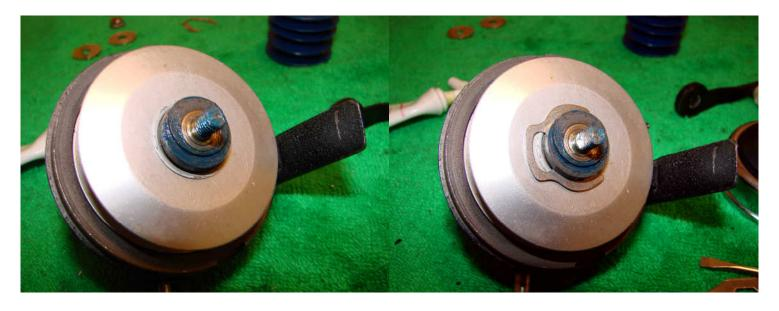
Reattach the spool and add a light coating of grease where the line pick up ejector contacts the body (don't forget to add a light coating of oil/grease to the friction surfaces on the ejector on the underside of the winding cup). Replace the circlip.
