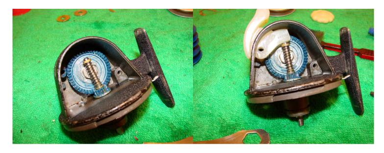
When everything is spotless apply grease to the gears. A toothbrush is good for ensuring coverage to the base of the teeth. Apply some light grease to the friction surfaces on the thumb button. Add a light coating of oil on the throw out pin and spring.
