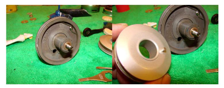
Note the stud on the spool and the corresponding hole on the reel body. These need to be lined up so that the spool is fixed.
