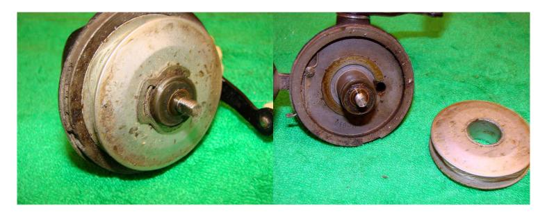
Remove the circlip that holds on the spool and then remove the spool. Note the hole in the reel body where the spool sits. The spool has a corresponding stud-this reel is a *true* fixed spool reel; the spool never moves, only the winding cup.
