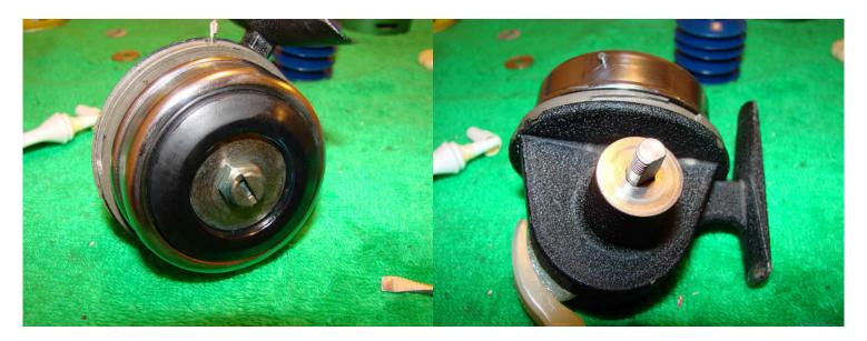
Reattach the winding cup and nut. Attach the flat metal washer to the drive/handle shaft.
