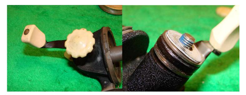
Unscrew the drag knob and remove the handle. Note the orientation of the washers. From the top, drag knob, curved metal washer, flat metal washer, fiber washer, handle, fiber washer, flat metal washer.
