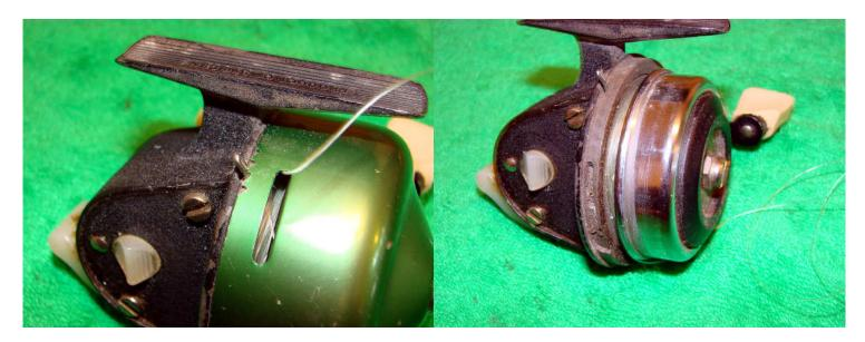
First thing to do is remove the bell cover. To do this depress the wire lock towards the reel body and then twist the cover-it is bayonet mount.
