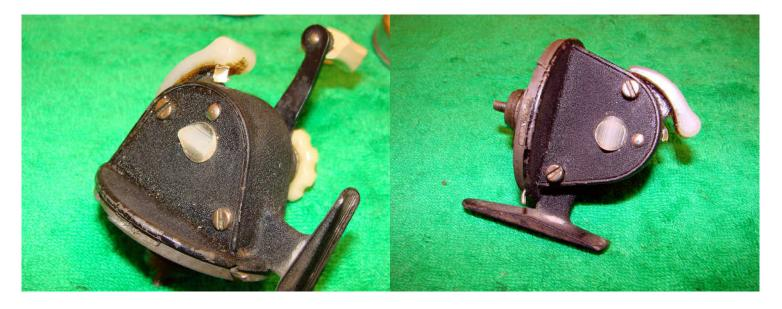
Remove the two screws holding on the side plate.
