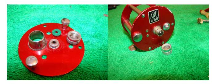
Remove the right spool cap and pry out the felt washer with a toothpick. This can be cleaned by soaking in lighter fluid. Remove the left spool cap.
