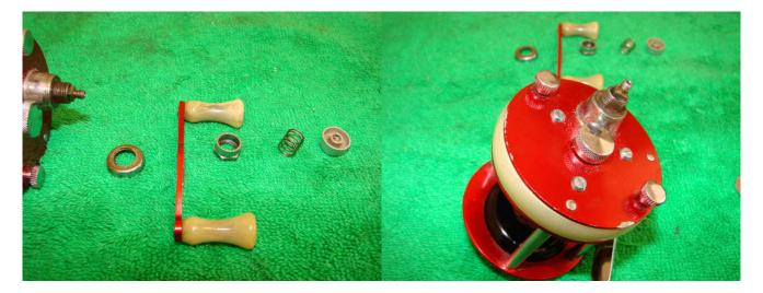
Remove the dust shield. Everything is laid out in sequence. Unscrew the two thumbnuts on the right plate.
