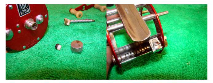
And remove the spool bearing. Remove the level wind assembly from the frame by undoing the line carriage screw and removing the pawl. The worm gear can then be removed from the line carriage.
