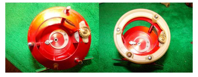
Add a drop of liquid grease to the clicker assembly. Move the clicker side to side to make sure it is worked in properly. Replace the head ring (plate spacer).
