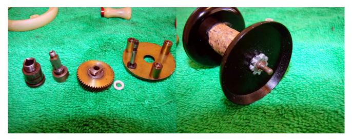
Followed by the drive gear and gear shaft bearing (white plastic washer). The spool shaft on the clicker side shows corrosion and will need to be cleaned up.
