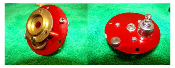
Replace the bridge gear unit on the side plate and fix in place with the three bridge screws. Replace the dust shield.
