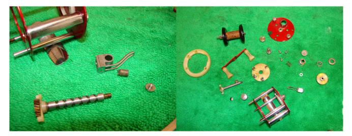
Worm gear (foreground), line carriage next to pawl and line carriage screw to the right of the photo. Everything is now ready for a thorough clean before reassembly. I prefer not to use harsh cleaners on older reels. A clean using warm water and washing up liquid followed by a thorough rinse should be sufficient.
