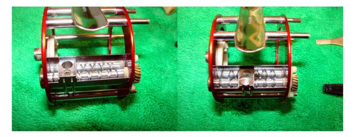
Add a drop of oil to either side of the worm gear. Make sure that it soaks in past the plastic bushing. Replace the worm gear and the line carriage in the frame. Replace the pawl and the line carriage screw. The line carriage sits on the worm gear so smear oil/liquid grease on the entire worm gear and not just in the grooves.
