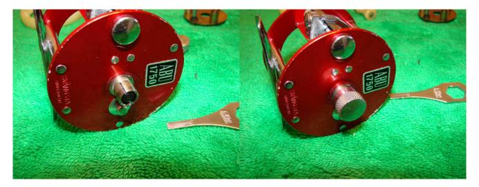
Add a drop of oil to the spool bearing and replace in the left side plate. Replace the left spool cap.
