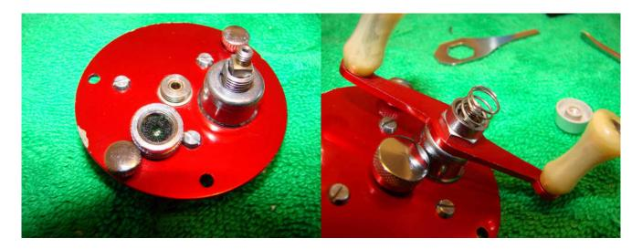
Replace the felt washer in the right spool cap and add a few drops of oil to it. Add a drop of oil to the bushing in the side plate before replacing the spool cap. Replace the dust shield followed by the handle. Replace the free spool spring and the free spool button.
