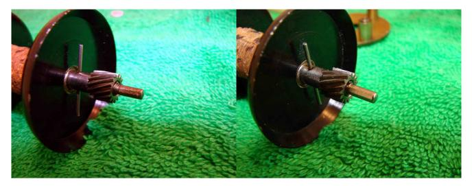
As will the drive gear side. Second photo shows corrosion removed. If you use a metal polish make sure to wash the part thoroughly to remove any trace of the polish. Note that there are no brake blocks present.
