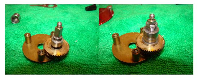
Replace the main gear on the drive shaft followed by the lock pin retainer and the handle bearing. Lubricate the handle bearing with liquid grease or heavy oil.
