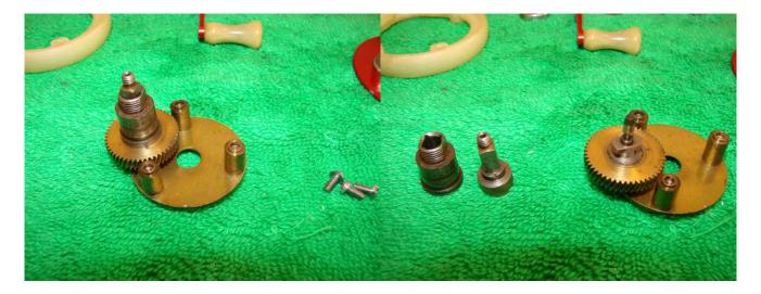
Remove the entire gear bridge unit from the other side of the side plate. The handle bearing and lock pin retainer can then be removed.
