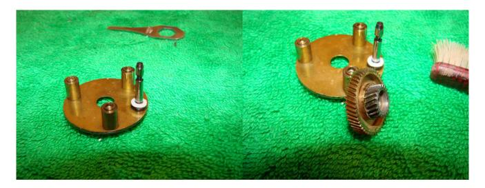
Add a drop of oil to the drive shaft and replace the drive shaft bearing (plastic washer). At this stage it is easier to add grease to the teeth on the main gear. I have used a light liquid grease.
