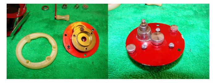
Remove the whole side plate and head ring (plate spacer). Remove the three bridge screws.
