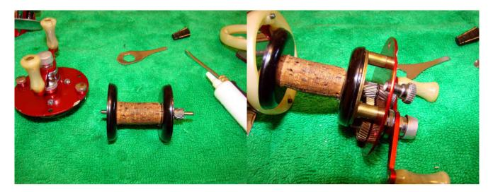
Add a drop of oil to both ends of the spool shaft and then replace the spool in the right side plate. The spool and side plate can then be replaced in the frame. Tighten the two thumb nuts.
