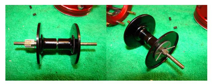
It must have been a huge amount of force to cause the spool to separate and bend the brake pins (judging by the force required to get them back together). I have no idea what could have caused it.
