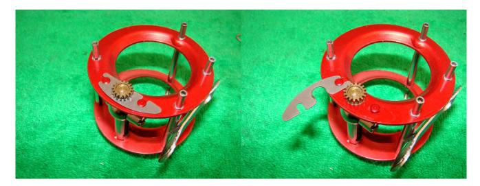
The carriage screw lock is on upside down here! Remove by sliding off.
