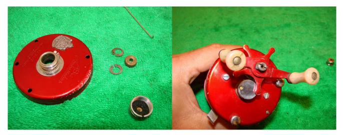
Remove the circlips and the bushing. The felt can be pried out of the spool cap with a tooth pick and the copper shims can be removed. Clean the felt washer by soaking in lighter fuel. Undo the handle nut and remove the screw.
