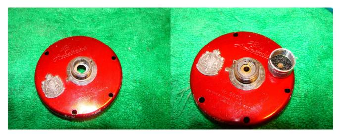
Replace the bottom circlip. Soak the bushing in oil and wipe of any excess and then replace it followed by the top circlip. Replace the shims in the spool cap (with a drop of oil), and then replace the felt washer. Apply oil to the felt washer and then replace the spool cap ensuring that the indicator wire fits properly into the slot.
