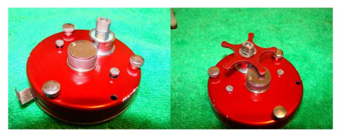
Replace the side plate on the brake plate. Grease the threads on the bridge screws and snug them down. Replace the star drag.
