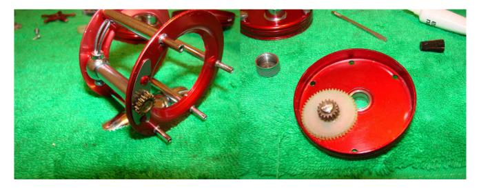
Replace the carriage screw lock, the pawl and the line carriage nut. Add a drop of oil either side of the carriage screw (in the threads). Add a drop of oil to the idler gear post and then replace the idler gear and the retaining screw. Spread liquid grease on the teeth of the idler gear.
