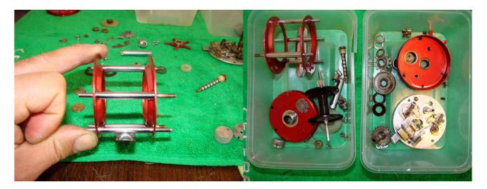
Without the side plates maintaining rigidity this frame shows a bit of flex! Everything needs to be cleaned before reassembly. Washing up liquid, warm water and a toothbrush should get things clean (use lighter fluid for the bushings, centrifugal brakes and the drag washers). If there are stubborn grease and oil deposits you can use lighter fluid/shellite, though I wouldn't recommend using it on plastic parts. Make sure that you rinse and dry all parts thoroughly.
