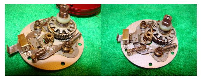
No sign of lubrication though there is no corrosion to speak of. Remove the main gear assembly and the pinion gear for cleaning. You may find it easier to remove the pinion gear if you place the reel in free spool by pressing in the thumb button.
