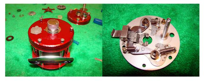
Replace the side plate on the frame. Grease the threads on the four pillar screws and snug them down firmly (not too tight). Time to move on to the brake plate.
