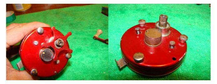
Remove the handle and star drag and then undo the three thumb nuts and remove the side plate from the frame. Undo the two bridge screws and remove the side plate from the brake plate.
