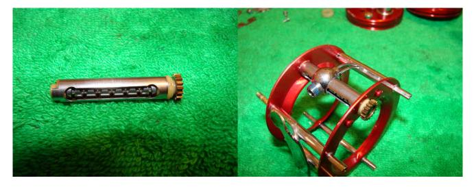
Add a drop of oil either side of the bushing on the carriage screw (near the gear) and one where it contacts with the plastic bushing in the cover. Place the assembly back in the frame. Grease the threads on the level wind.
