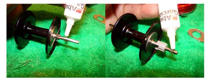
Add oil to the spool shaft on both the left and right hand side of the spool.
