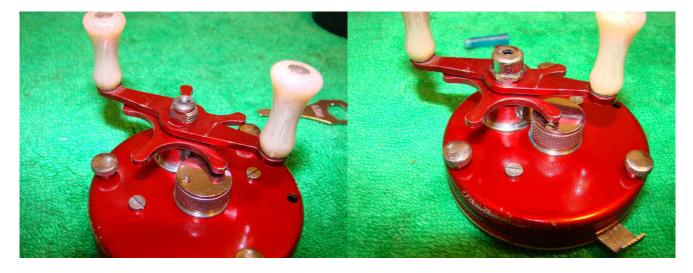
Replace the handle and drive shaft screw followed by the handle nut. Make sure it is snug as there is no handle nut lock on these older Ambassadeurs.
