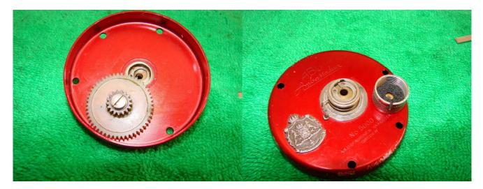
Remove the four pillar screws holding on the left side plate. Remove the idler gear screw and remove the idler gear. Turn the plate over and remove the spool cap.
