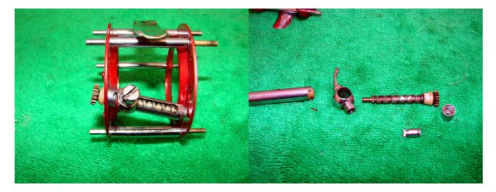
Remove the line carriage nut and pawl and then the carriage screw and cover can be removed from the side of the frame.
