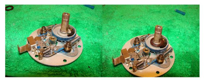
Replace the main gear and the pinion gear. Apply grease to the gears ensuring that it reaches the base of the gear teeth. A small paint brush is useful for ensuring even coverage. Replace the top drag washer-I found that if this is greased it can make the drag jerky-as such leave it dry.
