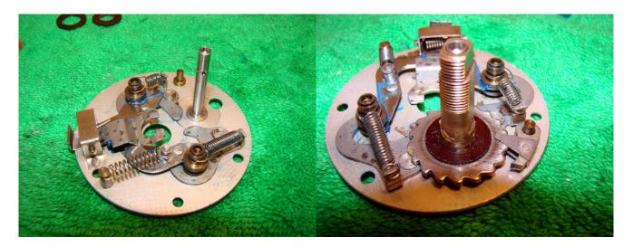
Apply a thin smear of grease to all of the friction surfaces (you can add a drop of oil to each stud that attaches the press arms to the brake plate). Smear liquid grease on the drive shaft post and then attach the drive shaft and anti reverse dog. Apply a thin smear of drag grease where the ears of the anti reverse dog grip. Apply a very light smear of drag grease to the base drag washer and the drive shaft where it contacts with the main gear.
