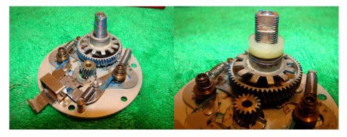
Replace the click wheel and then the curved washer followed by the flat washer and the drive shaft bearing. Smear liquid grease to the outside of the drive shaft bearing.
