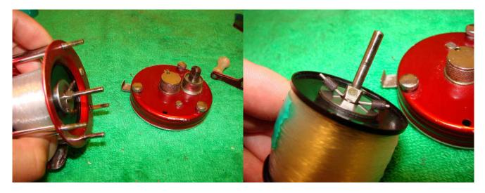
When I removed the right side plate the centrifugal brake pins looked bizarre-like they had been forced upwards.
