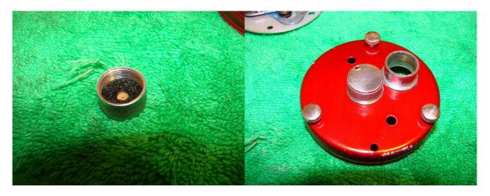
Replace the circlip in the right side plate followed by the bushing (soak in oil first and remove any excess). Replace the copper shims in the spool cap with a drop of oil. Replace the felt washer and saturate it with oil. Grease the threads for the spool cap and replace the spool cap ensuring that it is screwed in fully.
