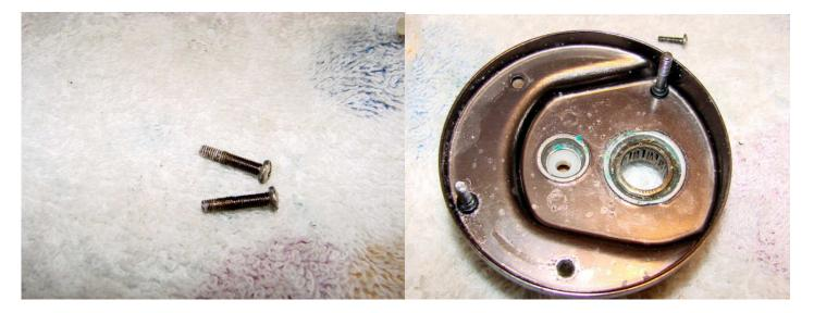
These screws need to be replaced. Fortunately the inside of the side plate is not as bad as it looks. The IAR bearing works fine and the corrosion on the plate can be cleaned off. To prevent future corrosion you can put a little bit of grease on your finger and smear it on the inside of the side plate.
