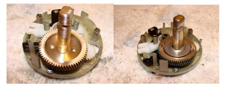
Apply some light grease to the teeth on the plastic level wind drive gear and ensure it is sitting correctly underneath the main gear before replacing this on the drive shaft.
