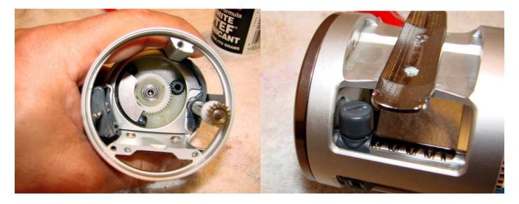
Make sure that the line guide is sitting correctly in the frame and then replace the pawl and washer and the line guide nut. Add a few drops of oil to the grooves in the worm gear.
