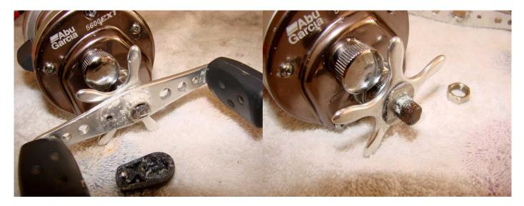
Remove the handle nut cover and the handle nut. Lift off the handle. Salt deposits are very evident.
