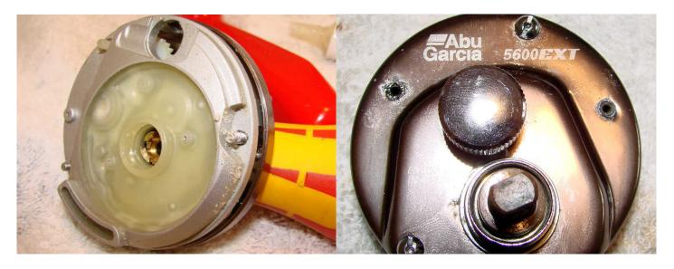
The clutch plate shows some salt deposits-interestingly it is made of plastic; no corrosion worries at least! Remove the two remaining side plate screws and lift the side plate from the clutch plate. Unfortunately the right side plate is showing a little bit of corrosion around the screw holes.
