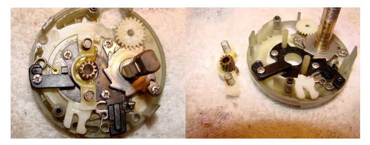
The left photo shows the clutch plate before disassembly. Firstly remove the pinion yoke (with two springs) and the pinion gear.
