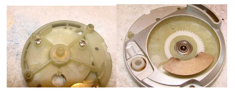
Remove the magnet carrier by removing the two screws on the other side of the inner side plate. The mag carrier simply lifts off. Remove the mag adjustment plate. Note that there are cut outs on the white plastic part-line these up with the notches on the inner brake plate and then you can lift it off.
