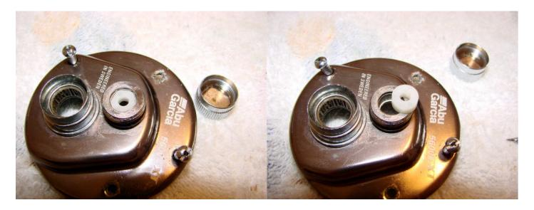
Remove the right spool cap. Remove the clip and take out the plastic bushing. Give the bushing a thorough clean before replacing and fixing it back in place with the clip. Remove the copper shims from the spool cap and give the cap and shims a thorough clean. Add a drop of oil in the spool cap before replacing the shims. Add a drop of oil on top of the shims (the spool shaft contacts here).
