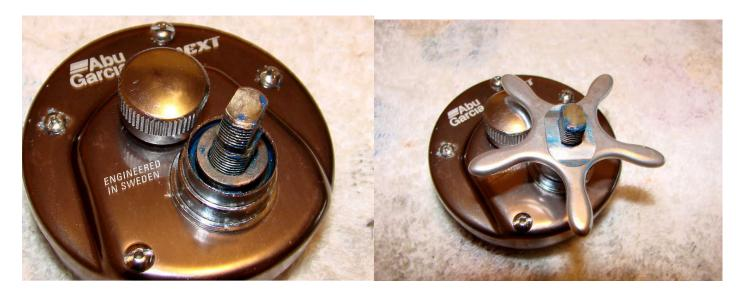
Grease the o-ring and the threads for the spool cap and then replace it on the side plate. Make sure that the threads on the main shaft are greased and then replace the star drag and the friction washer.
