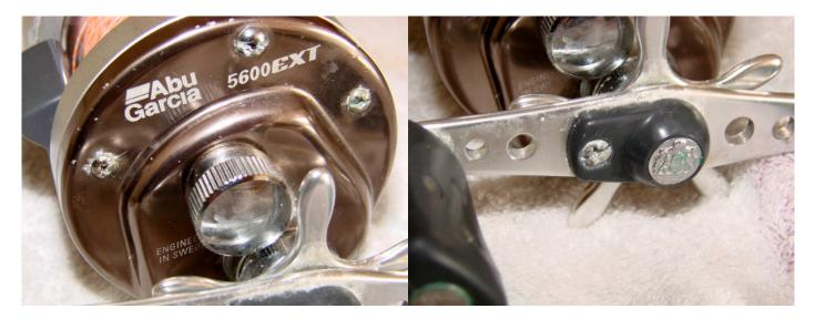
The screws and part of the side plate have suffered from saltwater corrosion. The screws were actually seized tight and wouldn't move. Don't try to force stuck screws-this may cause them to snap off, especially if they have been badly corroded by salt. In this case the screws were liberally coated with penetrating fluid and left overnight. Fortunately this did the trick.
