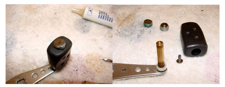
Before replacing the handle you can grease/oil the spindles for the handle knobs.
