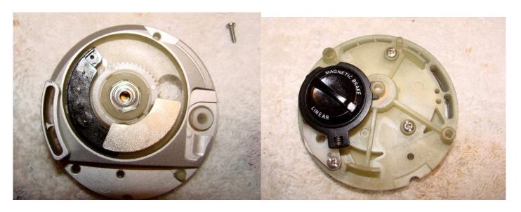
Replace the mag carrier in the inner side plate and fix in place with the two screws. The mag adjuster can then be replaced on the side plate.
