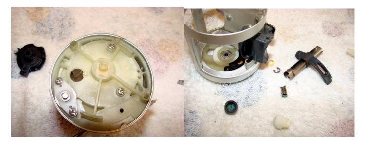
The black mag control simply lifts off. To the left of the plate is a circlip holding on the level wind assembly. Remove this to free up the level wind and then remove the level wind. Disassemble the level wind for cleaning. Note that there is a small washer that sits underneath the level wind pawl.
