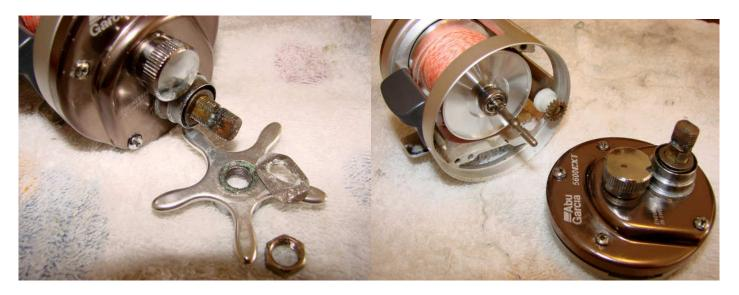
Remove the friction washer and undo the star drag. Undo the two side plate screws (the ones at the top and the bottom of the side plate) and remove the side plate. If the side plate seems hard to remove try pushing on the clutch plate from the inner side of the frame.
