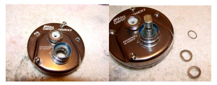
Replace the side plate on the clutch plate and fix in place with the side plate screws-of course the threads are greased now! Three washers need to be replaced on top of the bearing sleeve-the small washer is first followed by the two curved washers. Note that the correct orientation is ( ).
