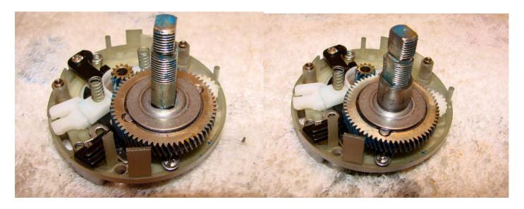
I have put a light coating of grease on the main shaft to minimize any effects of water intrusion. Replace the IAR bearing sleeve-note it can only fit on in one way.
