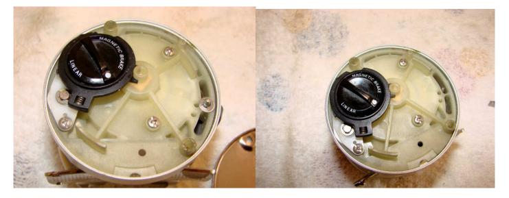
Interestingly the inner side plate is also plastic-note the drain holes at the bottom of the inner side plate. To the right of the inner side plate is a circlip holding the thumb bar in place. Remove this to free the thumb bar from the inner plate.
