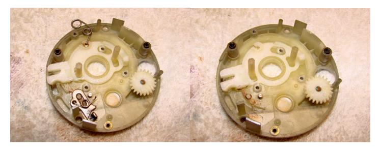
With the position holder removed the springs can be removed. Note the top spring has a brass insert. Remove the kick lever (metal part), and then finally remove the lift curve (white plastic part).
