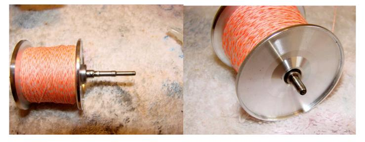
Add a drop of oil to the bearing on the right side of the spool. Clean the spool shaft thoroughly and smear some oil on the right hand shaft where it contacts the pinion gear. Clean both spool tips and add a drop of oil to each end.
