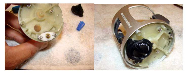
Reassemble the whole level wind assembly and replace it in the side plate. You may find it easier to do this if you replace the side plate in the frame first and without the mag adjuster in place.
