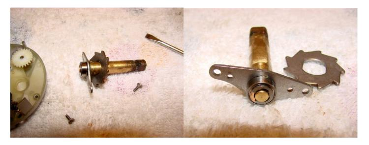
Remove the two screws holding the main shaft assembly and remove from the brake plate. The ratchet slides off the main shaft. Note the circlip at the base of the main shaft. Remove this and separate out the parts.
