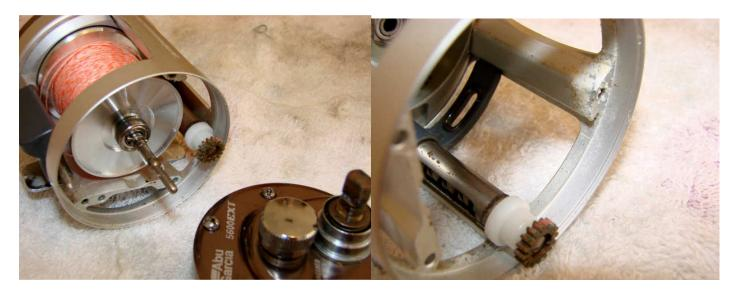
Remove the spool from the right side of the frame. The frame and level wind look as if they have been affected by salt water.
