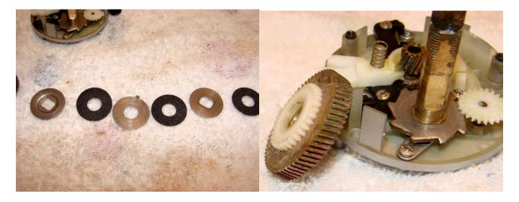
Drag washers separated out. Left to right = top to bottom. The drag looks to be unaffected by saltwater intrusion though the same cannot be said of the main gear and pinion gear teeth. It's nice to see that the drag washers are the new carbon style.
