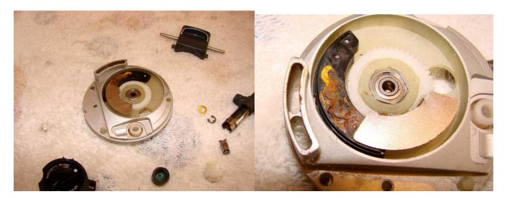
Push the inner side plate out from the frame-there are no screws holding it in place. The corrosion on the magnet carrier doesn't look good.
