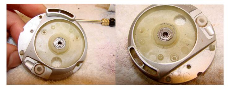
Remove the bearing from the left inner side plate-it is held in place with a clip. Give the bearing a thorough clean and when it is dry add a drop of oil of your choice. There will be a copper shim underneath the bearing-clean this off and then replace in the side plate.
