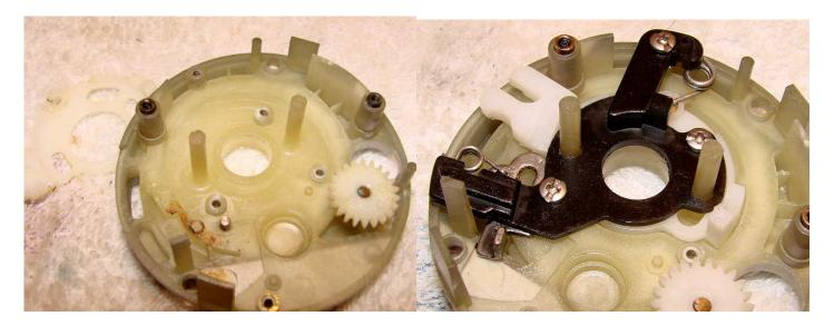
It is not really necessary to remove the worm drive gear. Give the clutch plate a thorough clean before reassembly.
