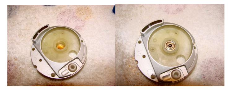
Add a drop of oil to the copper shim and then replace the bearing and clip.
