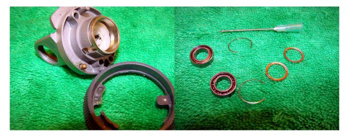
Make sure that you don't lose the stopper and spring-it sits in the gear box. Clean everything before reassembly. Shields can be removed from the bearings to clean out old grease.
