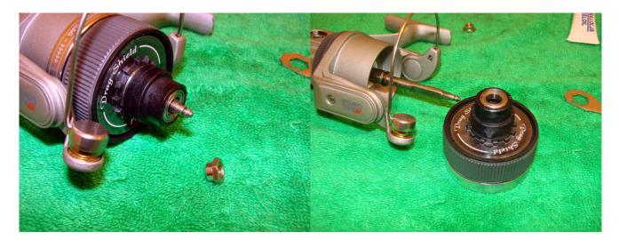
Remove the spool and undo the nut holding on the centre drag assembly. Put the drag assembly to one side as we do the rest of the reel.
