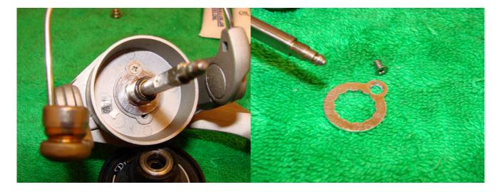
Remove the rotor nut lock plate screw and the rotor nut lock plate.
