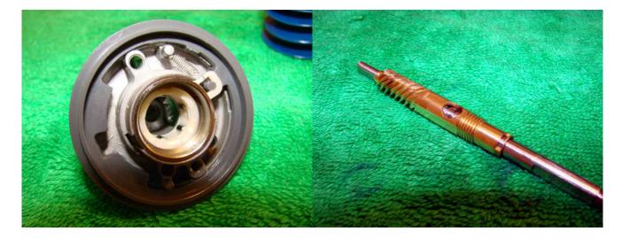
Replace the stopper lever ensuring that the pin stays in place. Snug down the sleeve and replace the spring. Smear liquid grease on the main shaft and grooves for the pawl and then replace in the pinion.
