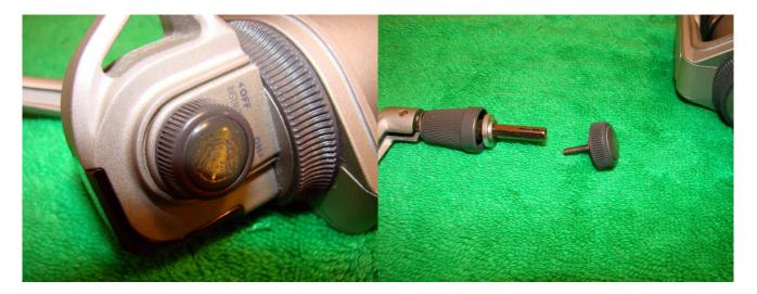
Remove the handle by unscrewing the handle knob.
