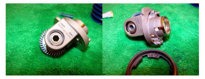
Replace the bearings and retaining clips. Pull the sleeve up slightly so that the stopper lever can be replaced. Smear some grease where the pin contacts.
