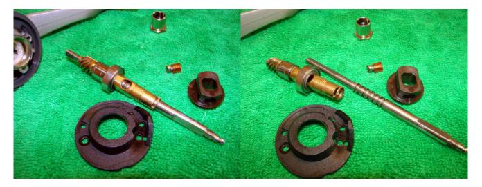
Remove the pawl, pawl holder and the flange cover. The main shaft can be removed from the pinion gear.
