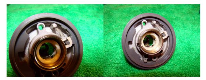
Remove the spring and slide out the sleeve just enough so that the clutch lever can be raised to allow the stopper lever to be removed. Clean the rollers on the one way bearing with a cotton bud soaked in lighter fuel. When completely dry run a bud with a drop of oil on it around the rollers. Do NOT over lubricate the one way bearing.
