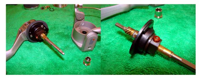
The rotor will lift off. Remove the four screws holding on the flange cover and remove the whole assembly.
