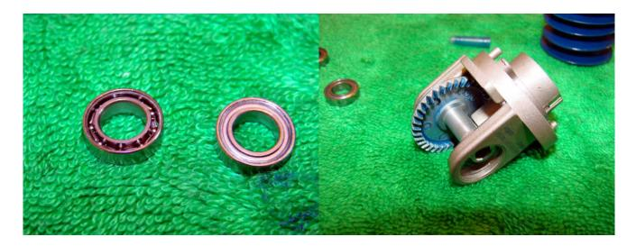
Pack the bearings with your lubricant of choice. I found grease alone to be a bit too thick so I used a mixture of oil and grease. Replace the shields and retaining clips. Put grease on the main gear and place back in the gear box. Don't forget the washer on the other side of the main gear.
