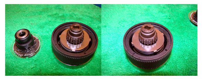
Remove the upper spool bushing (contains the bearing and drag shield). Close inspection of the drag assembly shows that the washers are not in the correct sequence.
