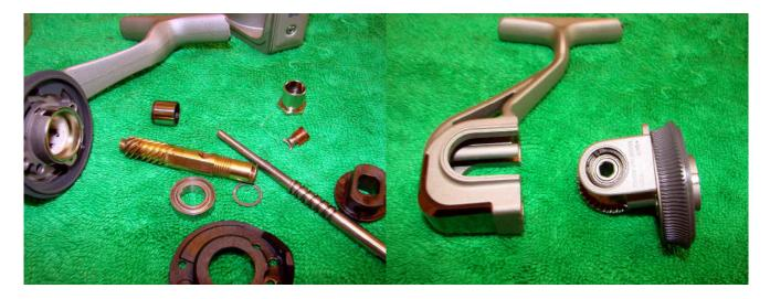
You can then remove the bearing, sleeve and washer. The gear box slides out of the body.
