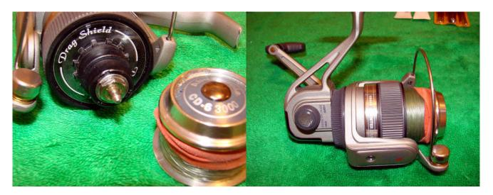
Replace the whole drag assembly back on the main shaft ensuring that it is seated properly. Replace the nut and spool.
