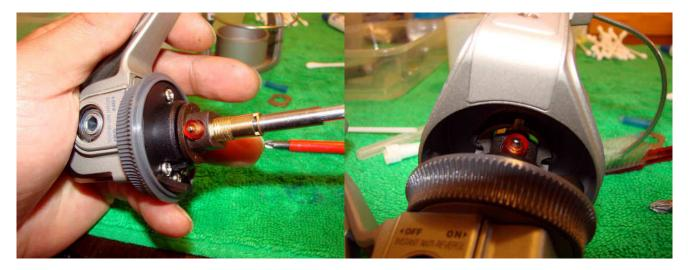
Replace the pawl holder and the pawl assembly. Replace the rotor-note the slot in the rotor that the pawl assembly slots in to.
