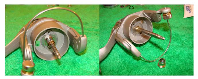
Remove the o-ring and undo the rotor nut.
