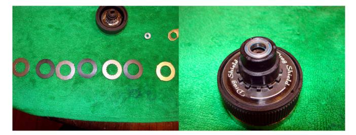
Double check the schematic for your reel. Here the washers are laid out in correct order bottom to top = left to right (metal washer-fibre-keyed metal washer-fibre-metal washer-fibre-keyed metal washer). The keyed metal washers are the ones with tabs on. The fibre washers are the same material as the ones in Ambassadeurs before carbon matrix came out. The drag shield does not look like it will really protect
