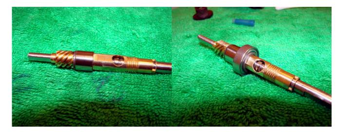
Replace the washer, the sleeve, and then the bearing. Add some grease to the pinion teeth.
