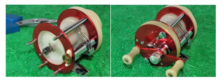
Replace the left side plate and fix in place with the three screws and then replace the spool. Add a drop of oil to the right spool shaft only. Replace the level wind assembly using a drop of oil on either side of the worm gear. As the line carriage sits on the worm gear add a light smear of grease to the entire worm gear-not just to the grooves. Replace the level wind pawl and the line carriage screw.
