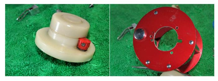
The left side plate has been modified to accept this custom made side plate.
