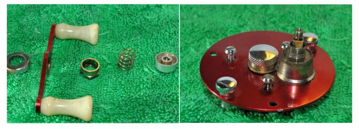
Remove the handle locknut and then the handle and dust shield. Remove the three bridge screws on the side plate.
