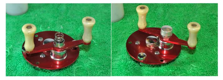
Reattach the dust shield, handle and handle lock nut. Replace the free spool spring and then screw in the free spool button.
