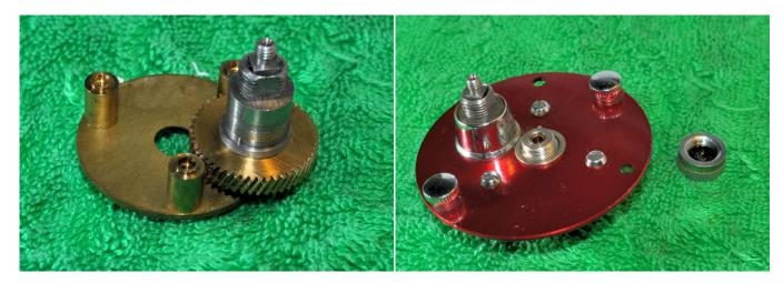
Give everything a thorough clean and then reassemble using oil on the friction surfaces and a light grease on the gear teeth (including the one that sits under the main gear-it drives the worm gear). Replace the bridge gear assembly and fix in place with the three bridge screws. At this stage you can add a drop of oil to the felt in the spool cap. Replace the spool cap on the side plate.
