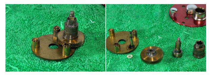
The whole bridge gear assembly can be removed from the other side of the side plate. First remove the handle bearing, then the lock pin retainer, drive gear, and finally the gear shaft bearing (white plastic washer).
