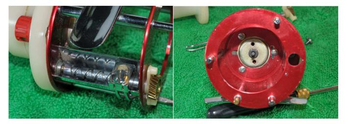
Remove the level wind assembly from the frame by removing the line carriage screw and removing the level wind pawl-the worm gear can then be removed. The left side plate is held in place with three screws. Remove these and lift off the left side plate.
