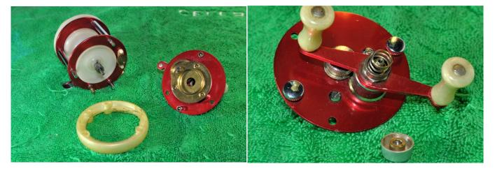
Before looking at the left side plate we'll service the rest of the reel-it's all standard 1750 A, so easy to do. Start by loosening the two thumb nuts on the right side plate. Remove the side plate and head ring (plate spacer). Unscrew the free spool button and remove the free spool spring.
