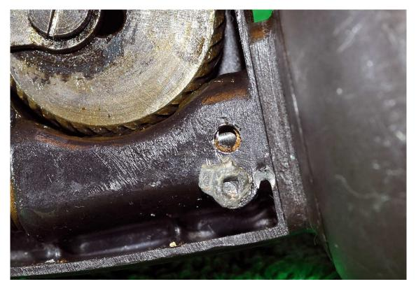
A closer look shows that someone has already tried to drill out a screw and made a bit of a mess. Note the oil port above the mangled screw-use this to lubricate the pinion gear.
