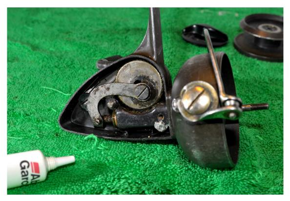
Apply a light coat of grease to the gear teeth and where the oscillating arm contacts the main gear, and oil to the main shaft and oil port on the pinion gear casing. Replace the side plate. The reel works fine and as it is an original display reel it is not worth risking further damage, assuming you could get original ABU parts for it.
